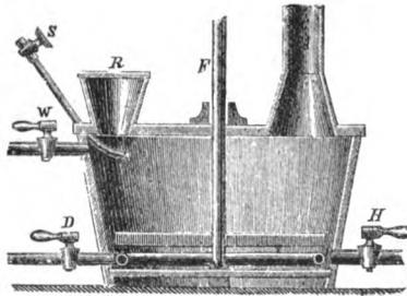
stirrer furnished with two or four paddles, and closed by a well-fitting lid. The stirrer is kept in motion during the entire operation.
