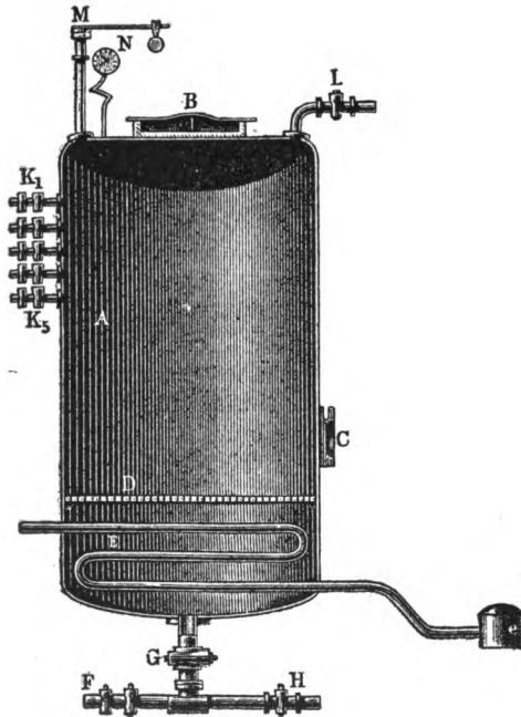
drawing off the fat. The insoluble residues of the glue-stock remain upon the false bottom and are taken out through the man-hole  $C$ .
