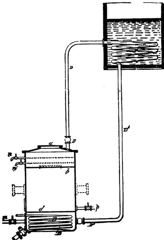
in the vessel below the diaphragm *d*, and the cocks of the outlet-pipes *n n'* are opened.
