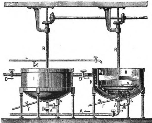
The mode of working with this apparatus is very simple. Water being admitted into the pan through *L*, the glue-stock is introduced and the mass brought to boiling by admitting steam. The finished glue-liquor is from time to time drawn off through the pipe *F* into the settling vessel.
