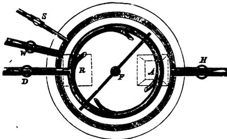
out-let pipes placed in the direction in which the stirrer revolves, lies about 4 inches above the bottom of the tank. *W* is the pipe for the admission of water, *S* the lead pipe connected with the sulphuric acid reservoir, and *A* an outlet of boards for carrying off the vapor evolved from the mass in admitting the sulphuric acid. *R* is a wooden hopper, which serves for the introduction of the bone-ash, and is removed when the tank has been filled, the aperture
