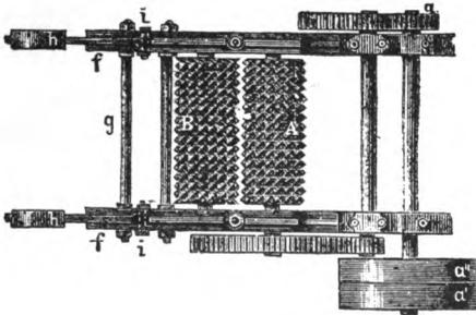
The base of the stamping mill consists of iron plates so arranged as to form steps, the plates lying towards the center of the mill constituting the lowest steps. Every two stamps standing alongside one another rest upon such a step. When the mill is set in motion, the bones reaching the stamping trough from the right and left fall upon the steps, and are crushed by the descending stamps.
