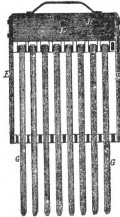
the fused phosphorus and the air is sucked from them by means of the air-pump; the external air-pressure forcing the fused phosphorus into the glass tube.
