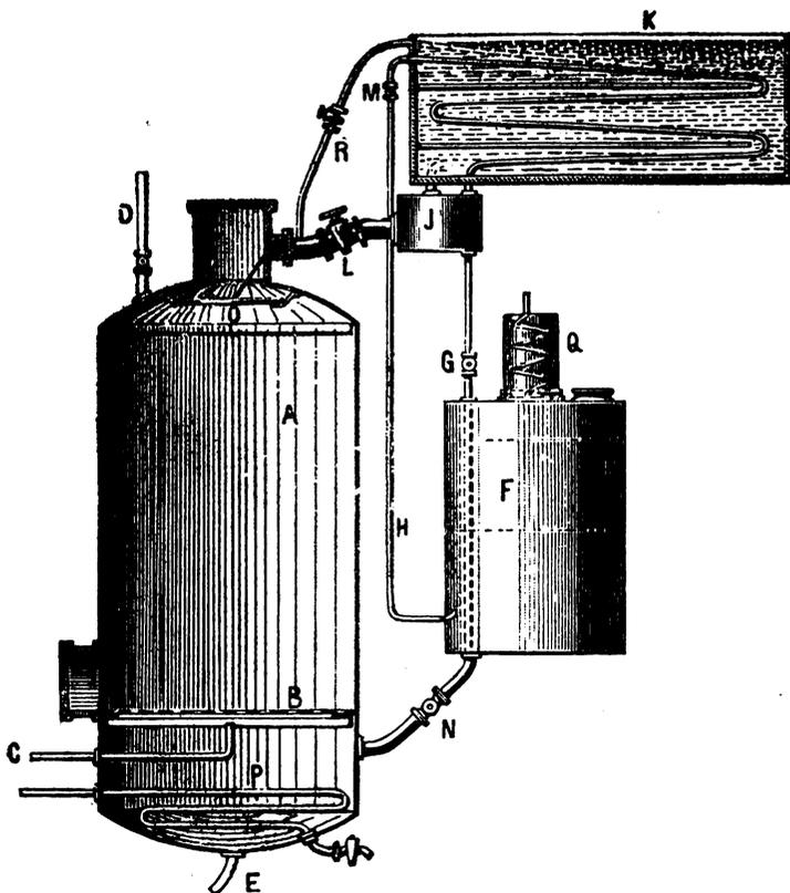
principle, without pressure, using solvent and steam simultaneously. The bones are placed in *A* above the perforated false bottom *B*. *D* is a steam pipe by means of which the bones are steamed as a preliminary, the surplus steam es-
