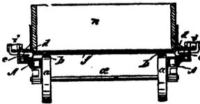
is fitted in boxes on bars, *A*, and near one end thereof it is provided with cranks at its ends, which connect by rods, *i*, to the slides, *d*.
