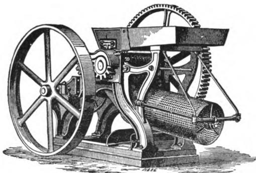
The Crosskill bone mill, Fig. 9, as described by S. Rideal, is intended to be driven by a strap from the fly wheel of a common portable engine. It consists of a pair of strong rollers made of wrought-iron with case-hardened cutters, and a revolving or oscillating riddle for separation of the ground bones as they fall from the cutters; the whole carried by a substantial cast-iron frame. The mill will grind from 6 to 16 hundred-weight per hour with a three to eight horse-power engine.
