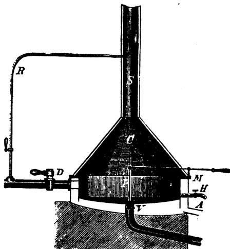
is a sampling cock for taking samples to test the concentration of the liquor.
