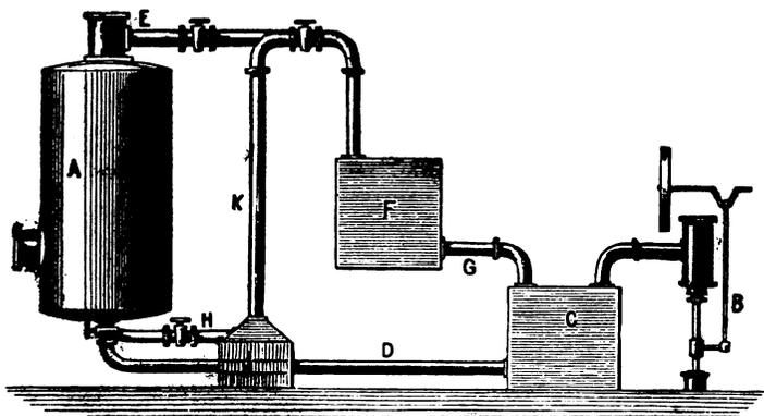
from the reservoir, *C*, through the pipe, *D*, into the cylinder, *A*, and the latter is heated. The vapors formed force the air through the pipe, *E*, into the condenser, *F*, where any vapor which may be carried along is condensed and passes through the pipe, *G*, back into the reservoir, *C*.
