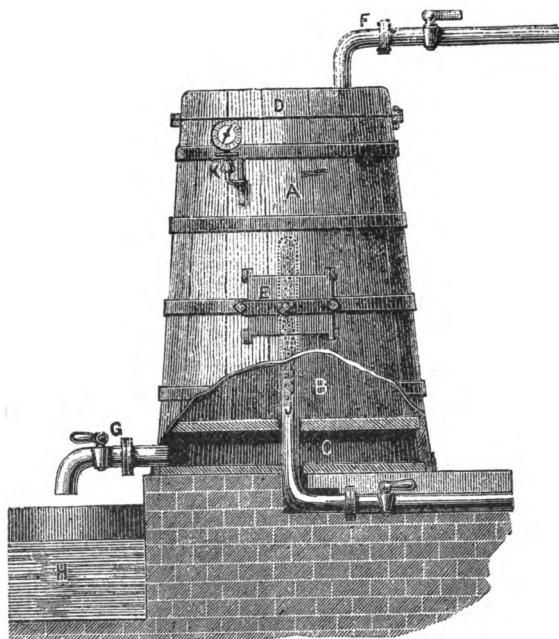
tinued cooking is prevented by drawing off the solution as quickly as formed. The escaping hot vapors may be utilized for drying the glue, softening the raw material, etc., the entire quantity of heat being thus utilized. A further great advantage of this method is that there is less annoyance from badly-smelling vapors than when boiling is done over an open fire. A number of such boilers can be ar-
