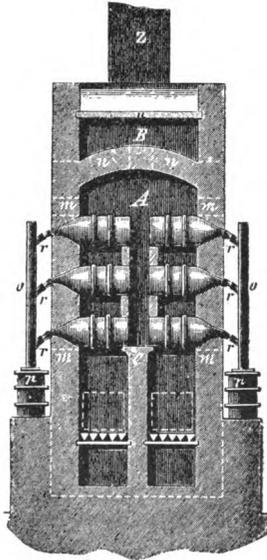
one above the other. Two such furnaces are placed together with their narrow sides, so that the fire-gases of both meet in a common chamber, and are conducted from the latter under the evaporating pans. Four such furnaces may also be arranged in the form of a cross, and their fire-gases conducted into a common chamber. By arranging the furnace, as is most frequently done, for three double rows of seven retorts each, it will hold 42 retorts, a double furnace 84,
