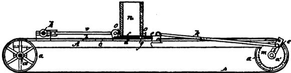
ends with cross-shafts, *a'*, carrying pulleys, *a a*, around which are endless belts, *b b*. *c c* are slide-ways upon the bars, *A*, and *d d* are slides carrying a cross-plate, *e*, and also a plate, *f*, to which plate *e* is attached a knife or cutter, *g*, the cutting edge of which is at the edge of the plate, *f*, and about the same thickness as the slices to be cut. The cross-shaft, *h*,
