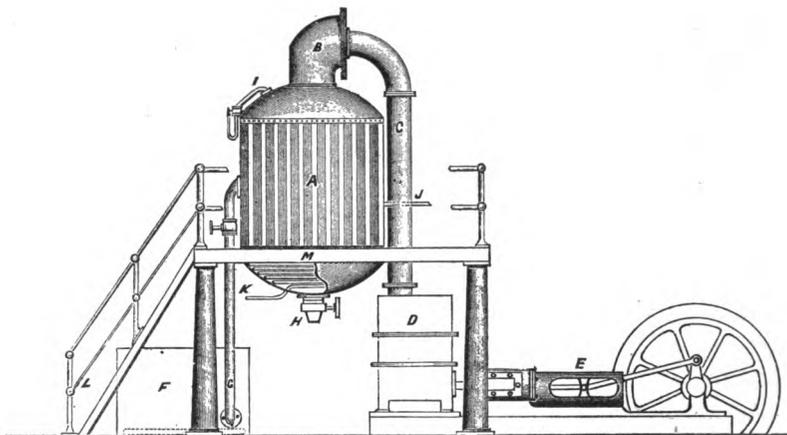
for supplying the coils; *K*, exhaust end of vacuum coils; *L*, iron staircase; *M*, steel floor.
