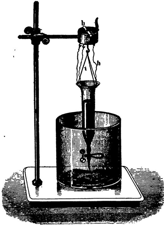
The glue solution is prepared as follows: The glue dried at  $212^{\circ}$  F. is weighed, soaked over night in water, then melted in a small glass in the water-bath, and finally enough water is added so that the solution contains 10 per cent. of dry glue.
