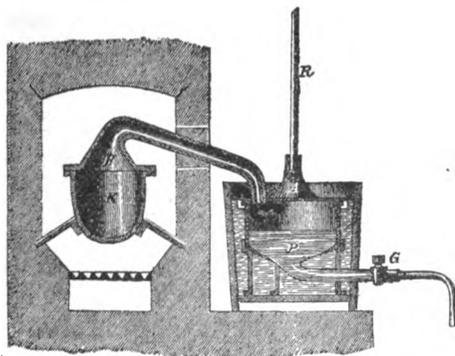
cast-iron retort, *K*, fitted with a cast-iron dome, *H*, the joint being made tight by means of clay and screws. The dome, *A*, tapers to a cone and terminates in a wide glass tube, *R*, bent at a right angle, and having at the mouth a diameter of about  $2\frac{1}{4}$  inches.
