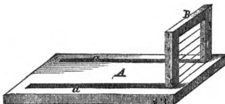
upright portion of the frame are fixed wires at such a distance from each other as required for the thickness of the cakes to be cut.
