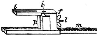
grooves, into which the wires catch to assure the entire cutting through of the block of jelly; *i* is the upper part of the truck, which opens by means of a hinge, and when closed is fastened with the pin, *k*. This upper part of the truck is fastened to the back part of the truck by means of a
