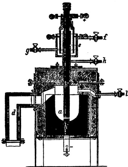
which serves as an insulator of heat, and is closed by a graphite cover, *c*. Through the bottom and the cover of the crucible pass the two electrodes, *k k*, which conduct the current, and between which the voltaic arc is formed. To prevent the upper electrode from becoming too highly heated during the operation, it is constantly cooled by water admitted at *g*, and running off at *f*. Through the pipes *h* and *l* an indifferent gas—as a rule, illuminating
