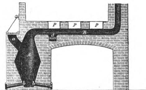
the upper portion of the shaft additional bones may be introduced. This aperture is covered with a heavy iron lid.
