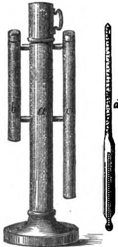
immersed in the tubes filled with glue-liquors to be tested, and temperature as well as percentage can be readily read off.
