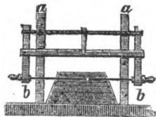
purpose. The vertical bars, *a*, furnished with the wire, *b b*, serve as guides. The sheets thus formed are lifted from the block with the moist blade of a large knife, and laid upon nets.
