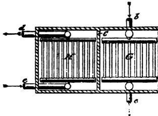
*G*, and having inlet *d*, and outlet *e*. Through this condenser there is kept flowing a refrigerating liquid or brine, which renders the condenser very cold. The continuous current of air from the blower passes over the contents of the cars or trays in the alley and takes up moisture in its passage. After such passage the air is charged with moisture and comes in contact with the coils of the condenser *H*,
