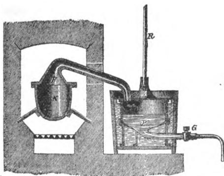
cast-iron retort, *K*, fitted with a cast-iron dome, *H*, the joint being made tight by means of clay and screws. The dome, *A*, tapers to a cone and terminates in a wide glass tube, *R*, bent at a right angle, and having at the mouth a diameter of about  $2\frac{1}{2}$  inches.
