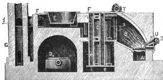
lengthways, and Fig. 49 a horizontal section. The illustrations, however, are given at different heights in order to show plainly the arrangement of the fire-place and the passage of the fire-gases.
