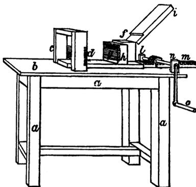
The cutting apparatus patented by M. Devoulx, of Marseilles, is much used in France. The machine stands upon a board or table, upon which are fastened two uprights, far enough apart to allow of the passage of a truck carrying the glue, which is cut into cakes by blades or wires stretched between the uprights.
