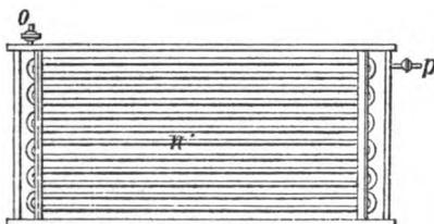
boil the liquid, enters through one of the ends which rises up vertically and is connected with the cock *h'*, Fig. 59. The other end is secured to the inner side of the box, which is perforated for the admittance of the cock *o'*. Upon the steam pipes lies a wooden frame-work with linen nailed upon it, the object of which is to prevent the comminuted bone substance from falling under the pipes. The frame must, of course, fit closely into the box.
