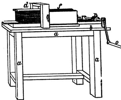
table-plate fastened to the frame, *c* and *d* are the uprights, between which the cutting wires are stretched, and *f* the truck carrying the glue.
