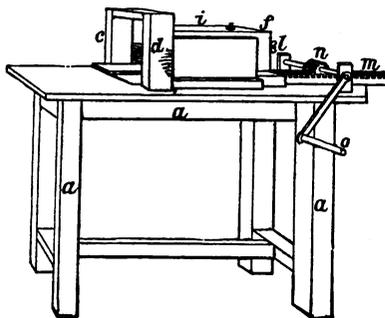
Fig. 19 shows the perspective elevation of the machine with its truck. The upper part is filled up for the reception of the glue to be cut up into cakes. The sides are
