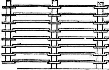
neighborhood of the steam pipes and air flues. As the cakes have to be occasionally turned upside down upon the nets, the latter must be placed at convenient distances, one above the other in the frames.
