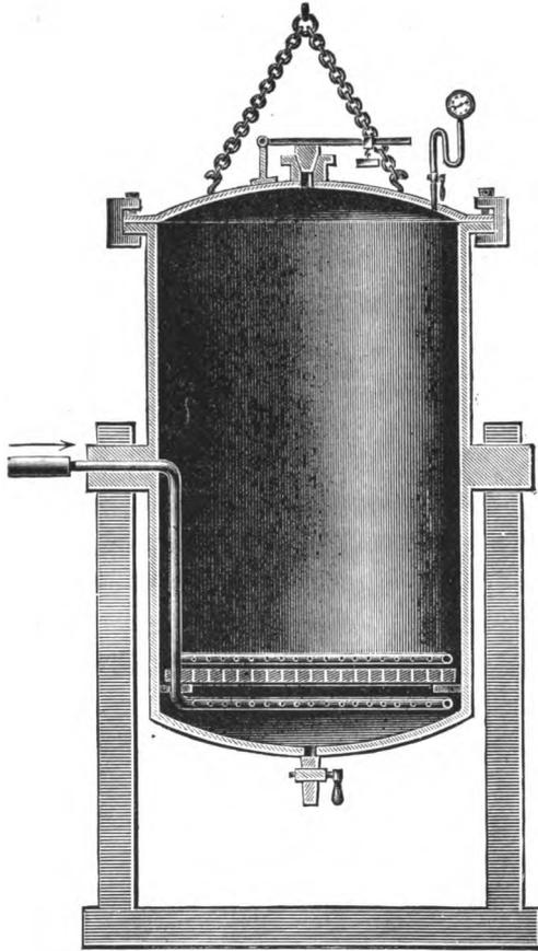
FIG. 4. Boiler for Glue Extraction.
