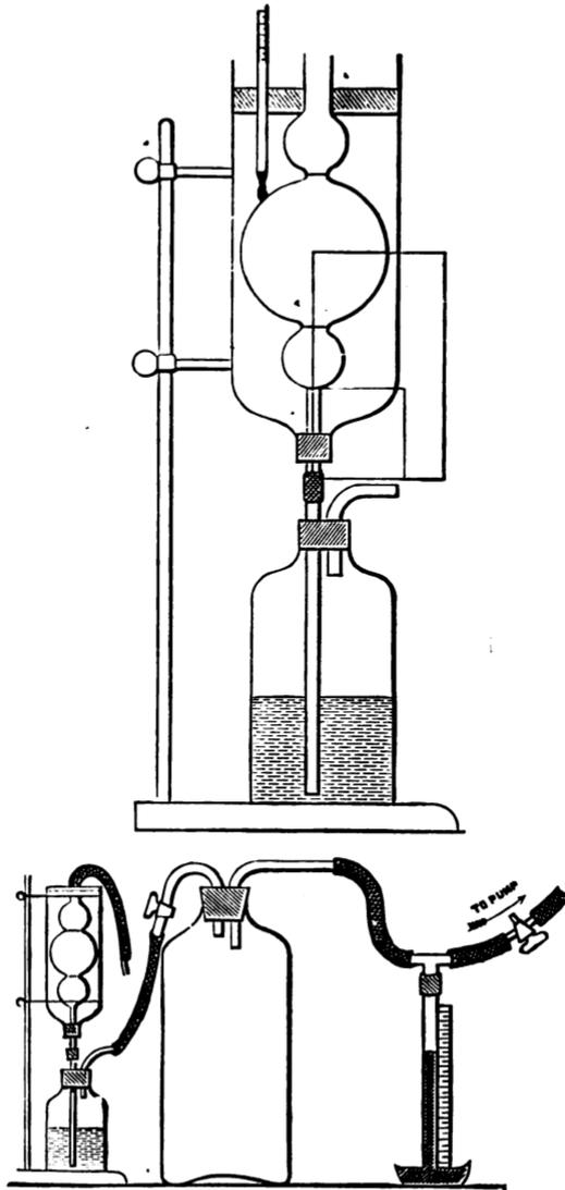
FIG. 14. Rideal-Slotte Viscosimeter.
