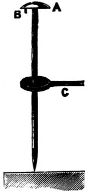
FIG. 12. Kissling's Consistency Apparatus.
