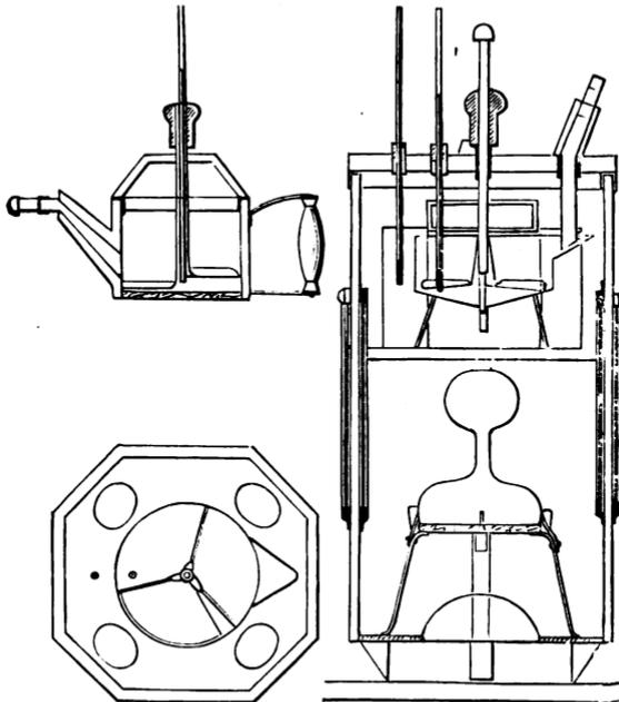
FIG. 13. Engler's Viscosimeter.
