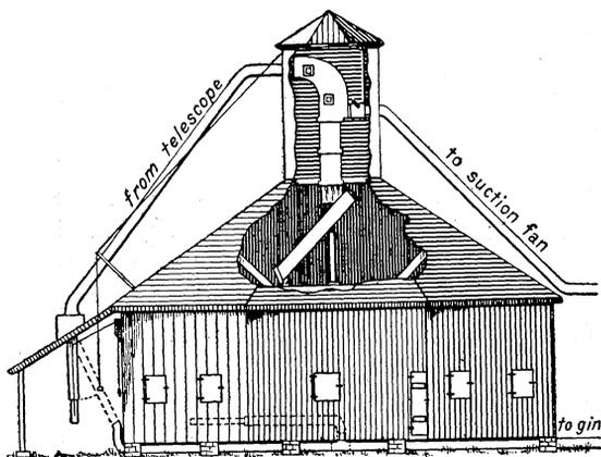
FIGURE 7.—Octagonal seed-cotton house, with pneumatic system for filling and emptying bins.
