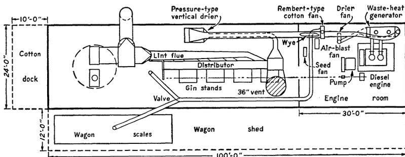
FIGURE 32.—Plan for a one-story modernized cotton-ginning establishment.
