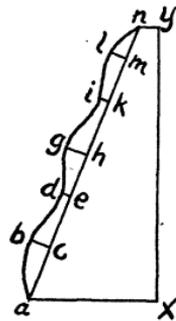
243. The area of a field is not its actual surface, but what its surface would be if graded to a level. When it is necessary to measure distances, the measuring line should be held level. For purposes of finding area, the distance from  $A$  to  $B$  is not the actual distance  $AB$  but the horizontal distance  $A'B,$   $A'$  being vertically above  $A,$  etc.
