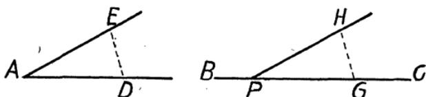
Hold three points of the chain at  $A$ ,  $E$ , and  $D$  pts., at the vertex and on the sides of the given  $\angle$  and an end long enough to reach from  $E$  to  $D$ . Stretch a part of this end from  $E$  to  $D$  and note the length of each side of the  $\triangle ADE$ . Complete the construction and prove it.
