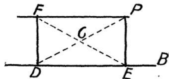
103. Evidently a part of the chain, tape or string may be used instead of the whole. Lines should be determined not by stretching a string but by points, e. g., in the figure of Ex. 152, ascertain whether  $D$ ,  $E$  and  $B$  are exactly in one line by standing at  $D$  and observing whether  $E$  is exactly between  $D$  and  $B$ .
