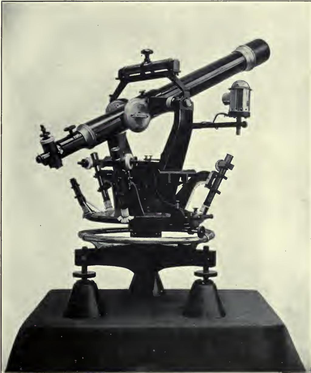
TWELVE-INCH THEODOLITE WITH ELECTRIC LIGHT FOR ILLUMINATING THE CROSS WIRES.
