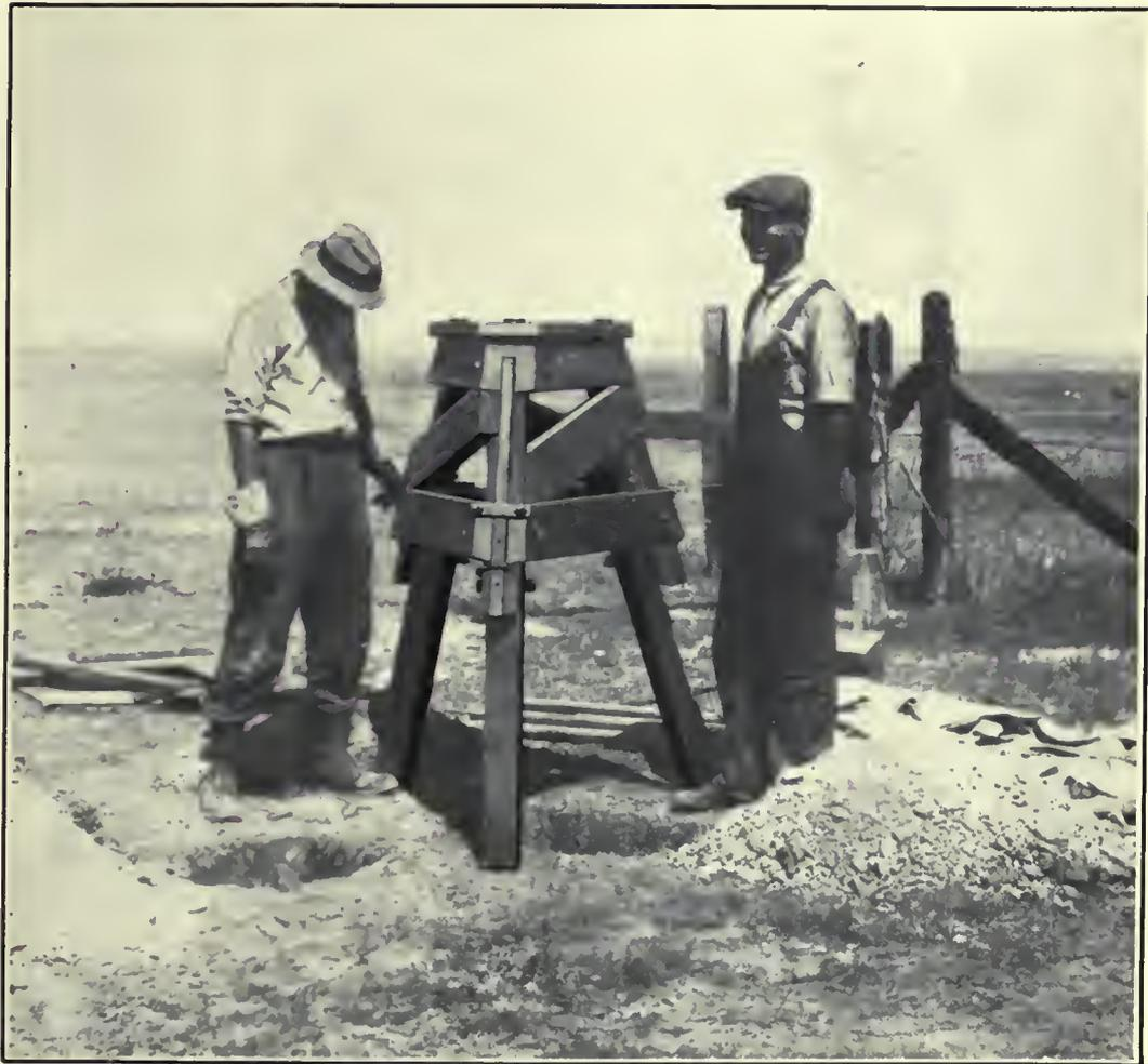
PORTABLE WOODEN SUPPORT WITH ADJUSTABLE LEGS FOR THE ZENITH TELESCOPE.
