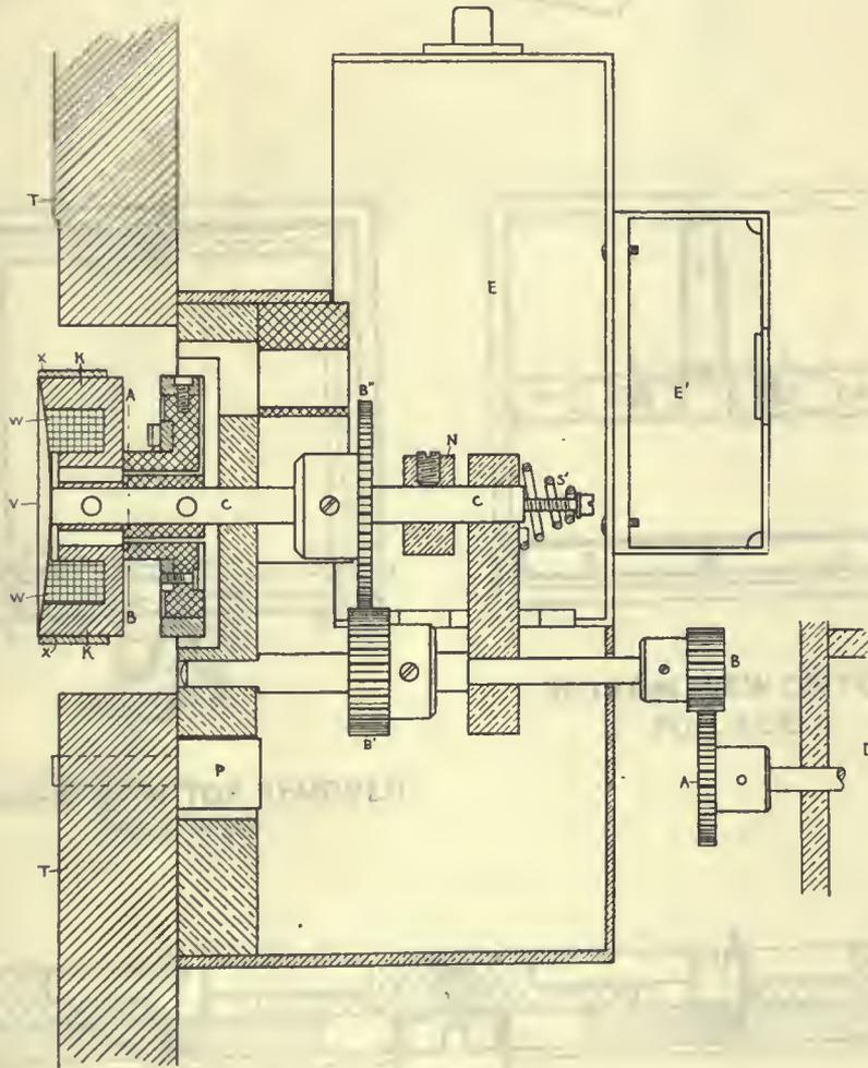
SECTION OF MAGNETIC CLUTCH.
