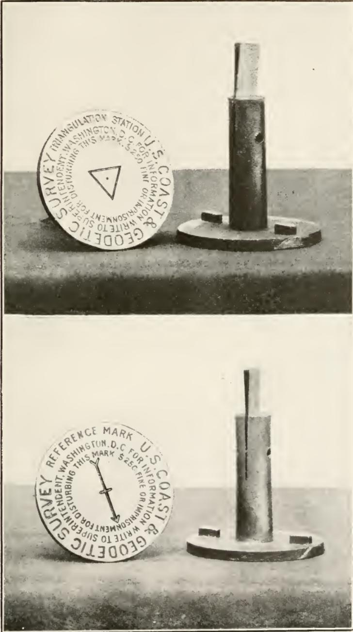
STANDARD STATION AND REFERENCE MARKS USED IN MARKING TRIANGULATION STATIONS.
