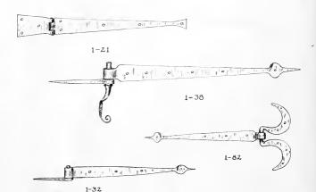
THE Hinge 21 is made with an offset on the short end of about an inch, or whatever the thickness of the material was to which attachment was made. It is called a chest hinge, though the usual chest hinge on American work was a pin hinge, like the cotter pin, two loops of tapered wire or larger iron hooked together.
