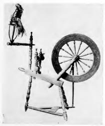
THE distaff on spinning jennies varies from the staff here to a less elaborate sort as seen in the piece below. is prettily turned and very daintily made. This spinning jenny has the well wrought wheel, the spokes of which are neatly turned. Such wheels, of course, are made in segments and are turned with beads, and in some cases are very decorative. especially when made in parti-colors. Owned by the author.
