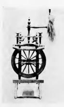
A DOUBLE Spinning Jenny is a rarity. The one here shown is arranged to spin two threads at once. It must have required a spinner of wonderful skill to keep it going. Fingering four part music on the piano would be easy in comparison. The double wheel was the foreshadowing of the machinery that was to follow, so that one spinner could attend an entire battery of jennies. Date: 18th Century. Owner: Mr. L. C. Flynt, of Monson.
