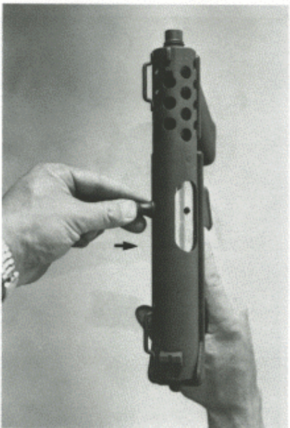
KG-98 open bolt SMG being readied to fire. Step one is to push bolt handle into the safe position.
