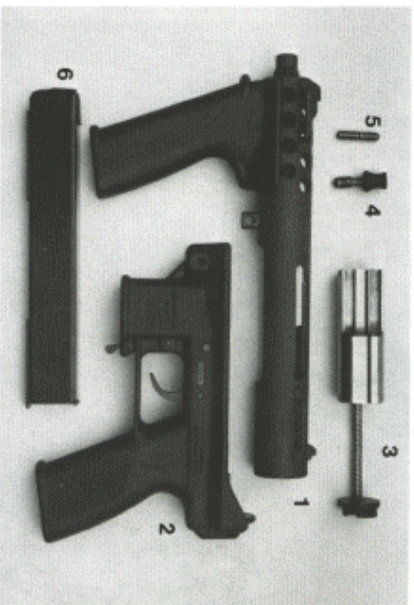
The KG-99 SMG field-stripped into its major components.
