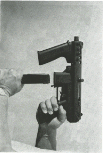
Insert a loaded magazine upward into magazine housing. Push firmly until the magazine latch engages locking block on magazine.
