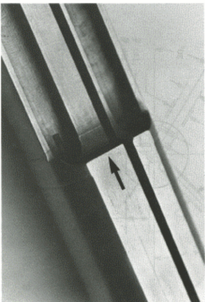
Close up view of front of SMG bolt. Note extractor, fixed firing pin, raised feed lip, recoil spring guide rod hole, and clearance notches for magazine feed lips and ejector.
