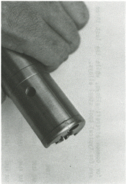
The extractor is held in place by a socket head set screw through the side of the bolt, intersecting the extractor hole.
