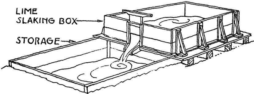
upper box and the lime is let out from time to time by running it through the gate into the lower box to leave room for slaking and to cool off before storage.
