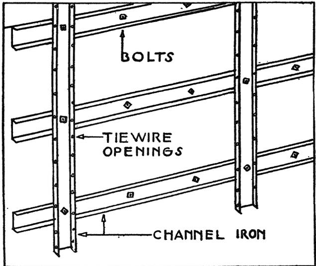
Furring strips are usually made of pine, perfectly dry and straight to avoid warping followed by cracking of the plaster. Large size fresco-murals call for a more extensive furring job. Galvanized channel iron strips are employed, fastened to the wall with EXPANSION BOLTS and screws. Still larger murals would have to be provided with expansion joints hidden in the picture composition.
