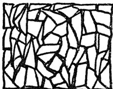
contain a high percentage of quartz, feel sharp and not roll between the fingers. The idea of using sharp sand is to squeeze the mortar tight and this is possible in plastering only when the sand is made up of small wedgelike particles, packed tightly
