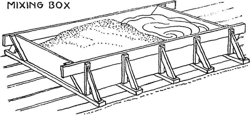
Old boxes, scaled from old lime or mortar and boxes that were used for gypsum plaster should not be used for fresco mortar. They can never be so completely cleaned that the danger of efflorescence will be eliminated.
