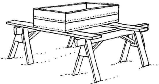
A couple of HORSES, two SCREENS of different mesh, a large DRYING PLATFORM raised a foot from the ground and a WATERHOSE comprise the sand washing equipment. The screens are fitted one on top of the other and are of the same size. The lower screen is made of 28-34 mesh, reinforced with galvanized metal lath underneath, and the upper screen is equipped with window fly screen or 16 per inch mesh.
