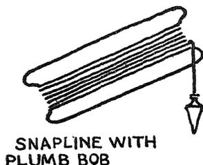
A small plumb bob tied to the loose end of the line will serve instead of the waterlevel on vertical lines. "Chalking" the line is done by rubbing it with broken pieces of charcoal sticks. Use of colors on the snaplines and in the pounce bag might result in serious smudging of the intonaco. Before snapping the line to transfer the charcoal, the line is lifted and let down gently again to loosen it from paper creases and rough mortar surfaces.
