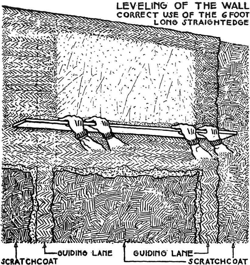
In a corner of the wall, a vertical lane of mortar, the width of the trowel, is spread on and five feet away from this lane
