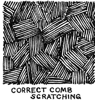
Over a well wetted down brick wall an ordinary sand-lime coat, mixed from 1 part lime and  $2\frac{1}{2}$  to 3 parts of sand is laid on to a thickness of about  $\frac{1}{4}$ ". This coating is scratched with the comb and before it is left to set it is given a fine spray of water.
