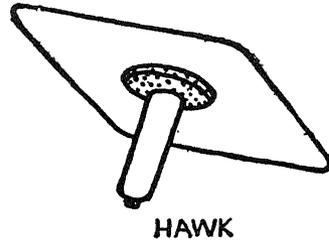
The HAWK is the plasterer's palette, a square piece of aluminum with a hardwood handle in the middle cushioned with a sponge rubber ring around the handle underneath the square.
