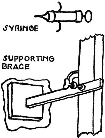
erly compounded CEMENTING AGENT through pinhole openings in the faulty places with a SYRINGE, a special kind of small hand sprayer. The loose plaster is pressed back slightly and a
