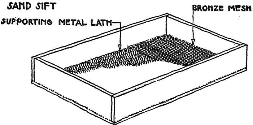
A level bucket of sand is poured into the sift and shaken through. For every bucket of sand sifted into the box, a grease pencil stroke is made on the outside of the box thus keeping close count of the intended mixture. Always measure in buckets for shovelful are too irregular. Extra buckets are counted in for sifting waste.
