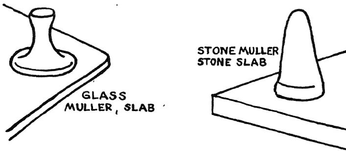
STONE MULLER may be procured from a lithographic supply house as well as a stone slab for grinding colors. Heavy slabs and mullers do the work twice as fast as smaller ones. A chemist's MORTAR AND PESTEL can be used with equal success. Test rubbing on the nail will tell when the pigment is ground to the desired fineness.
