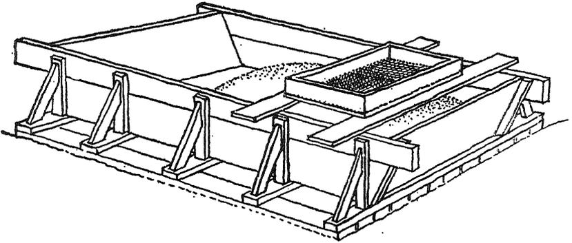
mesh window fly screen is used and for the browncoat and the sand finish, 18 or 20 mesh and for the intonaco a 32-34 mesh screen. The top sift in sandwashing, 18 mesh and the lower is of 29-30.
