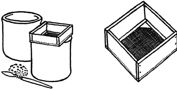
The equipment for making the MILK OF LIME consists of two one gallon stone crocks and a 56 mesh brass sieve of the same diameter as the top of the crocks. A long bristle brush is used to push the lime through the sieve and for cleaning purposes, a small sponge and a bucket of water.
