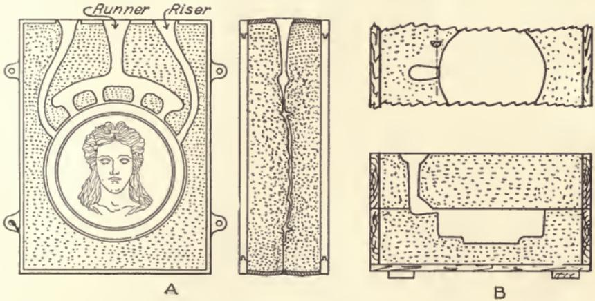
Fig. 128. (A) Mold for Thin Plate.—(B) Mold for Heavy Plate.
