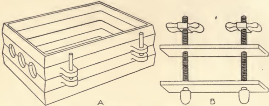
Fig. 125. (A) Flask for Brass.—(B) Screw Clamp.
