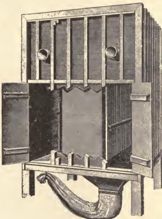
Fig. 112. Dust Collector for Tumbling Barrel.
