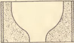
Fig. 123. Runner Box for Steel Mold.
