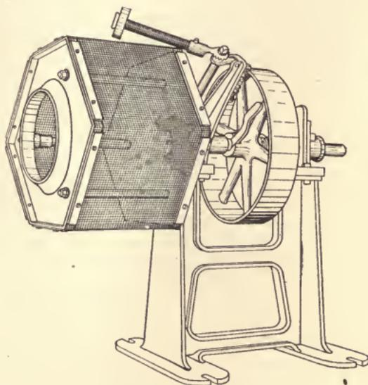
Fig. 107. Rotary Sieve.
