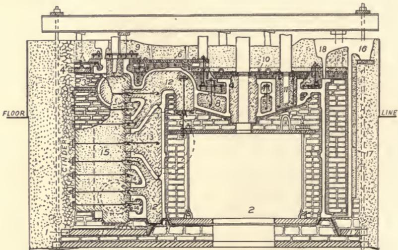
Fig. 97. Loam Mold for Marine Cylinder.
