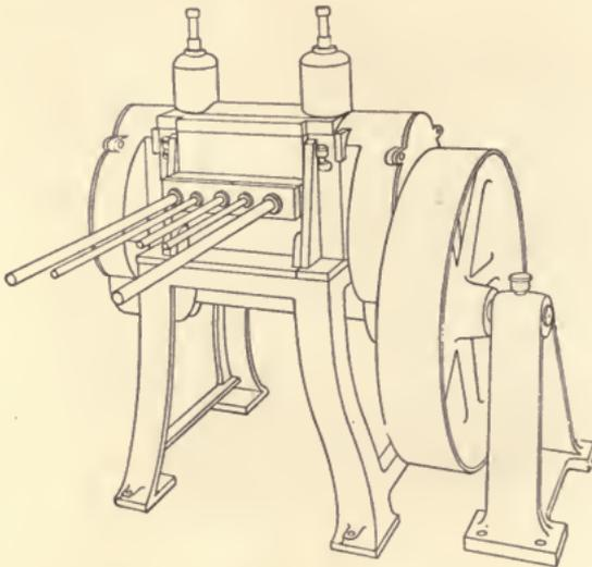
Fig. 115. Core Rod Straighteners.
