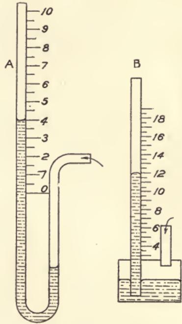
Fig. 101. Wind Gauges.
