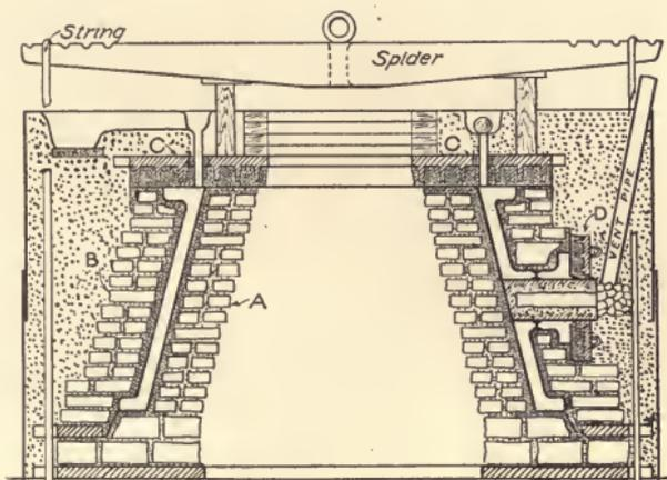
Fig. 96. Complete Typical Loam Mold.
