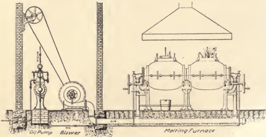
Fig. 136. Oil Furnace—General Elevation.
