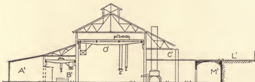
Fig. 138. Typical Elevation of Foundry.
