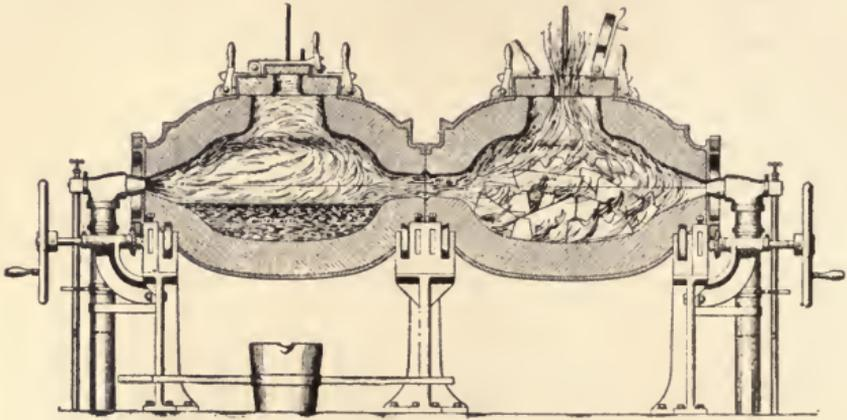
Fig. 135. Section Through Oil Furnace.
