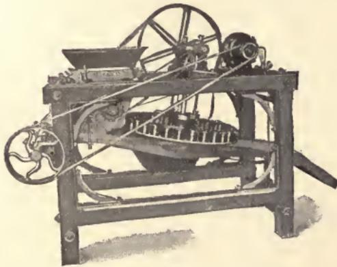
Fig. 132. Magnetic Separator.
