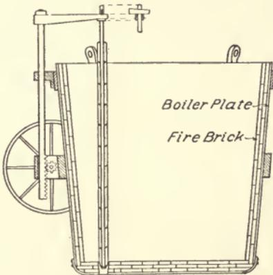
Fig. 122. Section Through Steel Ladle.
