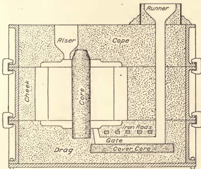
Fig. 119. Section Through Steel Mold.
