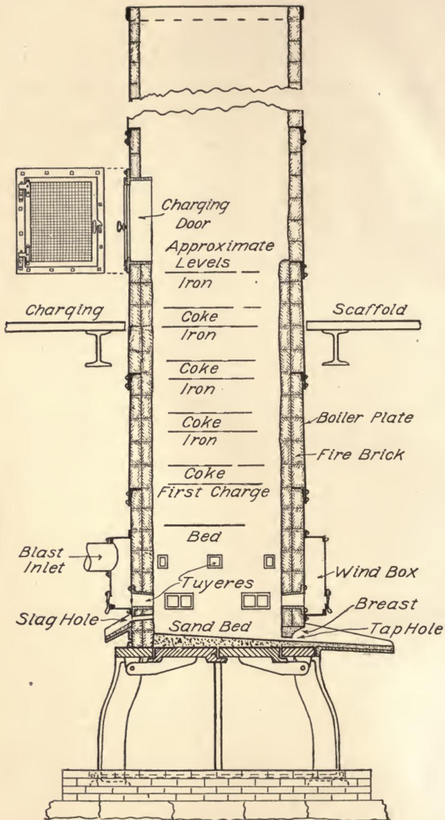
Fig. 98. Section Through Cupola Furnace.
