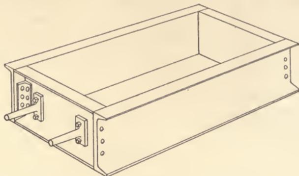
Fig. 118. Small Flask for Steel Molds.
