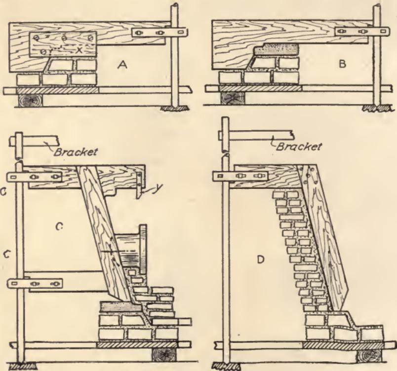
Fig. 95. Steps in Sweeping up Type Mold.
