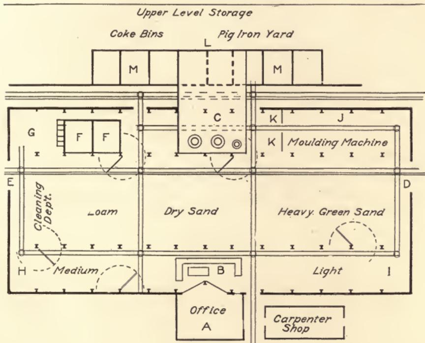
Fig. 137. Typical Plan of Foundry.
