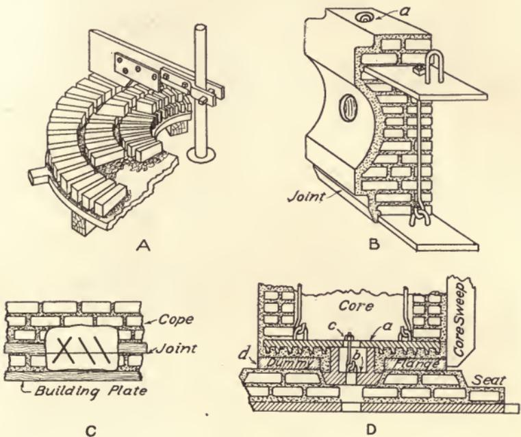
Fig. 94. Laying up Loam Work.
