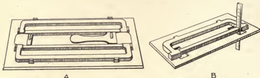
Fig. 141. (A) Keep's Test Bar Pattern.—(B) Measuring Shrinkage.
