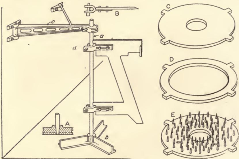
Fig. 93. Rig for Loam Work.
