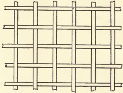
Fig. 121. How Brick is Set in Regenerator.
