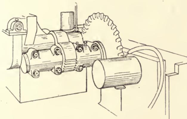
Fig. 124. Cutting off Riser.
