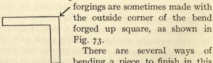
forgings are sometimes made with the outside corner of the bend forged up square, as shown in Fig. 73.
