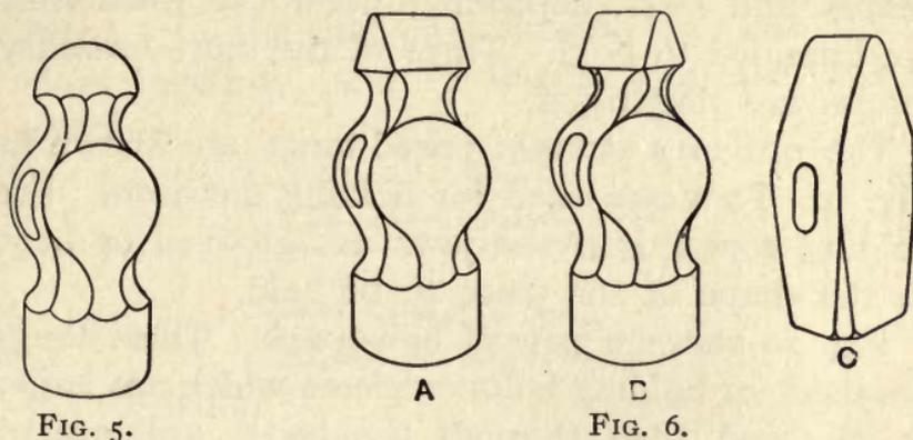
in Fig. 6. *A* is a straight-pene; *B*, a cross-pene; and *C*, a riveting-hammer.
