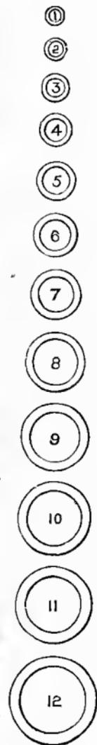
Fig. 163.—Brass Rod Rings. Nos. 1 to 12.
