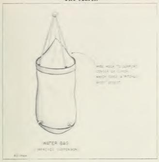
Figure 11.—Water sterilizing bags may be improved by supporting the bag cover in the center by means of a wire to the apex of the tripod support. This gives a pitched roof effect, allows rain water to run off the top, prevents sagging and contamination.
