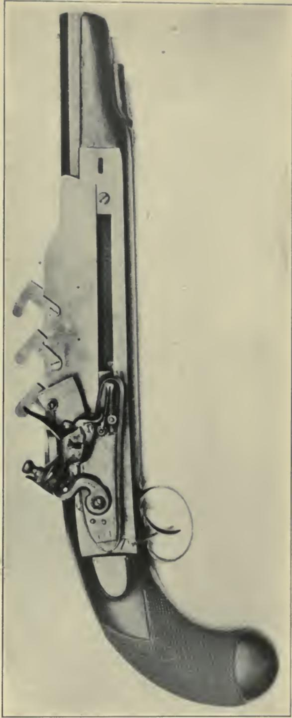
PLATE No. 28. — Four-shot Superposed Single Barrel Pistol
