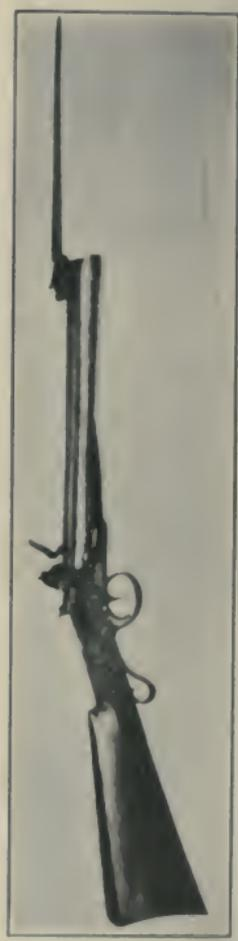
half round. It has "Fly or Die" engraved near the muzzle, and engraved brass mountings. The silver name-plate is engraved "I. Pritt & Co." The lock is case-hardened in colors. The wood is fancy walnut. The whole length is 29 inches, bayonet  $11\frac{1}{2}$  inches extra, weight  $6\frac{1}{2}$  pounds, muzzle diameter  $1\frac{5}{8}$  inches.
