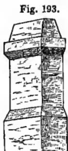
wind, at the same time that the surface is smaller on which the wind can strike the current, as shown in *Fig. 192*. A chimney of this character may be very easily made by contracting the tiers of brick, thus giving to it an ornamental appearance, as seen in *Fig. 193*.\*
