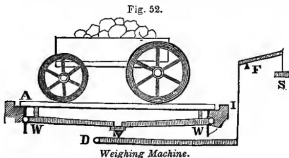
cattle, wagons loaded with hay, and other heavy articles. The wagon rests on the platform A (*Fig. 52*, p. 71), and this platform rests on two levers at W, W, which presses their other ends both on a central point, and this again bears on the lever D, the other end of which is connected by means of an upright rod with the steelyard at F.
