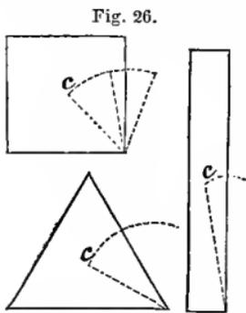
26) is less easily thrown over than the tall and narrow block of equal weight, because, in turning the square block over its lower edge, the centre of gravity must be lifted up considerably in the curve shown by the dotted line *c* ; but with a tall, narrow block, this curve being almost on a level, very little lifting is required. Hence the reason that a high load on a wagon is so much more easily overturned than a low one.
