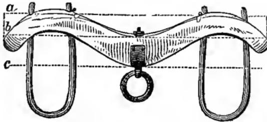
that is faulty in this respect, by having been cut from a piece of timber as wide as the dotted lines *a c*, and being thus weakened, it requires to be correspondingly large. *Fig. 84* is equally strong, much lighter, and is
