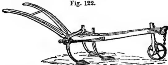
useful for paring, or cutting the roots of weeds; and formed like the mould-board of a plow, they are sometimes used for throwing the mellow earth toward the row, or, when reversed, from it.
