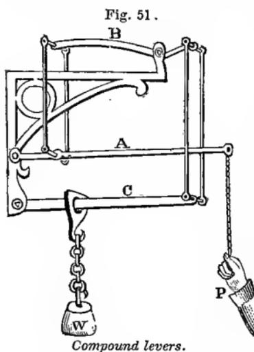
the lever *A*, exerting a force on the lever *B* five times as great as the power. *B* acts on the lever *C* with a force increased three times, and this, again, on the weight, *W*, with a four-fold force. Multiplying 5, 3, and 4 together, the product is 60; hence a force of one pound at *P* will support 60 pounds at *W*. By graduating (or marking into notches) the lever *C*, so that the distance is measured as the weight
