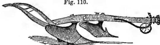
boards on one beam. The forward or small one pares off the surface or sod, and throws it into the previous furrow, usually to a depth of three to five inches. The larger one follows closely, lifting the under-soil upon the top, and in sward land completely burying the sod with the mellow earth from below. This is the best implement for trench-plowing yet introduced into practice, and with double the ordinary amount of team, will cut to a depth of nine to twelve inches.
