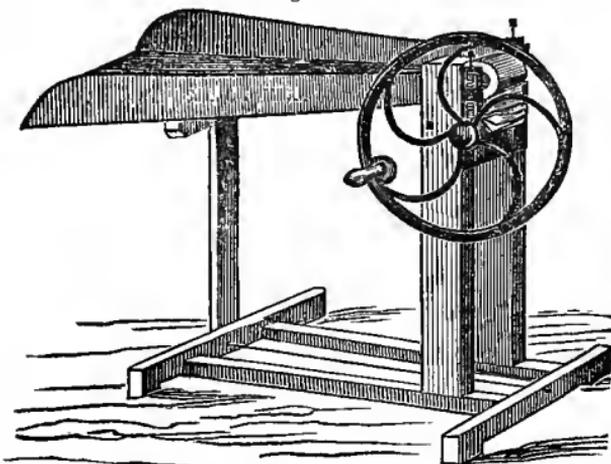
fect in this machine is its inability to cut shorter than one inch in length, which is not sufficient for corn-stalks and other coarse fodder.
