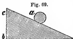
A body, in rolling freely down an inclined plane, acquires the same velocity that it would attain if dropped perpendicularly from a height equal to the perpendicular height of the plane. Thus, if an inclined plane on a plank road be 100 yards long and 16 feet high, a freely running wagon, left to descend of its own accord, will move 32 feet per second by the time it reaches the bottom, that being the velocity of a stone falling 16 feet. Or, a rail-car on an inclined plane 145 feet
