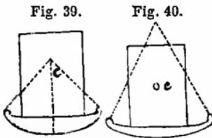
greater than the distance to the middle, *c*, as in *Fig. 39*, the motion will be slow and gentle; but if this difference be greater, as in *Fig. 40*, it will be rapid. When the centre is high, the rockers must have less curvature than where it is low and near the floor. If the centre of gravity be nearer the ends than to the middle, the chair will immediately be overturned. This principle should be well understood in the construction of all instruments which move by rocking.
