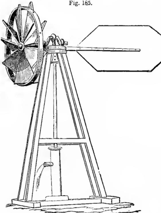
per circle moves around with the wheel and vane on the fixed lower circle, to which it is strongly secured so as to admit of turning freely. In other respects it is similar to the preceding.
