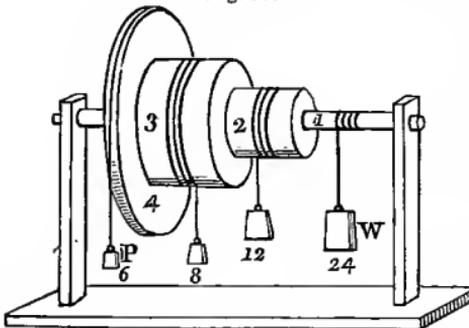
*Wheel and axle, showing the heavier weight for less motion.*
