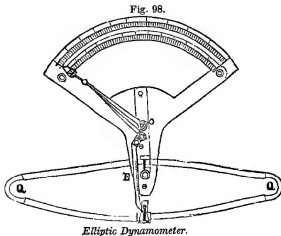
where the ends of the oval spring, *Q Q*, are attached to the plow and draught. The harder the force exerted by the team, the closer together will the sides of this spring be brought, causing the rod, *E*, to press against the index or pointer, and showing the precise degree of force on the circular scale.
