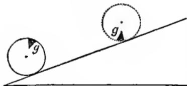
light cylinder of cork or pasteboard contains a concealed piece of lead,  $g$  (*Figure 18*). The lead, being heavier than the rest, will cause the cylinder to roll up an inclined plane, when placed as shown by the
