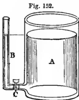
square inch of the bottom, or upon every square inch of the sides fourteen inches below the surface. If the tube, C, be an inch square, the water will be driven into it with a force of half a pound, and will press with that force against the one-inch surface of the stop-cock, C. If the tube, B, be now filled to an equal height, the same force will be exerted against the other side. To prove this, let the stop-cock be opened, when the two columns of water will remain at an exact level.
