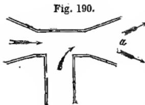
regarded as incurable. *Fig. 190* is intended to show the mode of its operation, the wind, as shown by the arrows, being deflected for a considerable distance on the lee side, so as to form a vacancy at *a*, which the wind from the other end and from the chimney both rush in to supply. Being fixed on without turning in the chimney, it is both simpler and less noisy than any caps furnished with a vane.
