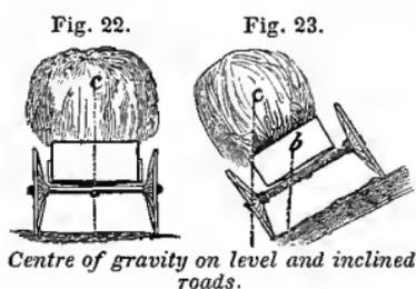
in *Fig. 22*, by the dotted line,  $c$  being the centre. But if it pass a steep side-hill road, throwing this line outside the wheels, as in *Fig. 23*, it must be instantly overturned. If, however,
