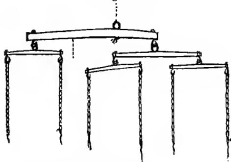
as much greater than the other as four is to three, then the weaker horse should be attached to the arm of the whipple-tree made as much longer than the other arm as four is to three.
