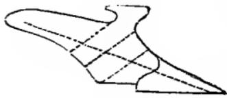
the face at right angles to the line of motion, as shown by the dotted lines in *Fig. 104*, the mould-board will be so far right; but if the straight edge must be placed in other positions, as in *Fig. 105*, it is defective in form. A mould-board may be much modified,
