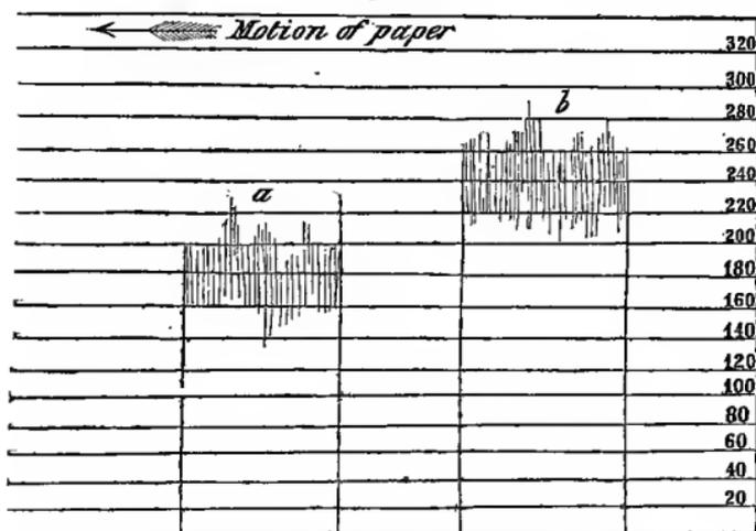
The markings of the Self-recording Dynamometer.
