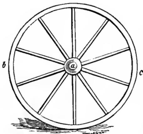
leverage of the wheel on the friction at the axis ; and the smaller the axle, the greater is this leverage ; for, if the axle, *a* (*Figure 88*), be six inches in circumference, and the wheel, *b c*, be ten feet in circumference, then the outer part of the wheel will move
