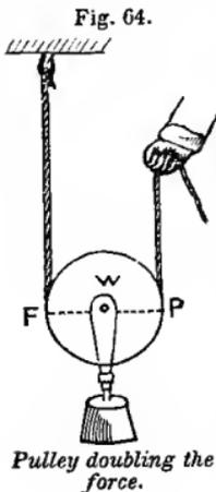
The wheel is called a *sheave*; the term *pulley* is applied to the block and sheave; and a combination of sheaves, blocks, and ropes is called a *tackle*.
