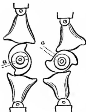
*Dick's Cheese-press* (*Fig. 145*, on the following page) operates on a similar principle. *Figure 146* shows the structure of its working part, the dotted lines indicating the position of the lever, which is inserted into a roller or axle, and, by turning, drives the movable iron blocks asunder, and raises the cheese against the broad screw-head above, as shown in *Fig. 145*.
