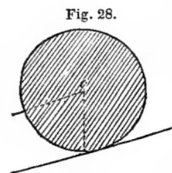
Wheel-carriages owe their comparative ease of draught to the fact that the centre of gravity in the load is moved forward by the rolling of the wheels, on a level, or parallel with the surface of the road, just in the same way that the round ball rolls so easily. Each
