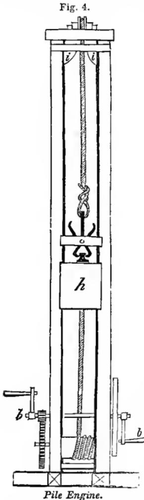
great size are forced into the mud of swamps and river bottoms, where other means would fail. When a steam-engine is used for lifting the ram, the work is more rapidly performed.
