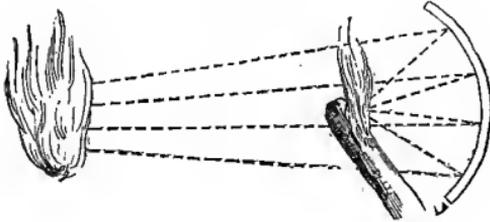
The reflection of radiated heat may be beautifully exhibited by using two such concave tin mirrors. Place them on a long table several feet apart, and ascertain the focus of each by means of the light of a candle. Then place in the focus of one a red-hot iron ball, or a small chafing-dish of burning charcoal. In the focus of the other place the wick of a candle with a small shaving of phosphorus in it. The heat will be reflected, as shown by the dotted lines (*Fig. 206*),
