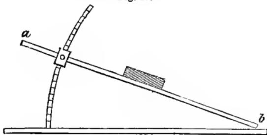
desired height by means of the arc of a circle and a screw. Lay a flat surface of the substance we wish to examine upon this inclined plane, and another small-
