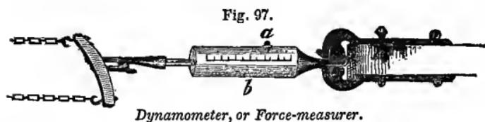
spring balance, with one hook attached to the plow and the other to the whipple-tree. The amount of force required to draw the plow is accurately measured on the scale by the index or pointer, *a*.
