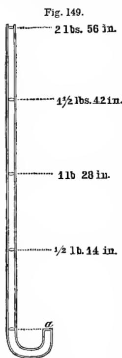
pounds, twenty - three feet ; twenty pounds, forty-six feet, and so on. Now, as the side pressure is the same as the pressure downward for the same head of water, the same column will, of course, exert an equal pressure on a square inch of the *side* of the tube. Or, if the tube be bent, as shown in the annexed figure (*Fig. 149*), the pressure upward on the end of the tube, at *a*, will be the same for the various heights.
