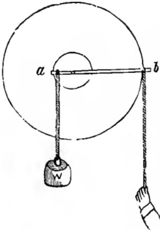
wheel be attached, so that this cord too may wind upon the larger wheel. These two wheels (fastened together so as to form one), as they are made to revolve on their axis, will now constitute, in a manner, a succession of levers, acting through an indefinite distance according to the length of the cords. The levers here successively acting are of the "first kind," and the axis of
