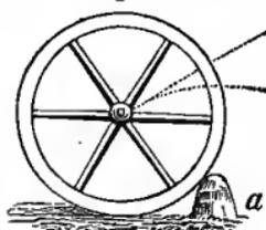
following explanation: Let the obstruction, *a*, in the annexed figure (*Fig. 91*), represent the friction the wheel constantly meets with in rolling over a common road. To overcome this friction, the wheel must
