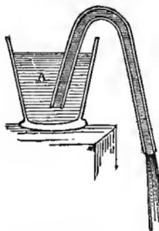
water, and then placed with the shorter arm in the vessel of water, A, the weight of the column of water in the longer arm, which is outside, will overbalance the weight of the other column, and will therefore run out in a stream. This tends to cause a vacuum in the tube, which is instantly filled by the water rushing up the shorter arm, being driven up by the pressure of the atmosphere. A stream will consequently continue running through the syphon until the vessel is drained.
