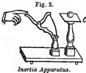
little instrument called the *inertia apparatus* (Fig. 2). A marble or small ball is placed on a card (*c*) resting on a concave stand. A spring snap is then made to strike the card, throwing it to a distance, but leaving the
