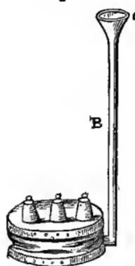
(*Fig. 155*), which consists of two round pieces of board, connected by a narrow strip of strong leather; into it is inserted a long narrow tube, B, with a small funnel, *e*, at the top. When water is poured into this tube, it will raise a weight as much greater than the weight of the water in the tube as the surface of the upper board exceeds the cross-section of the tube. Thus, if a pound of water fills
