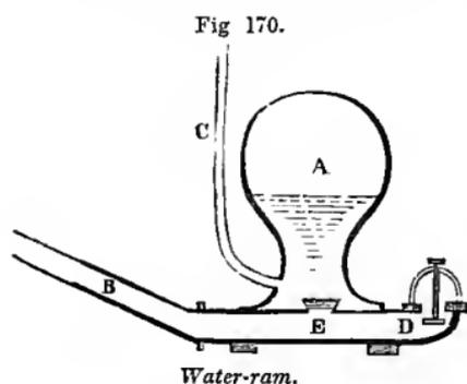
stream. Its principal parts are the reservoir or air-chamber, A (*Fig. 170*), the supply-pipe, B, and the discharge pipe, C. The running stream rushes down the supply-pipe, B, and, striking the waste
