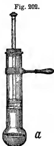
The *Steam-engine* owes its power to the enormous expansion of water at the moment it is converted into steam, which is about 1600 times its bulk when in the form of water. The principle on which the steam-engine acts may be understood by a very simple instrument represented in *Fig. 202*. A glass tube with a small bulb is furnished with a solid air-tight piston, capable of working up and down. The water in the bulb, *a*, is heated with a spirit-lamp or sand-bath; the rising
