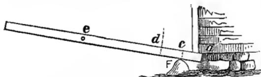
twelve feet long, *a b*, Fig. 49, be used as a lever to lift the corner of a building, then
