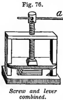
for example, a screw be ten inches in circumference, and its threads half an inch apart, it exerts a force twenty times as great as the moving power. If it be moved by a lever twenty times as long as the diameter of the screw, here is another increase of twenty times in force. Multiplying
