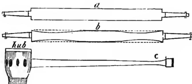
Sometimes several forces act at once on different parts. For example, the spokes of wagon-wheels require strength at the hub for stiffening the wheel; they must be strong in the middle to prevent bending, and large enough at the outer ends, where they are soonest weakened by decay. Hence there should be nearly a uniform taper, slightly larger at the middle, and with an enlargement at the outer end, as *c* (*Fig. 86*).
