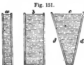
the water being equally high in both, the pressure on the whole bottom of  $b$  will be nine times as great as on the bottom of  $a$ ; or any one inch of the bottom of  $b$  will receive as great a pressure as the bottom of  $a$ . Again, if the vessel  $c$ , broad at the top, be narrowed to only an inch in diameter at bottom, the pressure upon that inch will still be the same, most of the weight of its contents resting against the sides,  $d d$ .
