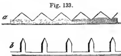
made at the present day consists of a serrated blade, as shown at *a* (*Fig. 133*), which passes
