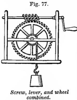
When the screw is combined with the wheel and axle (*Figure 77*), it is capable of exerting great power, which may be readily calculated by multiplying the power of the screw and its lever into the power of the
