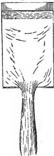
the stream will be considerably contracted (*Fig. 158*). If a short tube be inserted into the hole (the head being the same), this crossing of particles will be partly prevented, and the liquid will flow more rapidly. The greatest effect is produced
