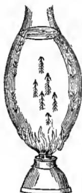
comes warm and expands; it immediately rises to the surface, and colder portions sink down and take its place, to ascend in their turn. In this way, a constant circulation is kept up among the particles. These rising and descending currents are shown by the arrows in *Fig. 200*. This result may be easily shown by filling a flask with water into which a quantity of sawdust from some green hard wood has been thrown, which is about as heavy as water.
