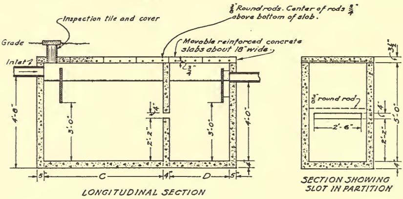
FIG. 25.—SUGGESTED DESIGN FOR A TWO-CHAMBER SEPTIC TANK
