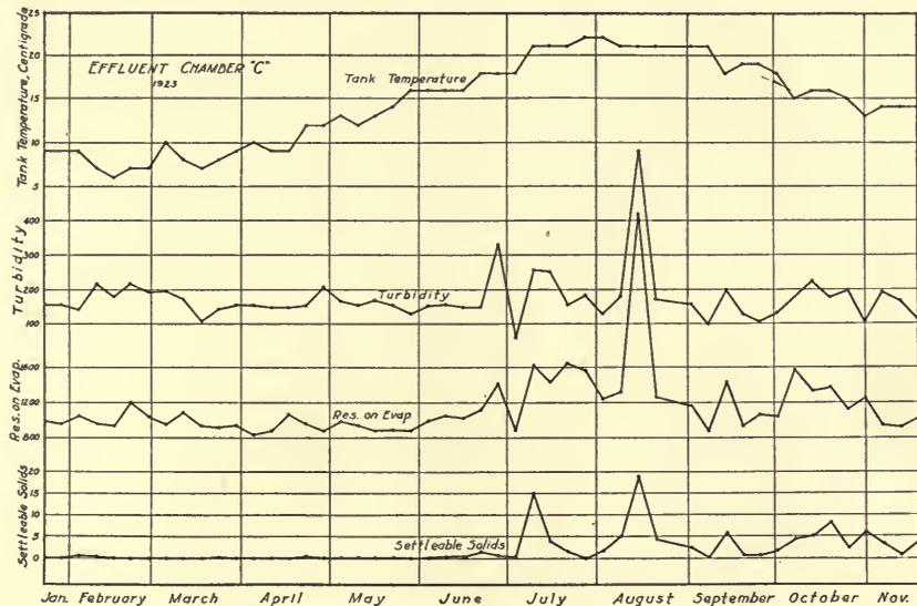
FIG. 13.—VARIATIONS IN EFFLUENT FROM CHAMBER C: CITY SEWAGE
