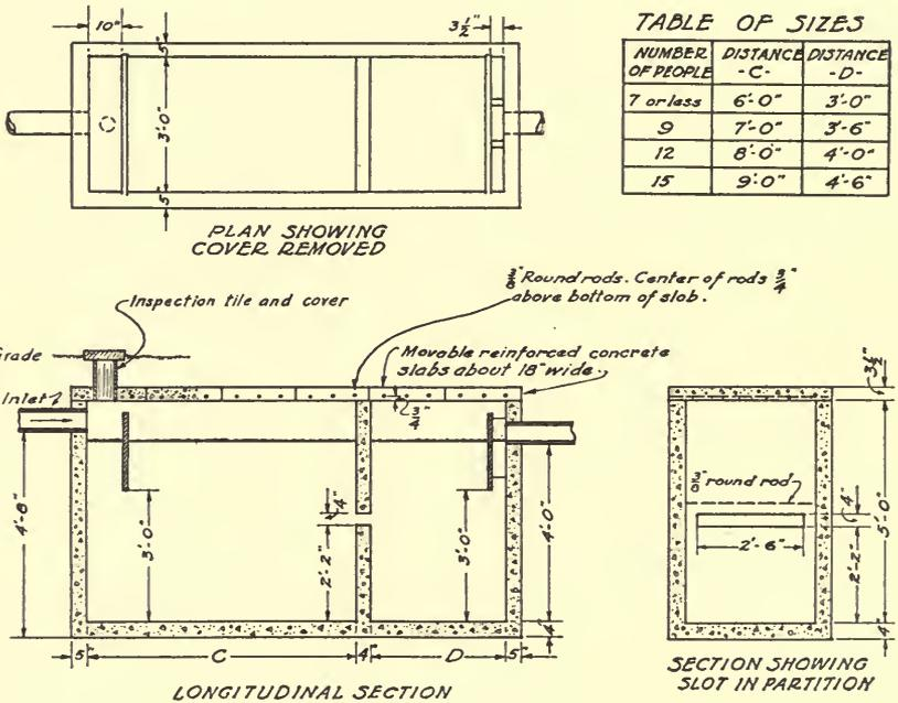
FIG. 25.—SUGGESTED DESIGN FOR A TWO-CHAMBER SEPTIC TANK
