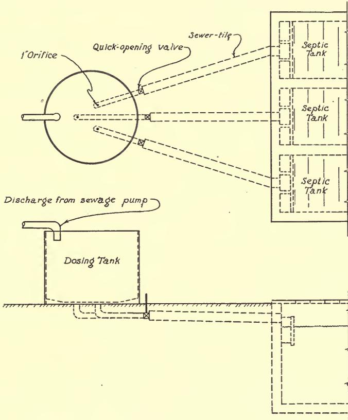
FIG. 5.—PLAN AND ELEVATION OF THE DOSING APPARATUS
