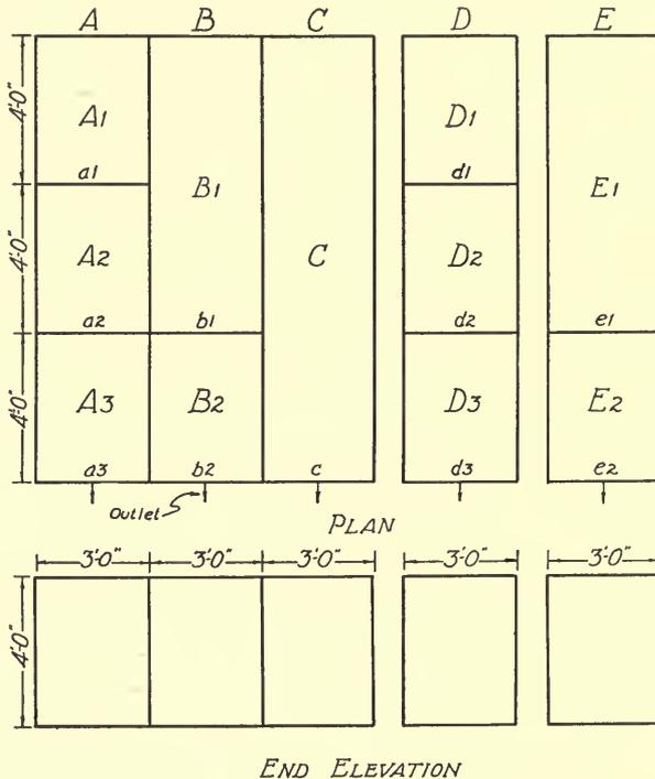
FIG. 4.—PLAN AND END ELEVATION OF EXPERIMENTAL SEPTIC TANKS USED IN STUDY II
