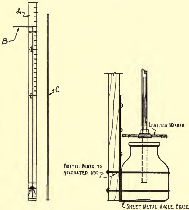
FIG. 9.—DEVICE FOR MEASURING THE DEPTH OF SLUDGE
