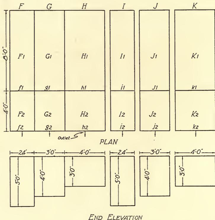
FIG. 17.—PLAN AND END ELEVATION OF EXPERIMENTAL SEPTIC TANKS USED IN STUDY OF DIFFERENTLY SHAPED CROSS-SECTIONS
