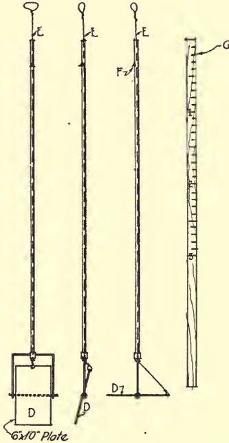
FIG. 8.—DEVICE FOR MEASURING THE THICKNESS OF SCUM
