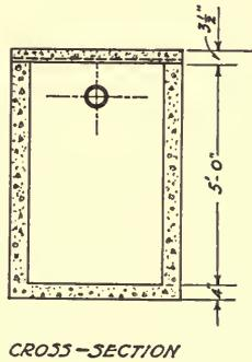
FIG. 24.—SUGGESTED DESIGN FOR A SINGLE-CHAMBER SEPTIC TANK
