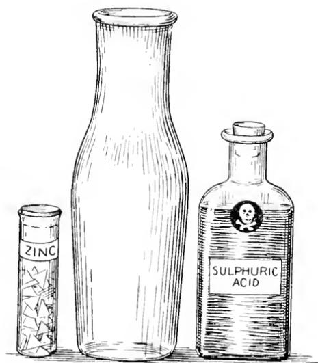
FIG. 4.—Apparatus used in preparing hydrogen.
