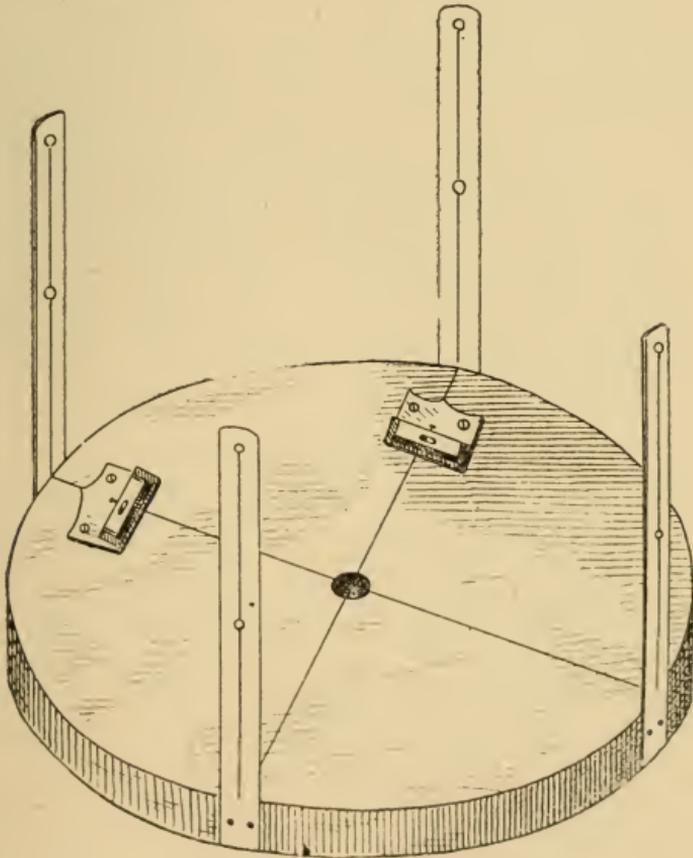
thin pieces of wood, 1 inch wide and 8 inches long, and make a slit  $\frac{1}{32}$  of an inch wide through the middle of each, to within one inch of each end. These being for the sights they must be fastened to the edge of the wheel or let in their thickness, so that their slits will
