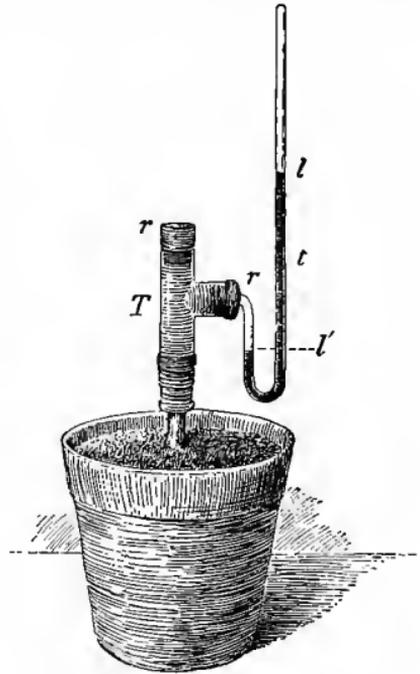
FIG. 23. Apparatus to measure Sap-Pressure.
