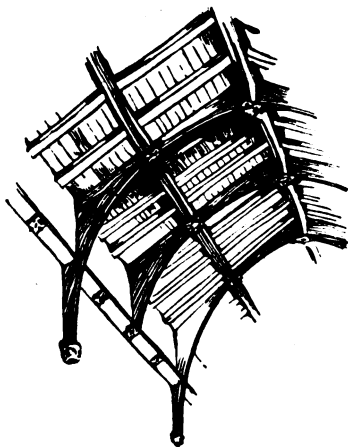
FIG. 71. ROOF WITH ARCHED PRINCIPALS, NORTH ELMHAM
