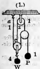
In a Spanish Burton, Fig. 1, where the ends of one cord, *a P*, are fastened to the support and the power, and the ends of the other, *c o*, to the lower and upper blocks, the weight is to the power as 4 to 1.
