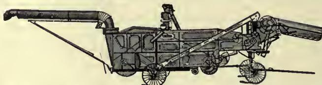
FIG. 4.—American "Separator" with self-feeder and fan-blast delivery-pipe for straw. (Avery Manufacturing Co., Peoria, Illinois.)
