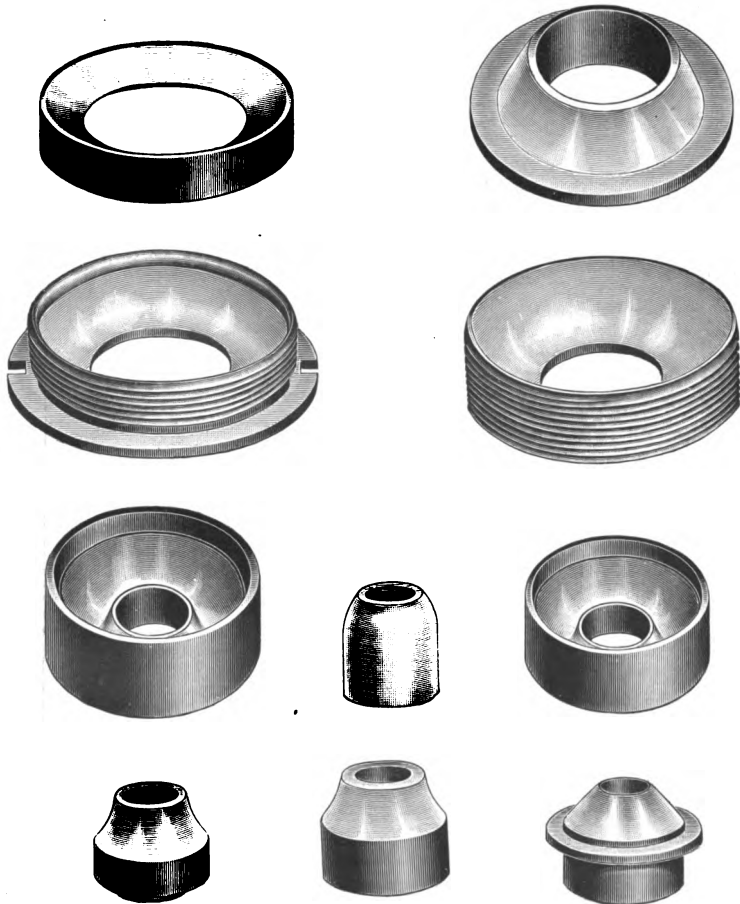
Fig. 67. Samples of Work ground on Machine, fig. 63.
