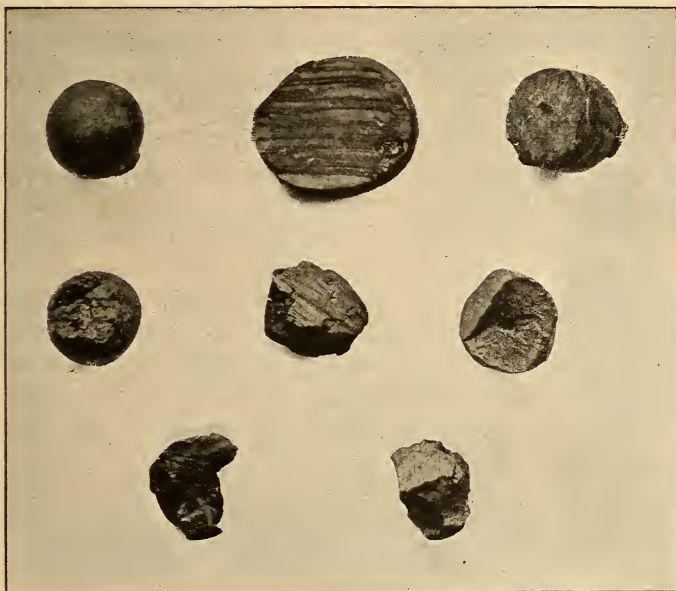
FIG. 94.—Normal, deformed, and fractured leaden shrapnel bullets. (Makins.)
