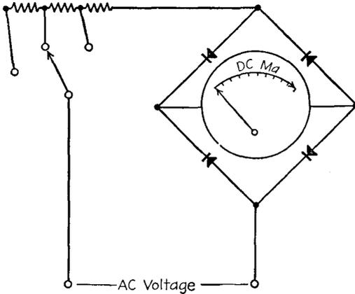
FIG. 4-12.—Typical multirange AC voltmeter.
