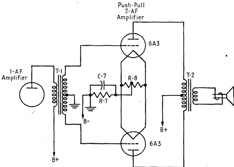
Fig. 21-8.—Schematic diagram of a transformer-coupled push-pull stage.
