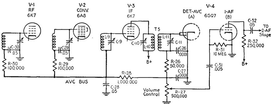
FIG. 12-5.—Typical detector and AVC circuit.
