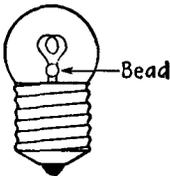
FIG. 18-16.—A pilot lamp showing position of bead.
