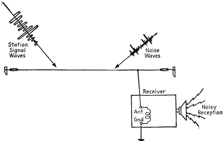
FIG. 17-2.—Noise and signal pickup by an antenna.
