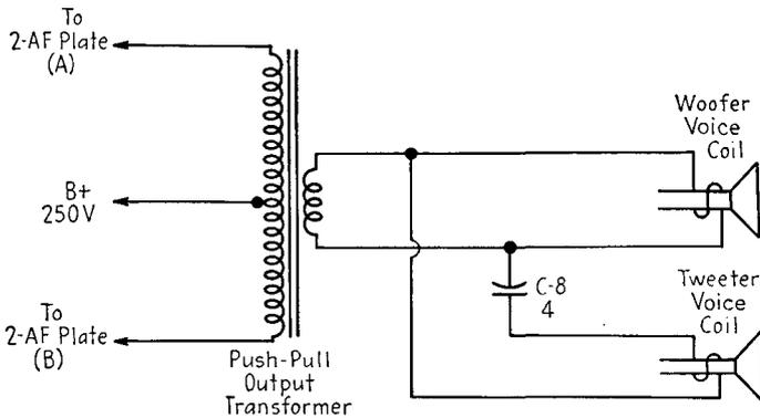
FIG. 21-18.—A high-fidelity loudspeaker system.
