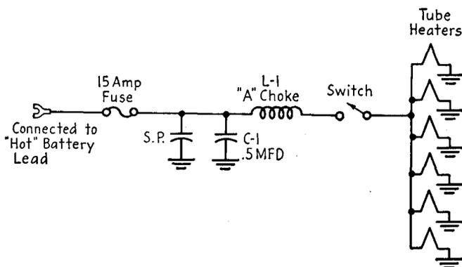
FIG. 20-1.—Typical auto radio heater circuit.
