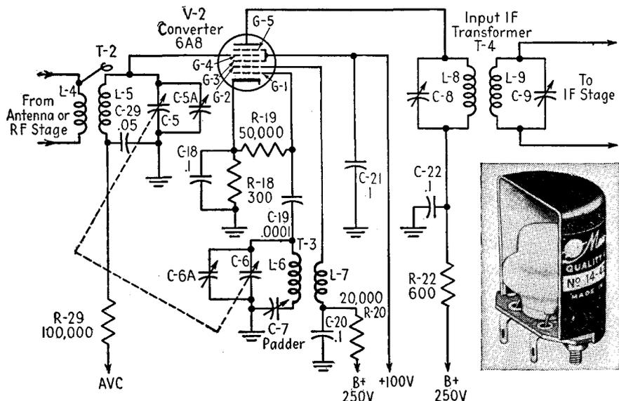
FIG 14-21.—A typical oscillator coil and its position in the converter circuit.
