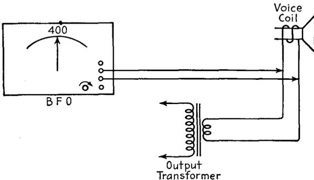
FIG. 9-6.—Checking a speaker with a beat-frequency oscillator.
