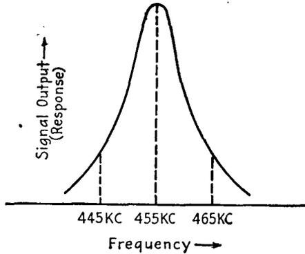
FIG. 13-16.—Frequency-response curve of the usual IF transformer.
