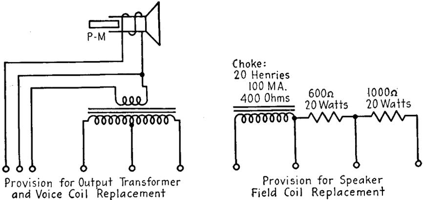
FIG. 24-3.—Bench test speaker.
