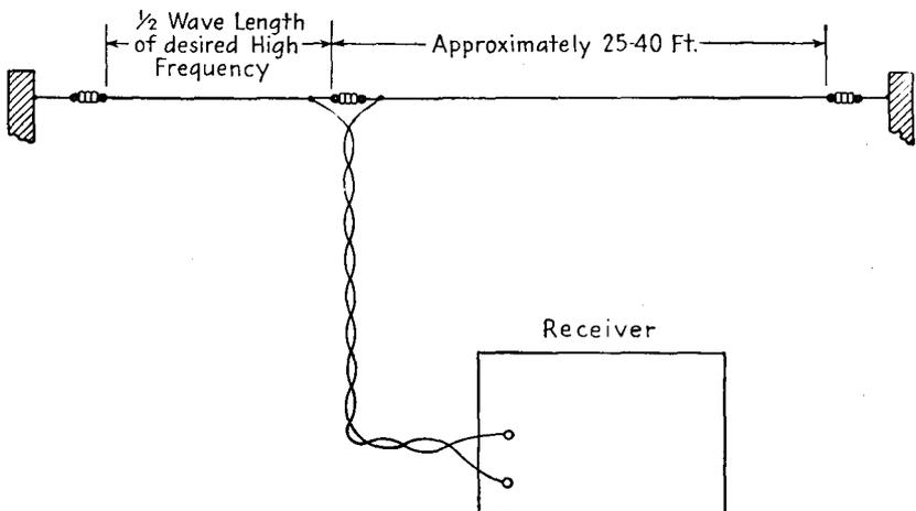
FIG. 17-24.—The asymmetrical dipole antenna.
