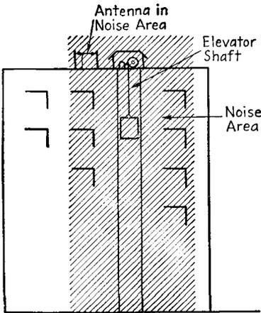
FIG. 17-9.—An antenna installed in a noise area.
