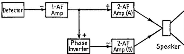
FIG. 21-9.—Block diagram of a phase-inverter type of push-pull amplifier.
