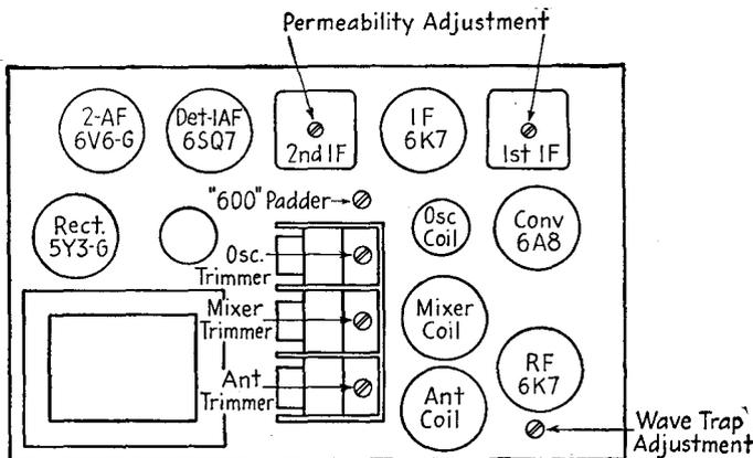
FIG. 22-5.—Layout diagram of a six-tube superheterodyne receiver.
