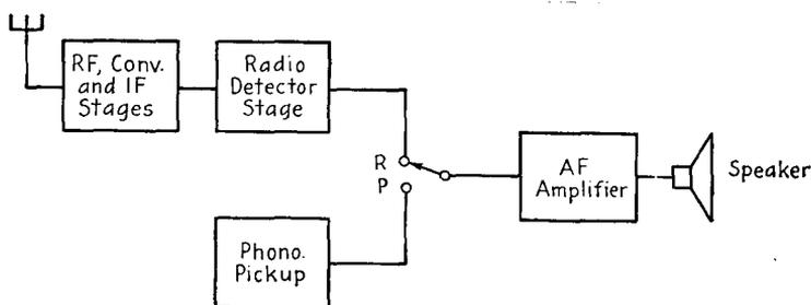
FIG. 12-15.—Block diagram of radio-phonograph operation.
