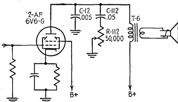
Fig. 10-12.—Tone Control in the second AF stage.
