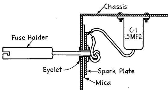
FIG. 20-2.—Spark-plate filter connected to the "hot" battery lead at the point of entry to the receiver.
