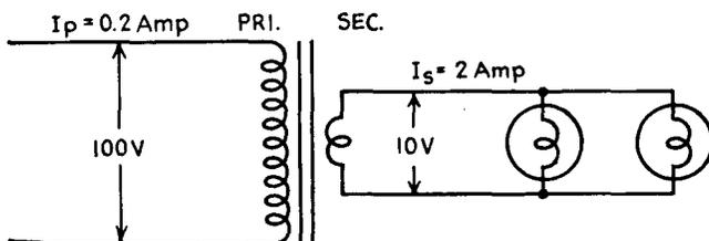
FIG. 10-8.—Transformer lighting two lamps.
