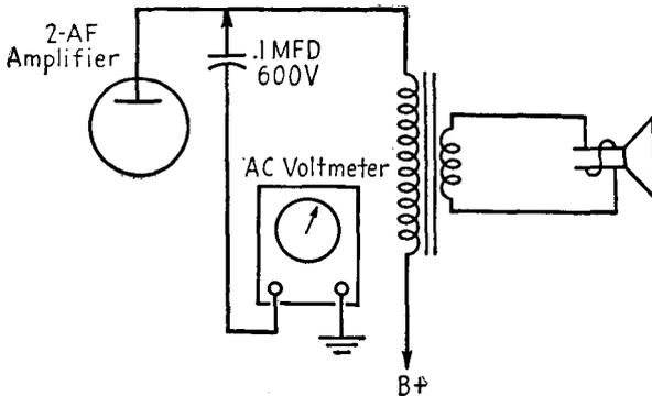
FIG. 22-3.—Connecting an output indicator for alignment.
