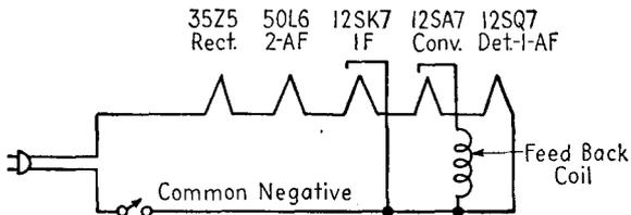
FIG. 18-22.—How a cathode-to-heater short affects other tubes.
