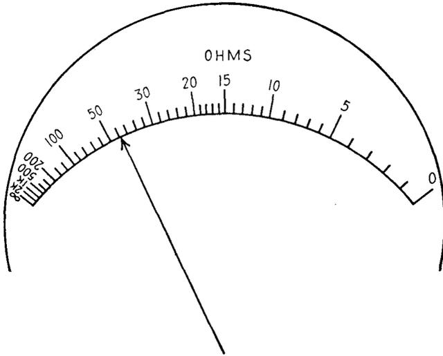
FIG. 4-14.—Typical ohmmeter scale.
