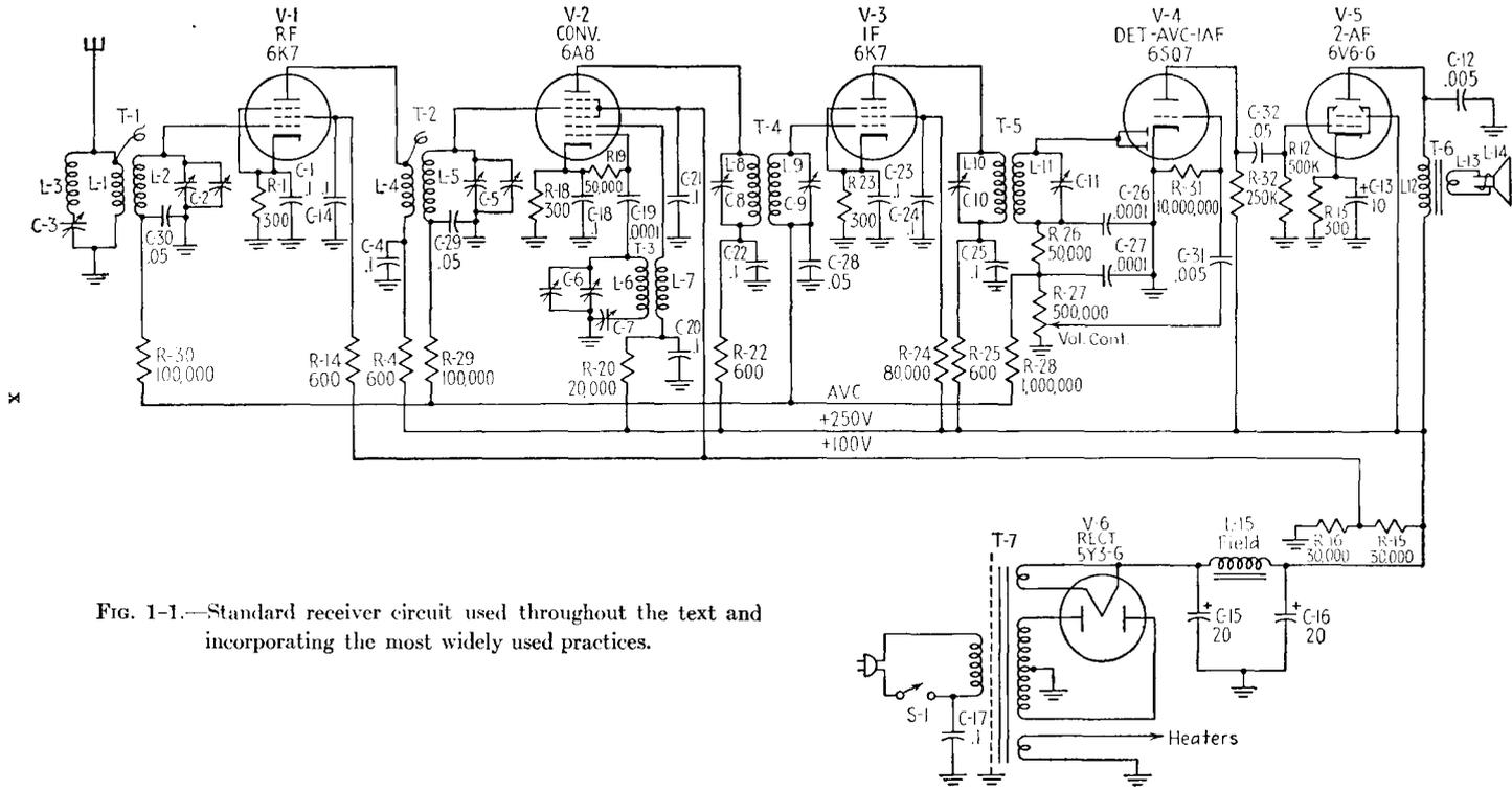
FIG. 1-1.—Standard receiver circuit used throughout the text and incorporating the most widely used practices.
