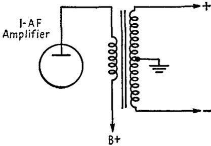
FIG. 21-2.—The center-tapped transformer for obtaining input voltages for a push-pull stage.
