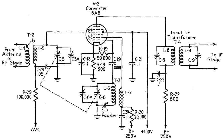
FIG. 14-1.—Typical pentagrid converter circuit.
