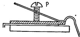
FIG. 14-25.—Low-capacity setting for padder *P*.
