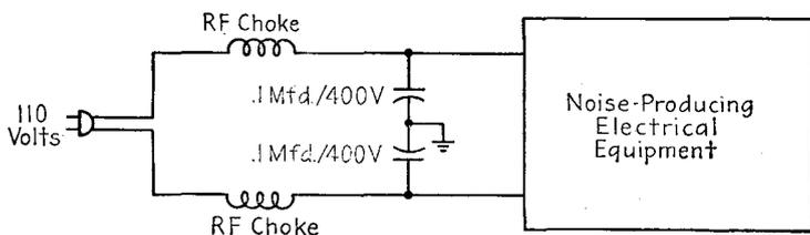
FIG. 17-16.—Filtering line noise at the source.
