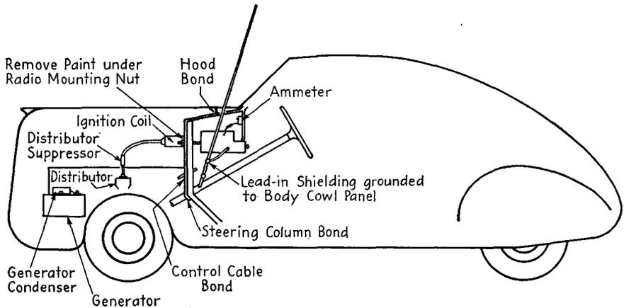
Fig. 19-14.—Standard automobile radio installation for side-cowl antennas.
