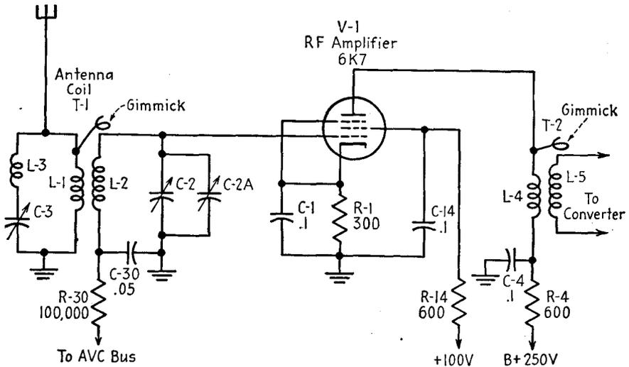
FIG. 16-2.—Schematic diagram of a typical RF stage.
