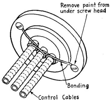
FIG. 19-11.—Control-cable bonding installation.
