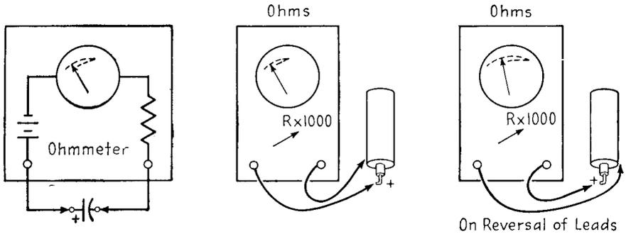
FIG. 8-11.—Checking an electrolytic condenser with an ohmmeter.
