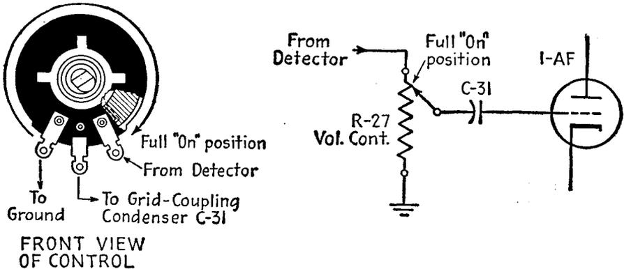
FIG. 11-16.—Volume-control connections.
