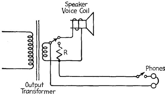
Fig. 9-17.—Circuit for connecting earphones to a receiver.
