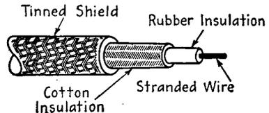
Fig. 17-11.—Structure of shielded lead-in wire.
