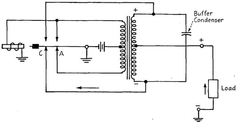
FIG. 20-20.—The synchronous vibrator: operation position 1.
