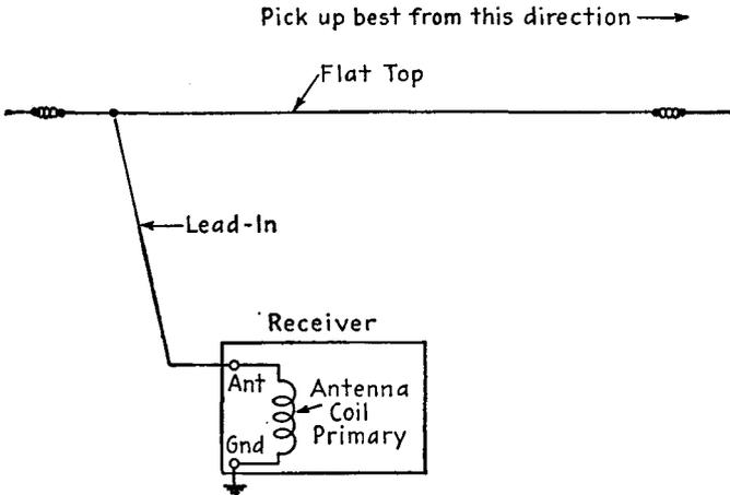
FIG. 17-1.—Simple inverted-L antenna.
