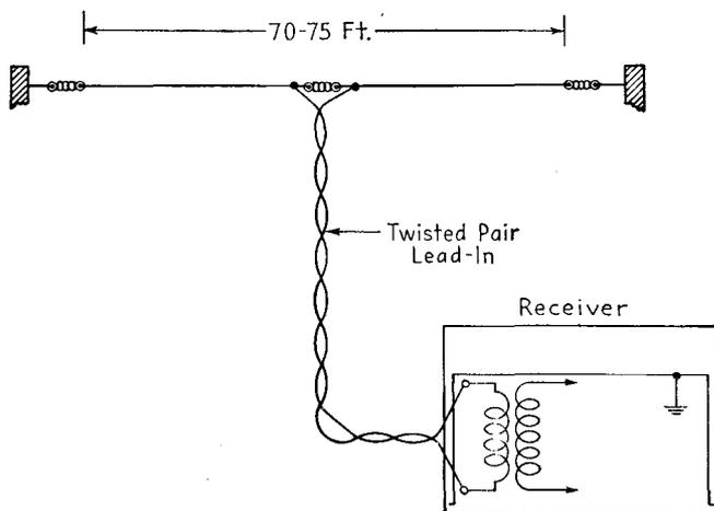
FIG. 17-22.—The Hertzian dipole antenna.
