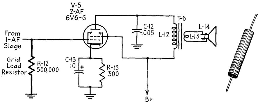
FIG. 10-4.—A typical grid-load resistor and its position in the second AF circuit.
