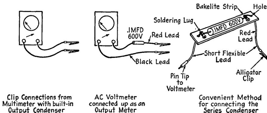
Fig. 11-7.—Test leads for the output meter.
