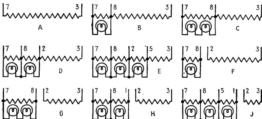
FIG. 18-18.—Standard base wiring for ballast tubes.
