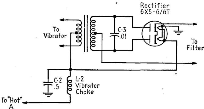
FIG. 20-9.—Full-wave rectifier in the vibrator-type power supply.
