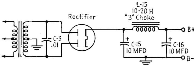
FIG. 20-11.—Filter circuit in the vibrator-type power supply.
