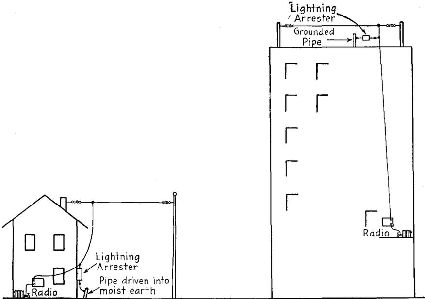
FIG. 17-8.—The installation of lightning arresters.
