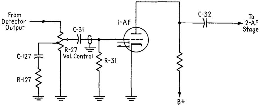
FIG. 11-22.—Bass compensation in the first AF stage.
