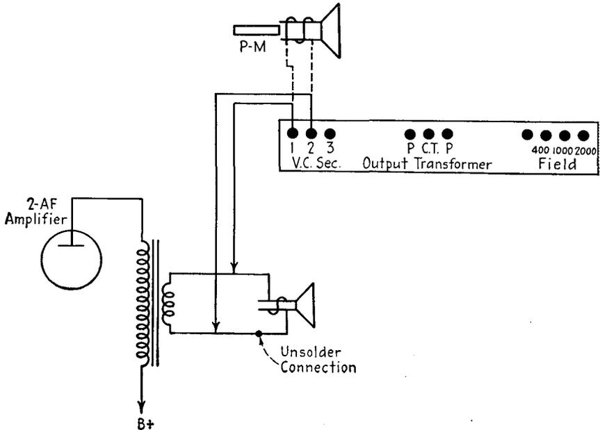
FIG. 24-5.—Checking a speaker voice coil by substituting the bench test speaker.
