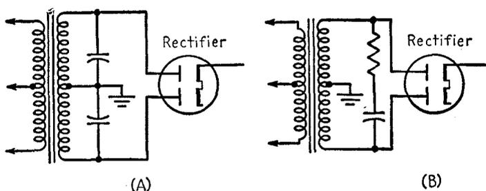
FIG. 20-16.—Variations in the buffer-condenser circuit.
