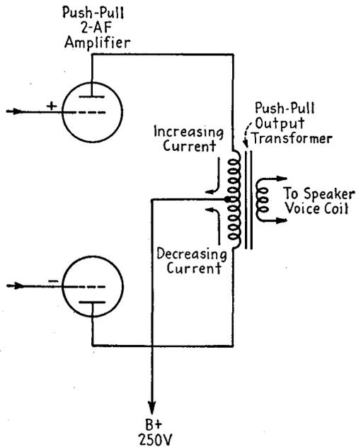
FIG. 21-5.—The output circuit of a push-pull amplifier.
