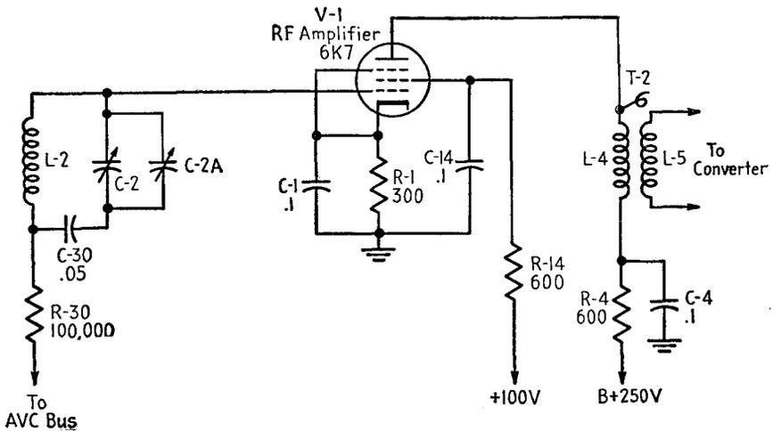
FIG. 16-6.—Decoupling filters in the RF stage.
