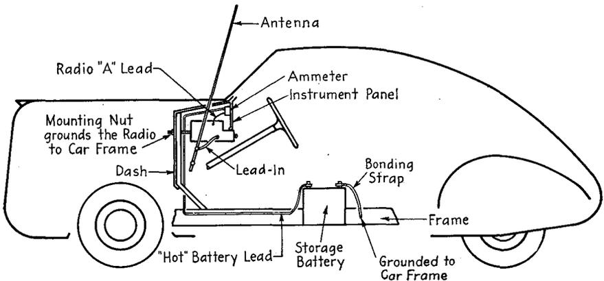
FIG. 19-1.—Typical automobile radio installation.
