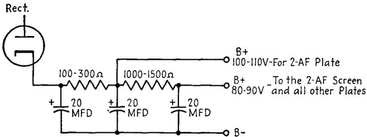
FIG. 18-27.—Two-section R-C filter.
