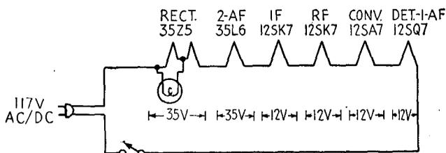
FIG. 18-5.—Heater circuit for a six-tube receiver using 0.15-amp tubes.
