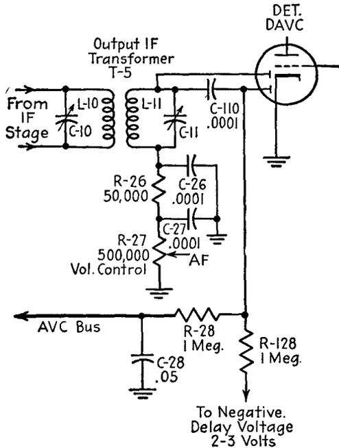
FIG. 12-13.—Delayed AVC circuit.
