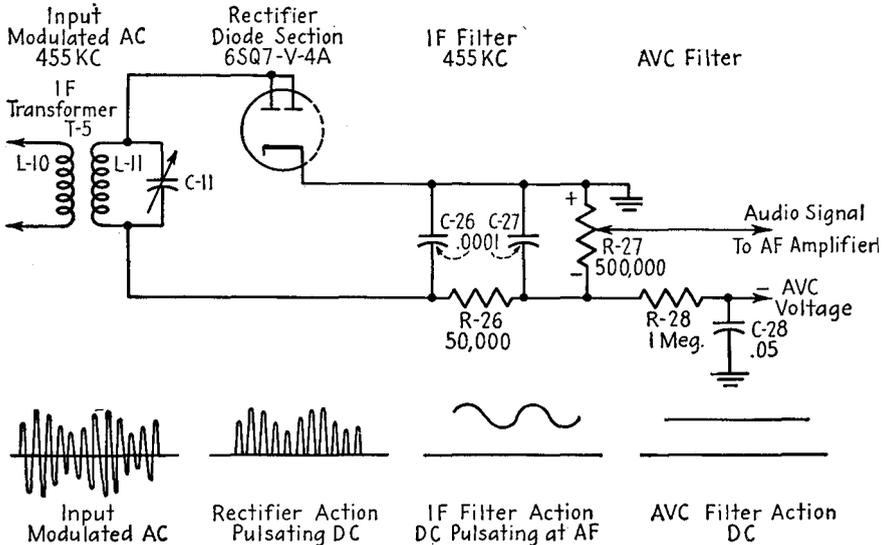
FIG. 12-4.—Developing audio signal and AVC voltage from the modulated intermediate-frequency signal.
