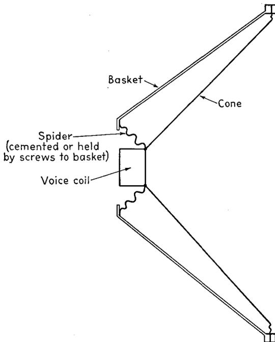
FIG. 9-9.—Inside spider connected to speaker basket.
