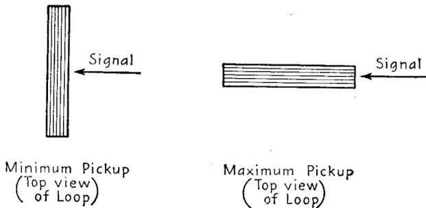
FIG. 17-21.—Directional characteristic of a loop antenna.
