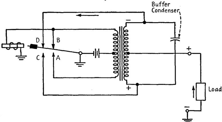
Fig. 20-21.—The synchronous vibrator: operation position 2.
