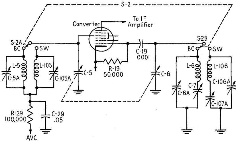
FIG. 15-3.—Simplified switching circuits for a multiband receiver.
