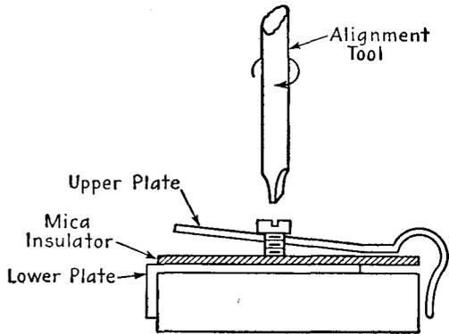
FIG. 22-7.—Adjusting a trimmer condenser.
