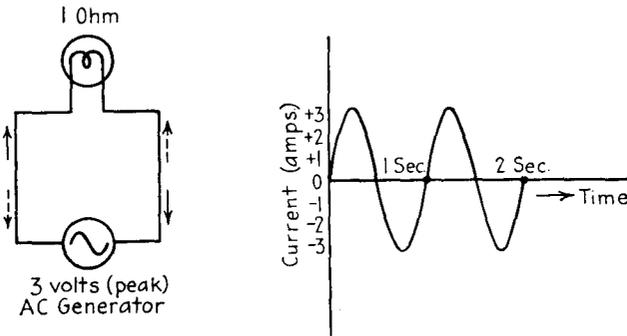
Fig. 5-3.—Circuit and wave form for a pure alternating current (AC).
