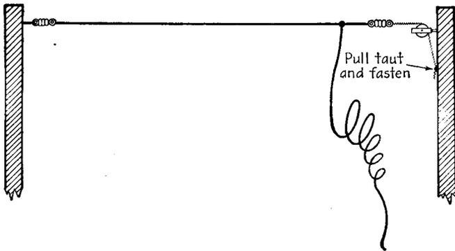
FIG. 17-6.—Attaching the second end of the antenna.
