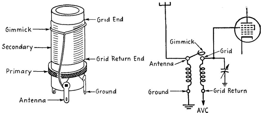
FIG. 14-12.—Antenna coil leads.
