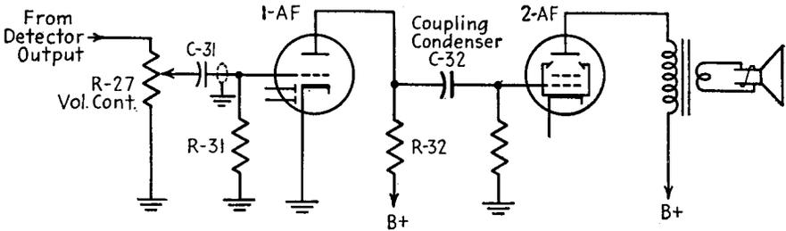
FIG. 11-20.—Coupling condenser C-32 between the first AF and second AF stages.
