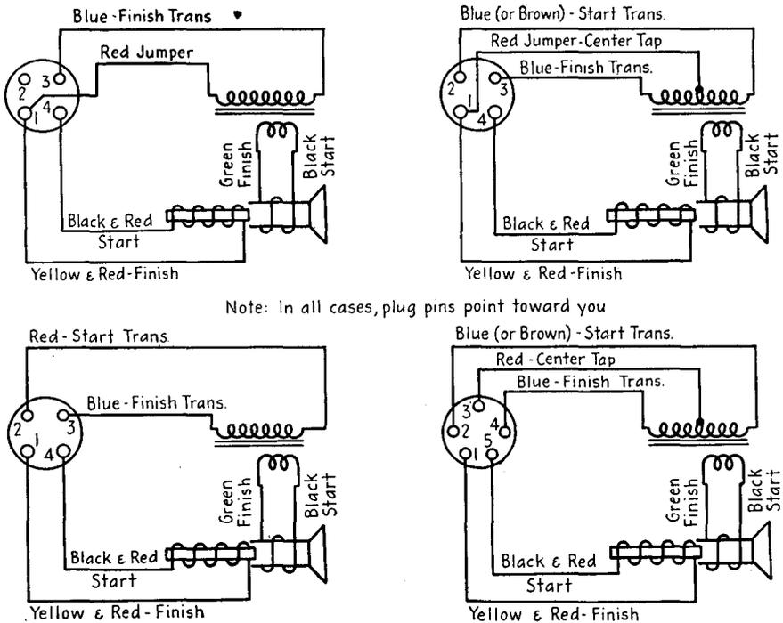
FIG. 24-7.—R.M.A. speaker-plug wiring systems.
