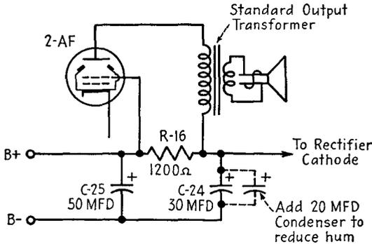
FIG. 18-29.—Replacing a hum-bucking-type output transformer. Method 1.
