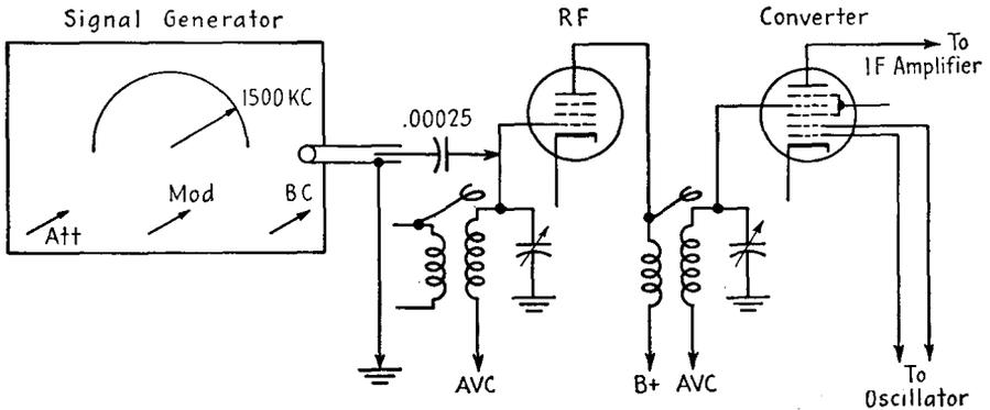
FIG. 14-6.—Signal-generator connections for stage-gain measurements of the converter when the receiver incorporates an RF stage.
