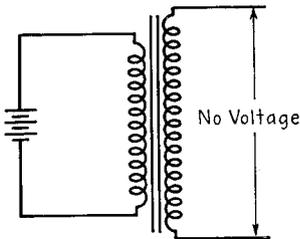
FIG. 20-4.—Transformer fed with direct current.
