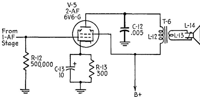
FIG. 10-6.—The AF by-pass condenser and its position in the second AF circuit.
