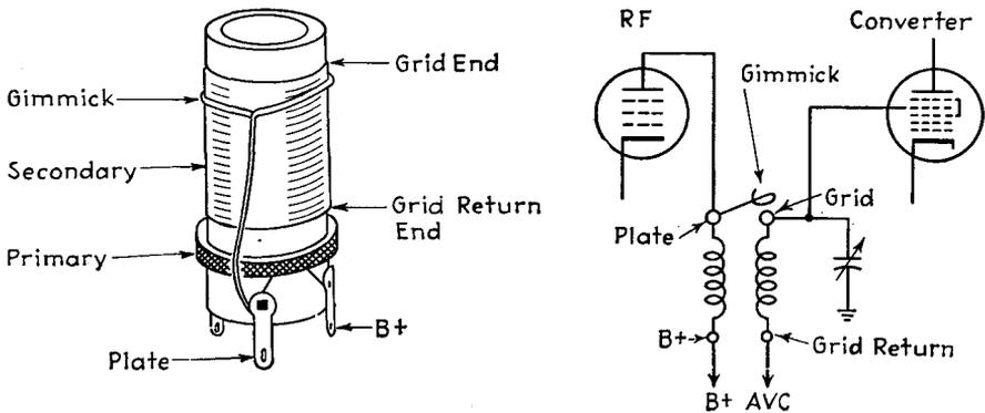
Fig. 14-10.—Interstage RF transformer leads.
