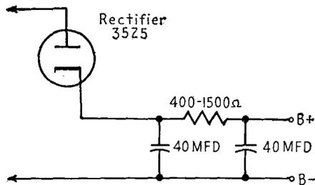
Fig. 18-7.—An AC/DC *B* power supply using an R-C filter.
