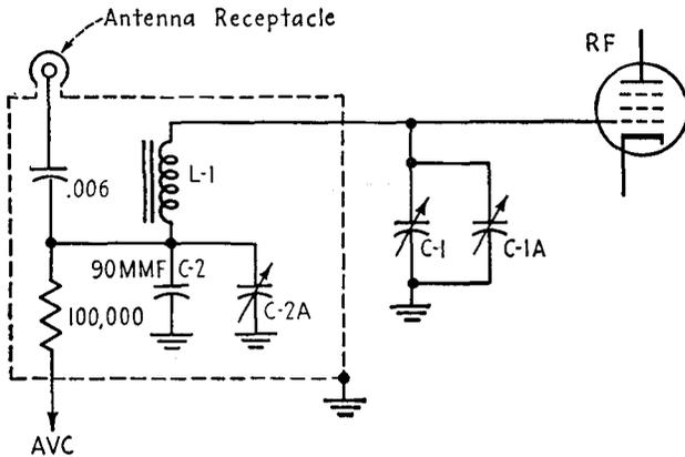
FIG. 19-3.—Automobile radio antenna coupling circuit.
