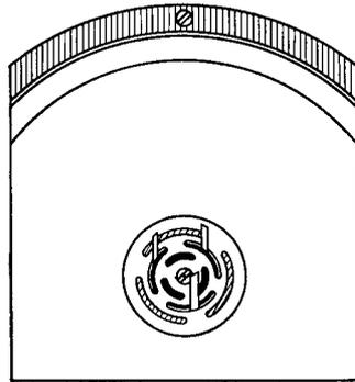
FIG. 9-8.—Centering a voice coil with three shims.
