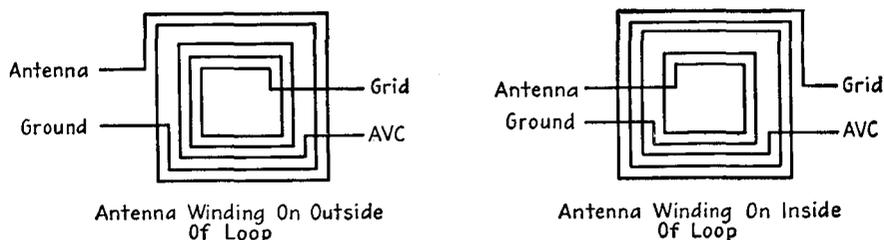
FIG. 14-15.—Identifying loop antenna leads.
