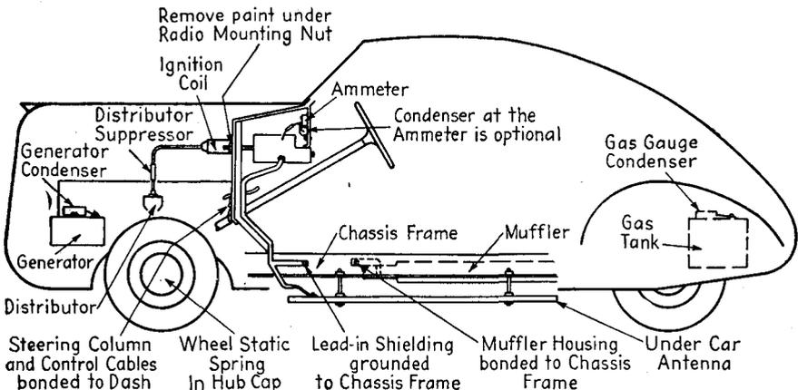
FIG. 19-16.—Standard automobile radio installation for under-car antennas.
