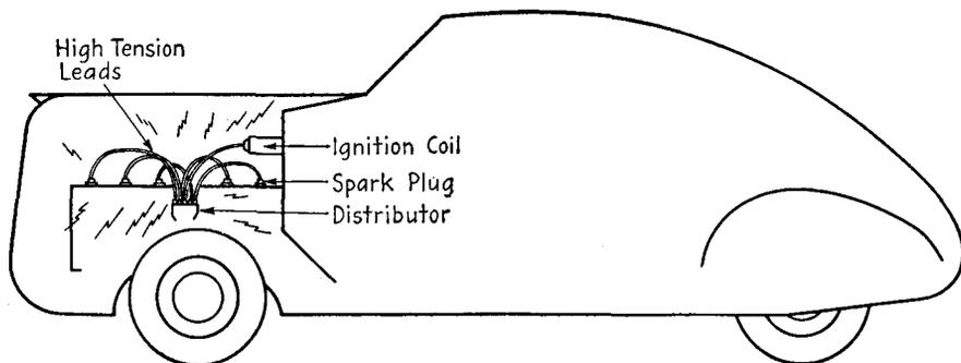
FIG. 19-4.—RF interference from the ignition wiring.
