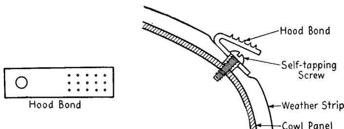
FIG. 19-6.—Hood-bond installation.
