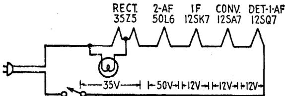
Fig. 18-4.—A typical AC/DC heater circuit for 0.15-amp tubes.
