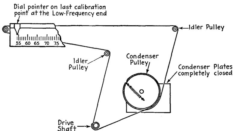
FIG. 22-11.—Setting the dial pointer.
