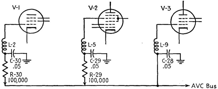
FIG. 13-9.—Decoupling filters in the grid return circuit to avoid coupling in the common AVC voltage supply.
