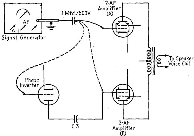
FIG. 21-15.—Signal check of a push-pull amplifier.
