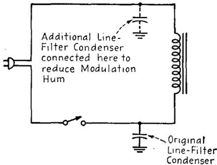
Fig. 23-1.—Procedure for reducing modulation hum.
