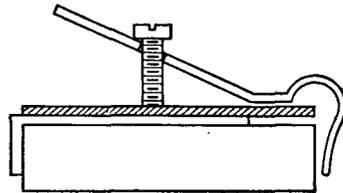
FIG. 22-8.—A trimmer condenser at its low-capacity setting.
