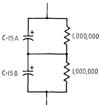
FIG. 8-12.—Connecting two condensers to increase voltage rating.
