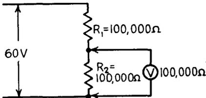
FIG. 4-7.—Measuring voltage with a 1,000-ohms-per-volt meter.
