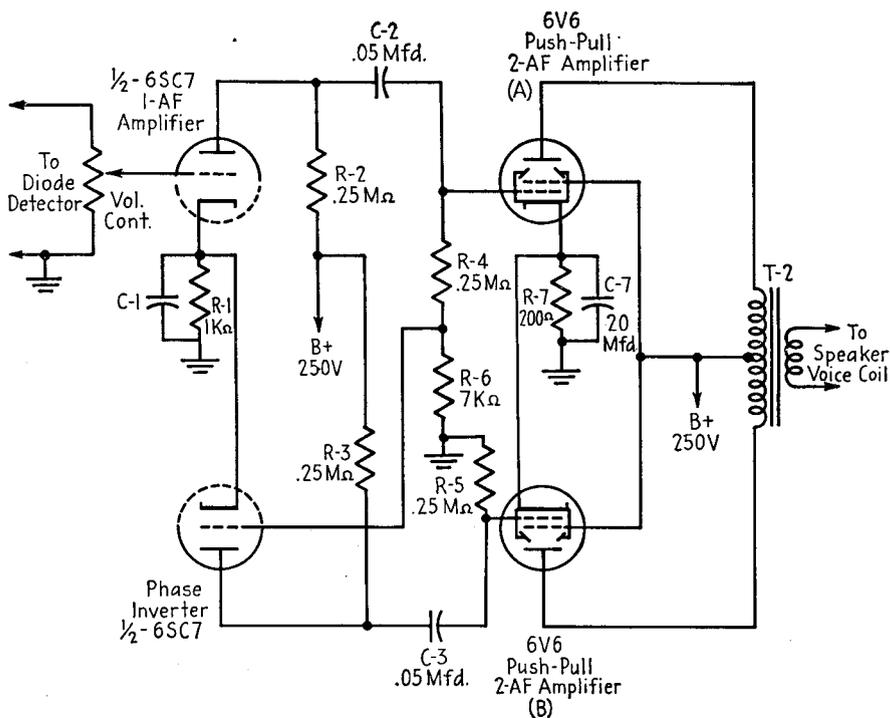
FIG. 21-16.—Schematic diagram of a typical push-pull amplifier.
