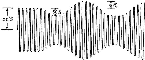
FIG. 6-2.—A 30 per cent modulated RF signal.
