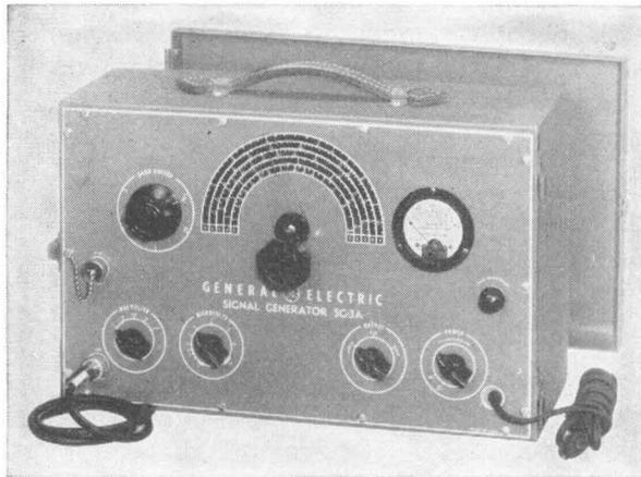
FIG. 6-6.—The General Electric signal generator, Model SG-3A.
