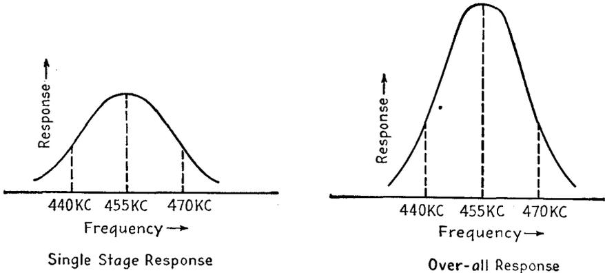
FIG. 13-18.—Frequency-response curve of a high-fidelity IF amplifier.
