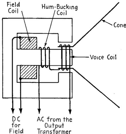
FIG. 9-5.—Electrodynamic speaker with a hum-bucking coil.
