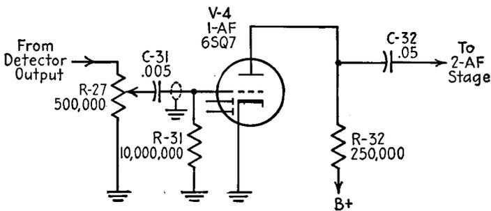
FIG. 11-1.—Typical first audio-frequency amplifier stage.
