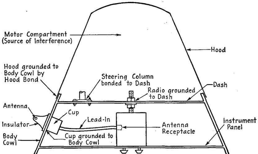
FIG. 19-10.—Top view of automobile radio installation.
