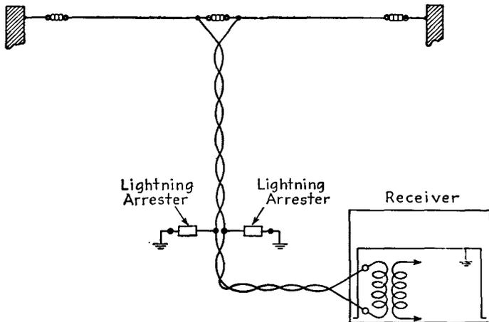
FIG. 17-23.—Connecting lightning arresters to a twisted-pair leadin.
