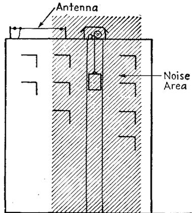
FIG. 17-10.—Moving antenna out of the noise area.
