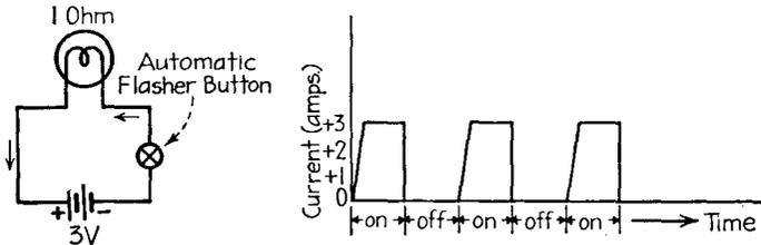
Fig. 5-2.—Circuit and wave form for a varying direct current.
