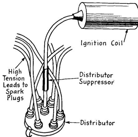
FIG. 19-5.—Distributor-suppressor installation.
