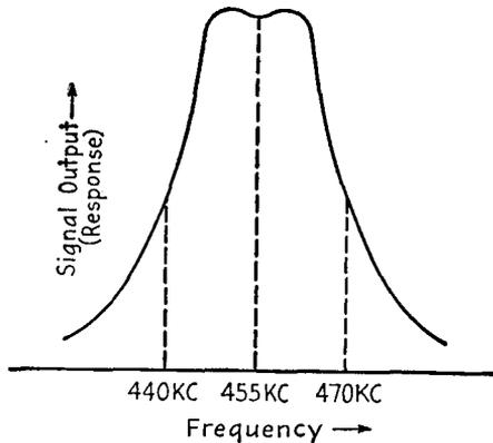
FIG. 13-17.—Frequency-response curve of a high-fidelity IF transformer.
