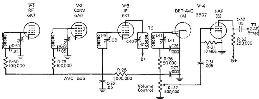
FIG. 12-11.—The AVC circuit.
