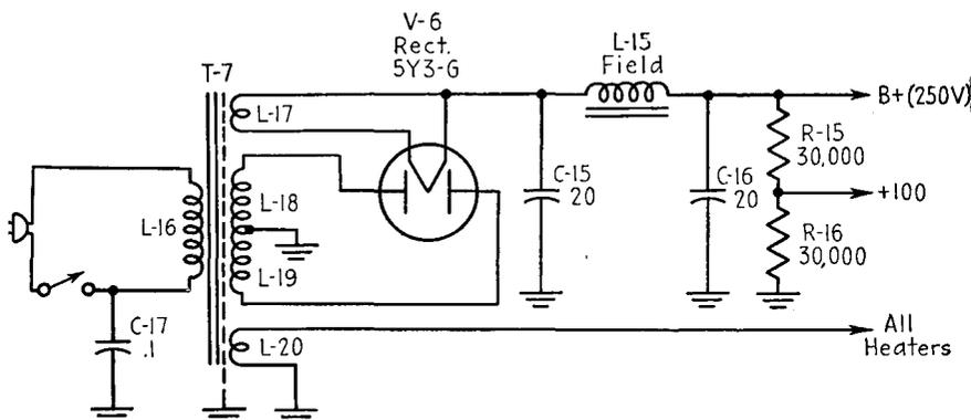
FIG. 8-2.—Standard circuit of AC power supply.
