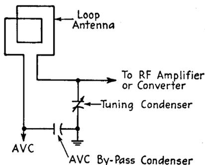
FIG. 17-19.—The loop antenna.
