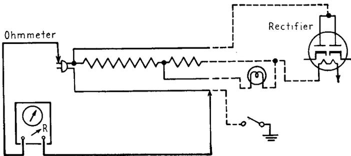
FIG. 18-17.—Identifying leads of a resistor-type line cord.
