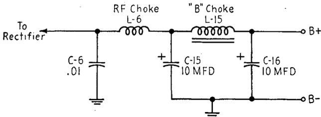
FIG. 20-17.—The auto radio *B* filter circuit.
