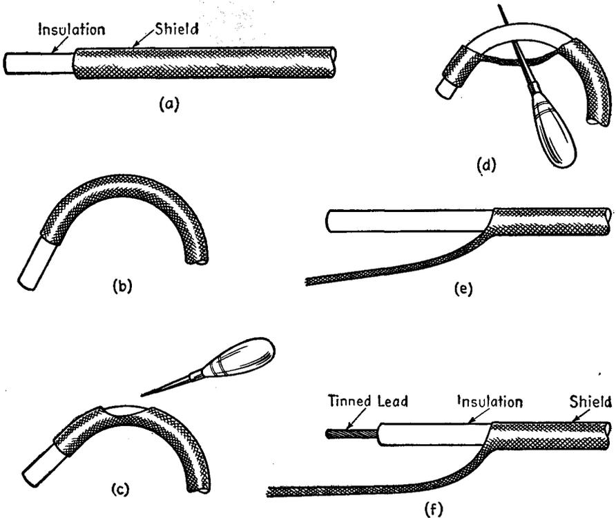
FIG. 11-18.—How to prepare shielded wire for use.
