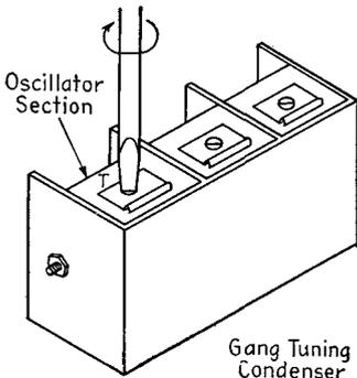
FIG. 14-27.—Adjusting the high-frequency trimmer  $T$ .
