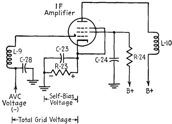
Fig. 13-3.—The grid bias applied to the IF tube is the sum of the self-bias and AVC voltages.
