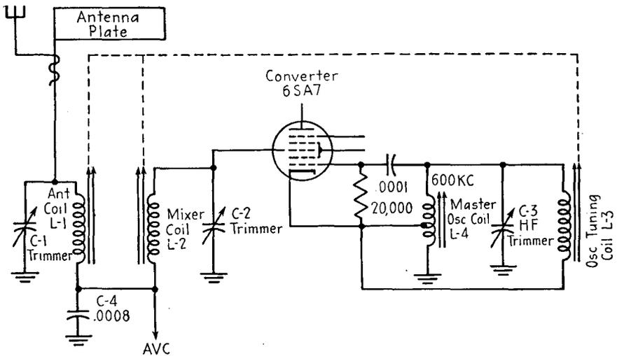
FIG. 15-16.—Three-coil permeability tuner with a preselector circuit.
