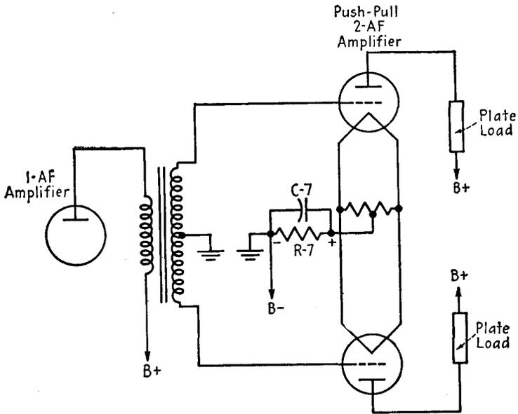
FIG. 21-4.—A method of obtaining bias voltage for a push-pull stage.
