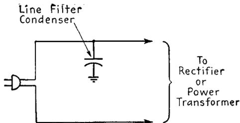
FIG. 17-14.—Line filter condenser in a receiver.
