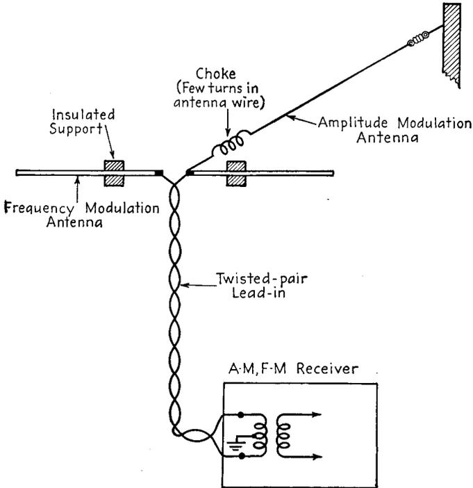
FIG. 17-25.—A-M and F-M antenna.
