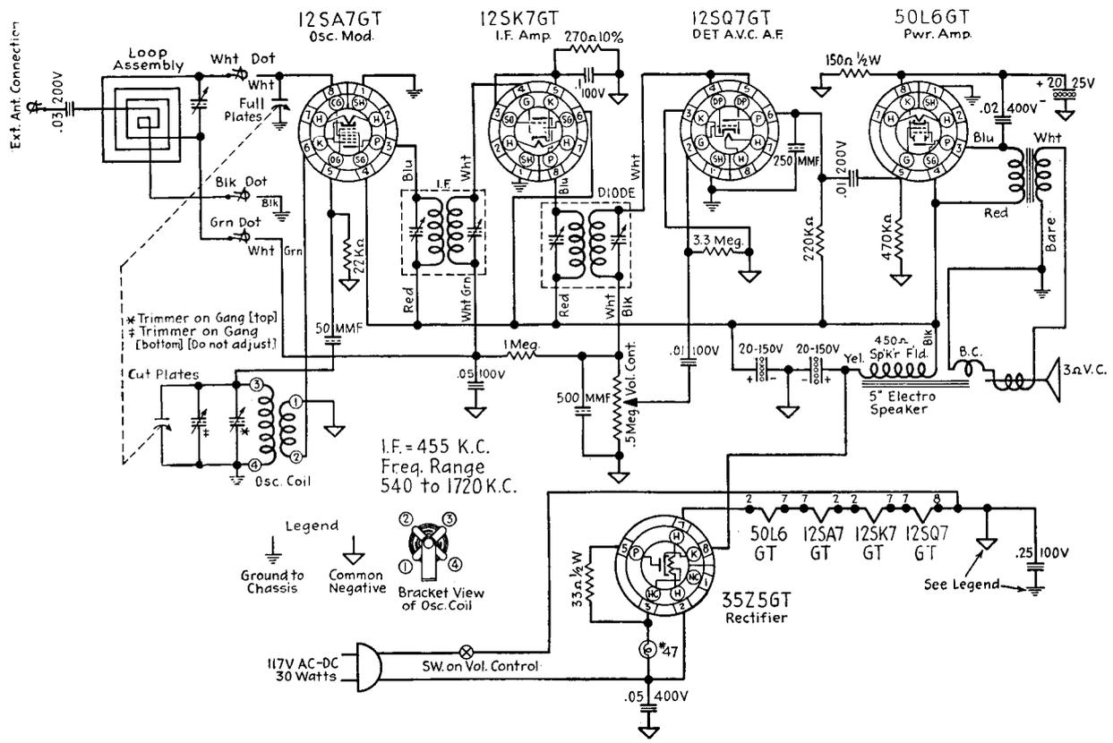
Fig. 7-5.—The Motorola Model 56X1 AC/DC receiver.
