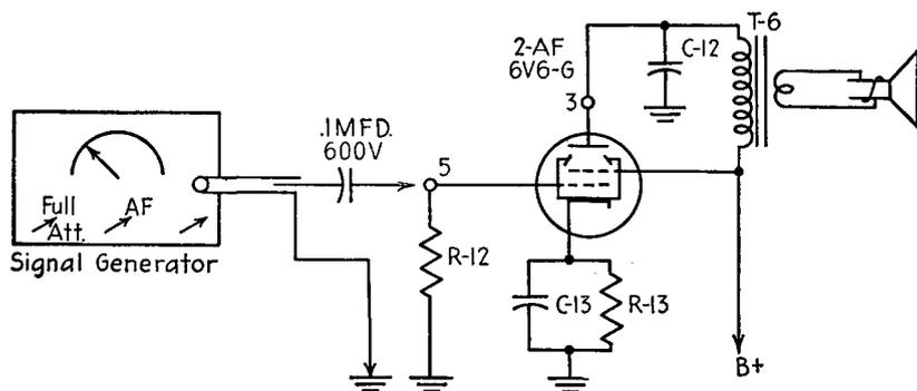
FIG. 10-3.—Signal check of the second AF stage.
