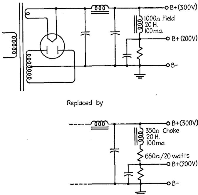
FIG. 9-13.—Replacing an electromagnetic with a P-M dynamic speaker—field-circuit adjustments.
