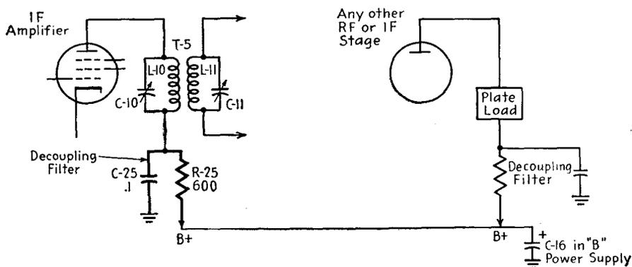
FIG. 13-14.—The IF amplifier plate-decoupling filter.
