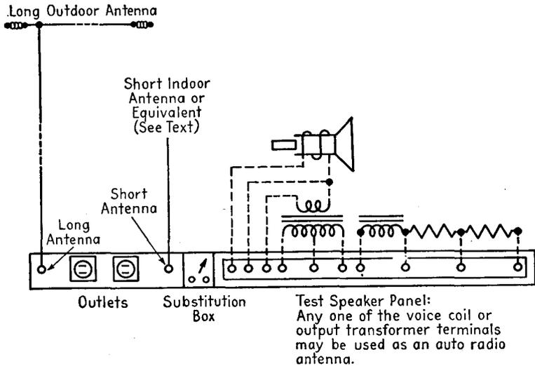
FIG. 24-10.—Panel on test bench showing antenna leads.
