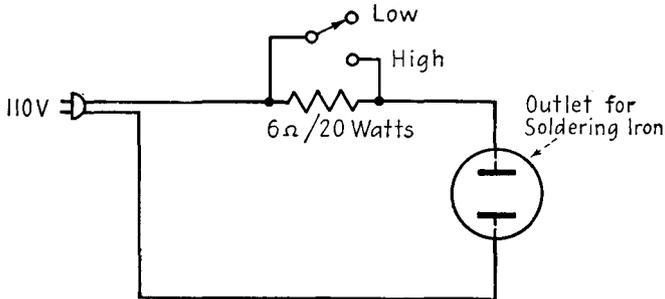
FIG. 24-13.—Schematic diagram of a “high-low” soldering-iron outlet.
