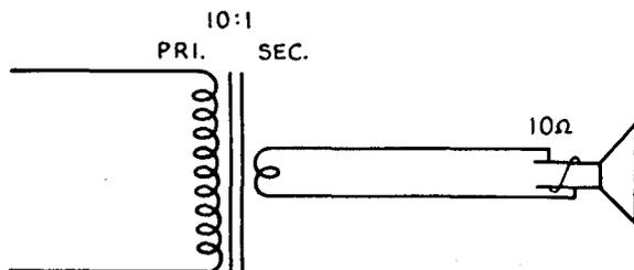
FIG. 10-9.—Transformer feeding a 10-ohm voice coil.
