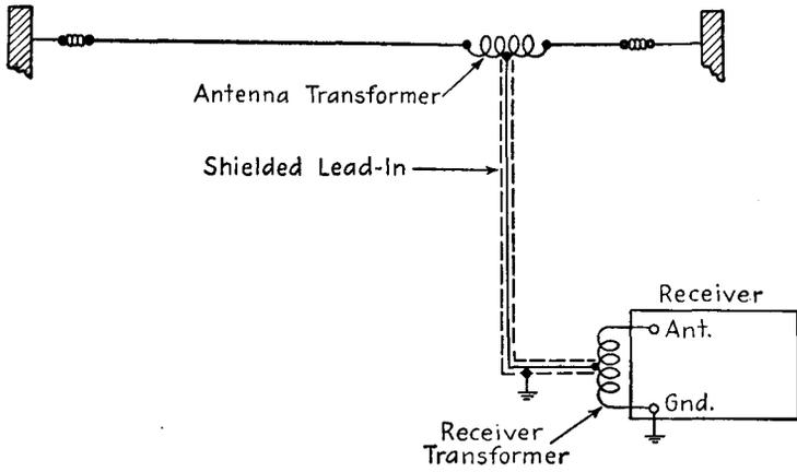
FIG. 17-12.—Noise reduction by the installation of coupling transformers and a shielded leadin.
