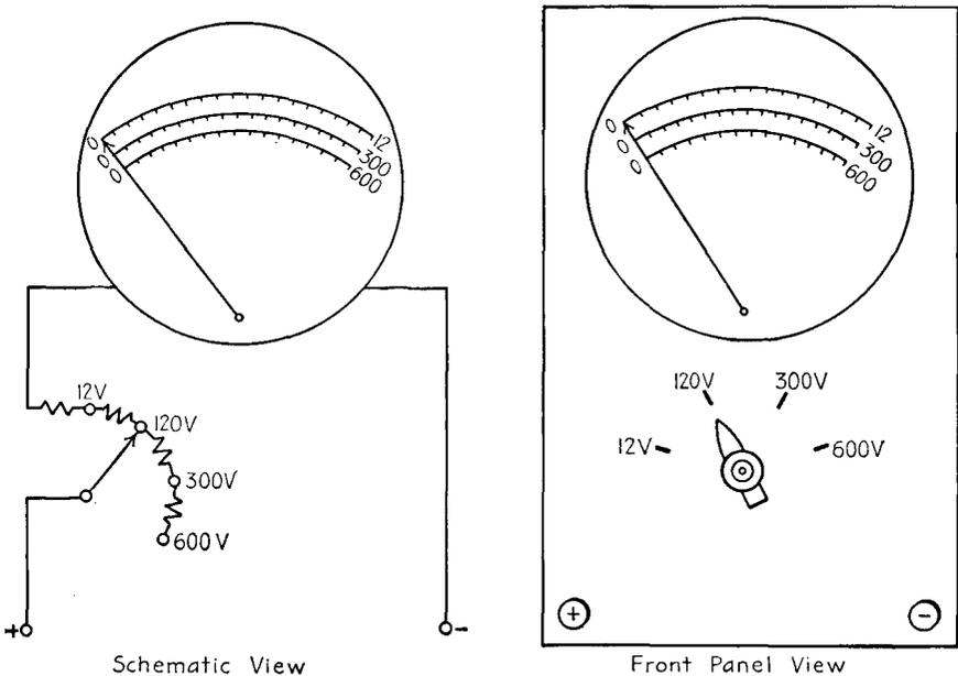
FIG. 4-5.—Multirange voltmeter showing range switch.
