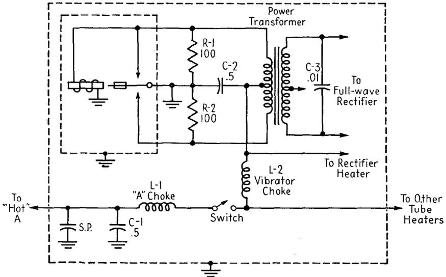
FIG. 20-7.—Typical vibrator circuit including provision for hash suppression.
