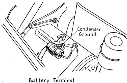
FIG. 19-12.—Generator-condenser installation.
