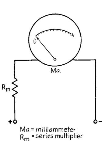
FIG. 4-2.—A basic voltmeter.
