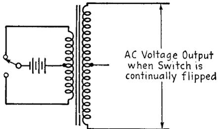
FIG. 20-5.—Reversing direct current through a transformer primary.
