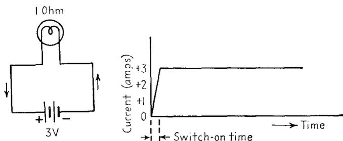
FIG. 5-1.—Circuit and wave form for a pure direct current (DC).
