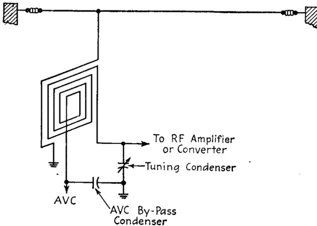
FIG. 17-20.—A loop with an antenna winding.
