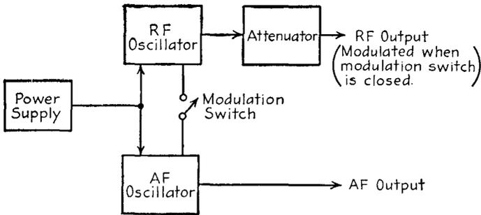
FIG. 6-1.—Block diagram of a signal generator.
