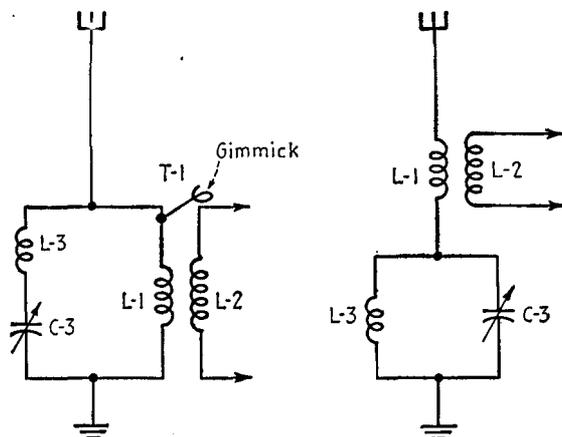
FIG. 16-7.—Common wave-trap circuits.
