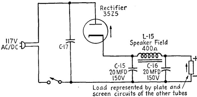
FIG. 18-6.—Typical AC/DC *B* power supply.
