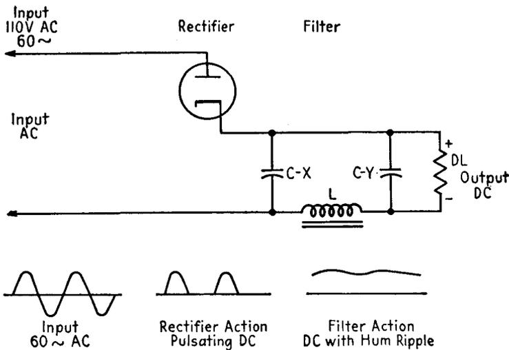
FIG. 12-1.—Half-wave *B* power supply.
