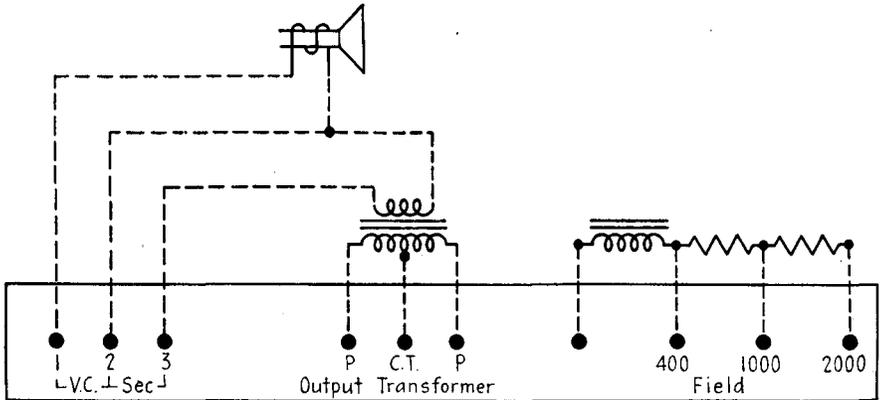
Note: When using Test Speaker Output Transformer, place a Shorting Jumper from 1 to 3. When using Receiver Output Transformer, use Terminals 1 and 2
