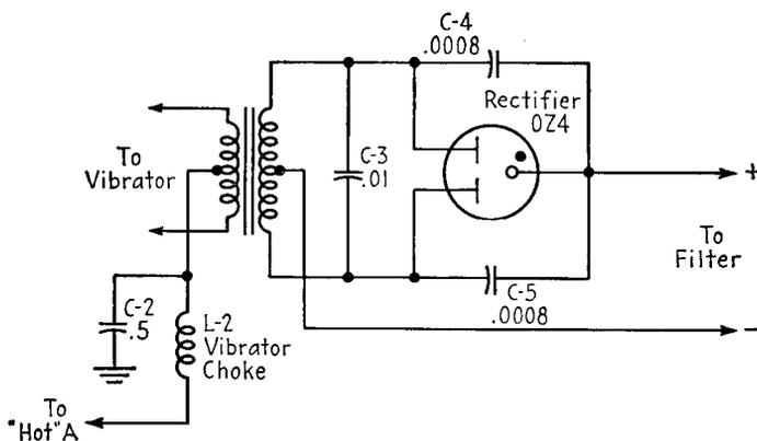
FIG. 20-10.—Cold-cathode type of rectifier circuit.
