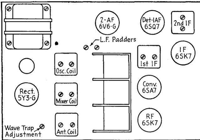
FIG. 22-6.—Layout diagram of a six-tube two-band receiver.
