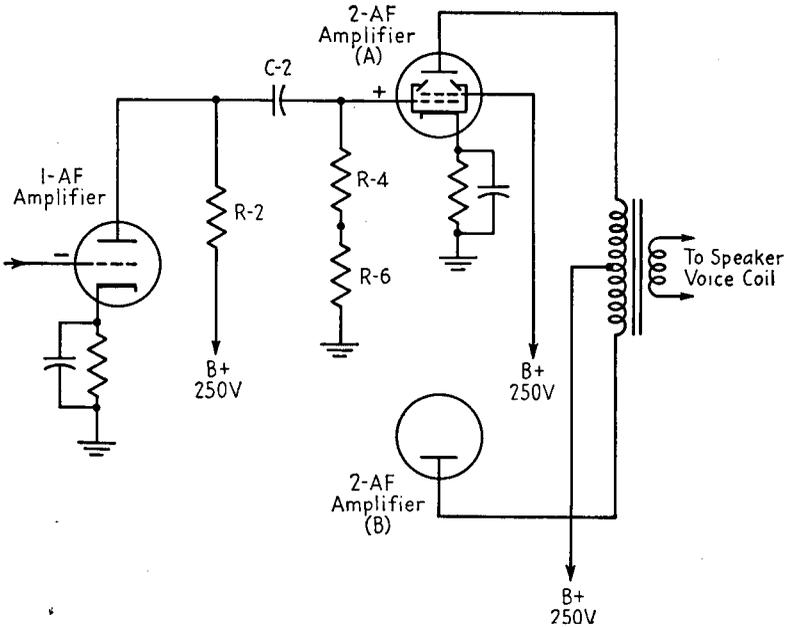
FIG. 21-10.—Obtaining a positive signal on one push-pull tube from a negative signal on the first AF amplifier grid.
