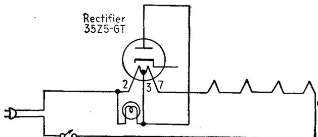
FIG. 18-21.—Pilot-lamp circuit for a 0.15-amp heater line.
