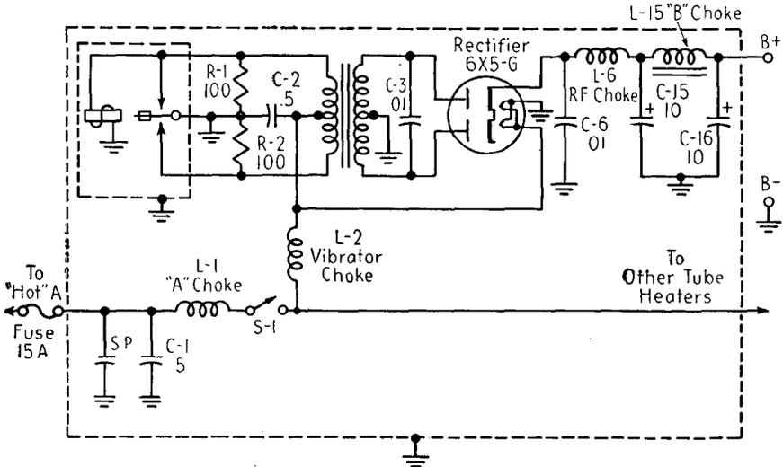
FIG. 20-14.—Typical auto radio vibrator-type power supply.
