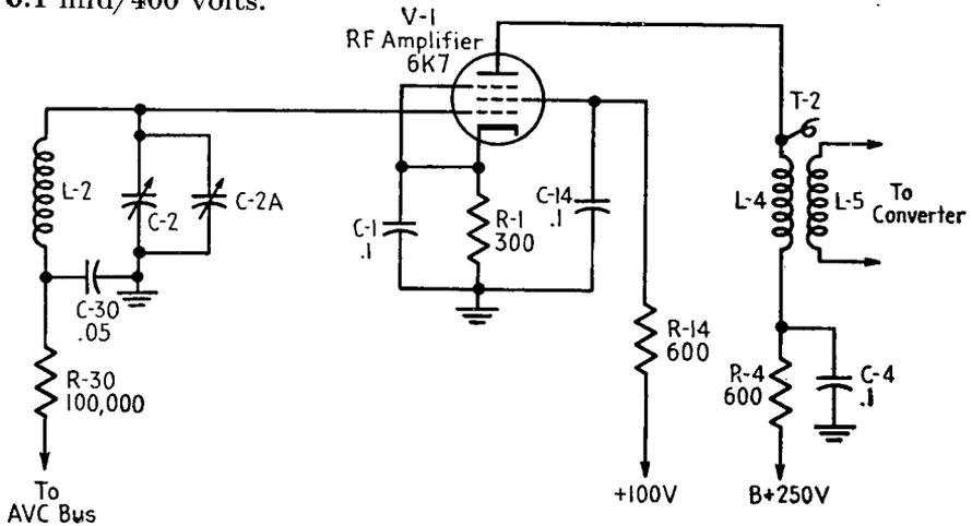
FIG. 16-4.—Decoupling filters in the RF stage.
