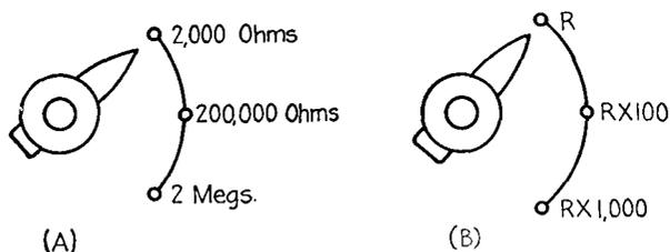
FIG. 4-15.—Typical ohmmeter range switches.
