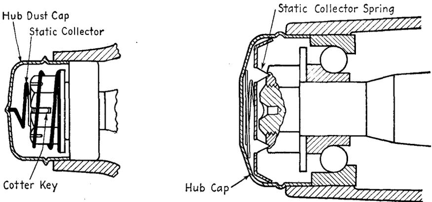
FIG. 19-13.—Front-wheel static-collector-spring installation.
