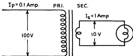
FIG. 10-7.—Transformer lighting one lamp.
