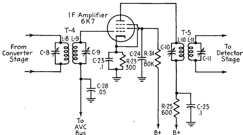
FIG. 13-1.—Typical circuit of an IF amplifier stage.
