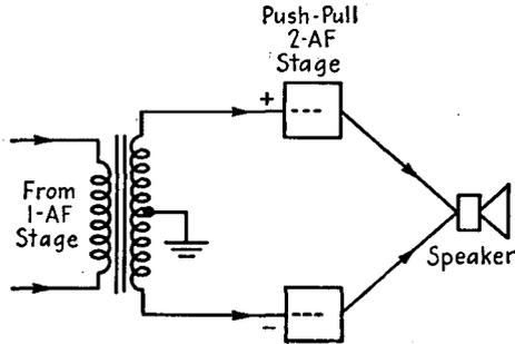
FIG. 21-1.—Block diagram of a push-pull amplifier.
