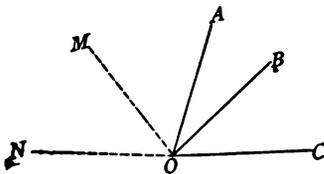
eters is  $0^{\circ} 00' 00''.00$ , and let  $m$  denote the most probable value of  $MOA$ . Then let the three readings on  $A$ ,  $B$ , and  $C$  give the three observation equations
