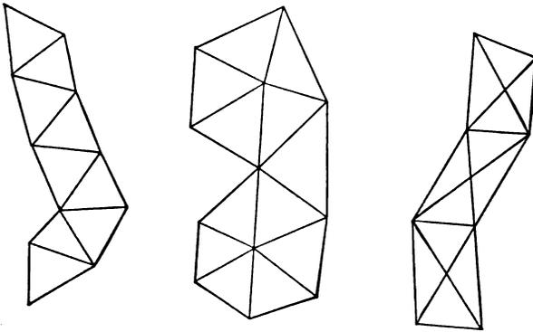
triangulation and the topography of the country will determine the location of the stations and the size of the triangles. A chain net is one suitable for a river survey, a polygonal net where the triangles from one or more polygons is some-
