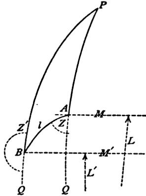
$$L' = L + \delta L, \quad M' = M + \delta M, \quad Z' = Z + 180^\circ + \delta Z. \quad (64)$$
