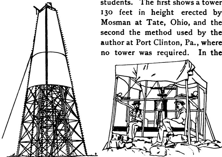
first view the theodolite is not visible, but in the second it is seen mounted upon the tripod. In both views heliotropes for flashing to the adjacent stations may be distinguished. Detailed information regarding the erection of towers will be found in the Report of U. S. Coast and Geodetic Survey for 1882, pages 199-208.
