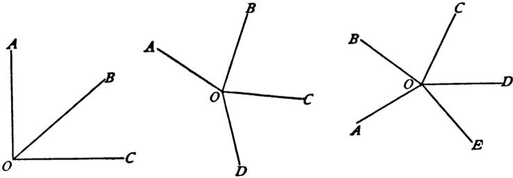
measure all the angles resulting from the combination of the lines two by two. Thus for three lines  $OA$ ,  $OB$ , and  $OC$ , the angles  $AOB$ ,  $AOC$ , and  $BOC$  should be observed; for four lines six angles should be measured, namely,  $AOB$ ,  $AOC$ ,  $AOD$ ,  $BOC$ ,  $BOD$ , and  $COD$ ; in general for  $n$  lines the measurements should be distributed over  $\frac{1}{2}n(n - 1)$  angles. If about 5 series are thought necessary for one inde.
