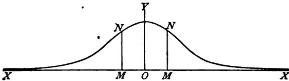
$x$  is zero, that  $y$  becomes very small when  $x$  is very large, and that the same value of  $y$  is given by equal positive and negative values of  $x$ . The figure shows the curve expressed by the equation,  $x$  and  $y$  being parallel to the axes  $OX$  and  $OY$ , and  $OM$  being any error whose probability  $y$  is given by the ordinate  $MN$ .
