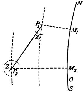
Through  $P_1$  and  $P_2$  let circles be drawn parallel to the central meridian  $NS$ , and let the angle which the line  $P_1P_2$  makes with the circle through  $P_1$  be called  $Z_1$ . Here  $Z_1$  is not strictly an azimuth, and it is best to call it a direction-angle. Similarly, the direction-angle of  $P_2P_1$  at  $P_2$  is called  $Z_2$ . These direction-angles are measured from the south around through the west, north, and east exactly like geodetic azimuths.
