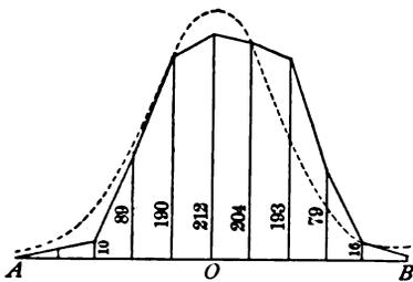
slight preponderance of shots below the middle, and there is reason to believe that this is due to a constant error of gravitation not entirely eliminated in the sighting of the gun. If this series of shots were to be repeated again under exactly similar condi-
