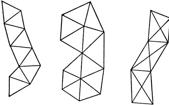
quadrilaterals only, the adjustment of each is made by Art. 80, and the sides then found from the plane angles. If it be made up of triangles, polygons, and quadrilaterals, as is generally the case, the same process may be followed, by starting at the base and treating each part in succession. Lastly the latitudes, longitudes, and azimuths are computed by the method of Art. 66 if the triangulation be a geodetic one, or by that of Art. 19 if it be plane.
