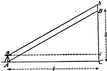
ature and refraction is  $44''$ , so that the vertical angle  $3^{\circ} 07' 59''$  is the value to be used. Then the difference of level between  $a$  and  $b$  is found by the use of the logarithmic tables to be 566.6 feet, and applying the correction for height of instru-
