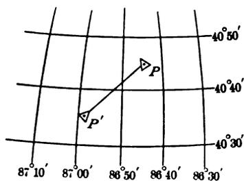
drawn on the polyconic projection method which is explained in Art. 69. Station  $P$  is located at latitude  $40^\circ 45'$  and at longitude  $86^\circ 43'$ , while station  $P'$  is located at latitude  $40^\circ 36'$  and longitude  $86^\circ 58'$ . The straight line, or geodesic, joining the
