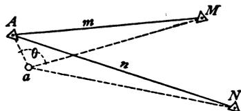
the true angle  $MAN$  from the observed angle  $MaN$ . To do this the distance  $Aa$  must be carefully measured and also the angle  $AaM$ , and the distances  $AM$  and  $AN$  must be found from the triangulation. Let  $Aa = d$ ,  $AaM = \theta$ ,  $AM = m$ ,  $AN = n$ ,  $MaN = a$ , and  $MAN = A$ . Then, as the opposite angles made by the crossing lines are equal,  $A + M$  equals  $a + N$ , and accordingly the required angle is
