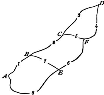
equations. This is perhaps seen more clearly by noting that, if the elevation of one bench be given, the elevations of the five others are to be obtained. In general the number of independent quantities in any net of level lines is one less than the number of benches.
