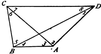
angle is  $A$ , while  $d_1$  and  $d_2$  are those for the triangles whose large angles are  $B$  and  $C$ ; also let  $d_3$  be the discrepancy for the fourth triangle  $CDA$ . Let  $v_1, v_2, \dots, v_8$  be the corrections in seconds to be applied to the observed values. Then the three conditional angle equations are
