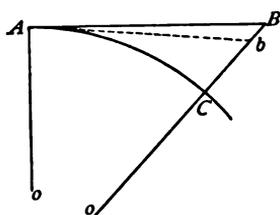
from  $b$  to  $A$ , thus making  $b$  appear at  $B$  to an observer at  $A$ . The deviation due to curvature in the distance  $l$  is hence represented by  $BC$  and that of refraction by  $Bb$ , their difference  $bC$  being the combined deviation; let these be called  $c$ ,  $kc$ , and
