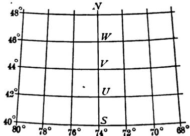
normal to  $NS$ , and on each of these the values of  $x$  and  $y$  are laid off as computed for the latitudes  $42^\circ$ ,  $44^\circ$ ,  $46^\circ$ , and  $48^\circ$ , thus locating six points on each parallel. Through these points curves are drawn and the coordinate system is completed.
