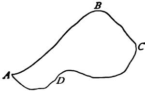
ocean level, the following elevations of other benches are found, and on returning to *A* its elevation is 420.467 feet, showing a discrepancy of 0.150 feet. The distances between the benches being 6, 3, 4, and 2 miles,  $\frac{6}{15}$  of the discrepancy is to be subtracted from the elevation of *B*,  $\frac{3}{15}$  from that of *C*, and so on. This method of adjustment is one that would
