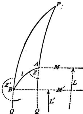
The azimuth of  $AB$  is the angle  $QAB$ , which is called  $Z$ , and the azimuth of  $BA$  is the obtuse angle  $Q'BA$ , which is called  $Z'$ . Let the latitude and longitude of  $A$  be given, together with the length and azimuth of  $AB$ . It is required to find the latitude and longitude of  $B$  and the azimuth of  $BA$ .
