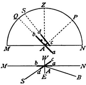
The lower part of the figure is a plan,  $A$  being the place of the instrument,  $NM$  the true meridian,  $W$  and  $E$  the west and east directions,  $AS$  the direction of the sun about 10 o'clock in the morning, and  $AB$  a line whose azimuth is required to be found.
