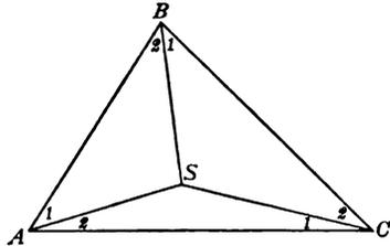
$$BS = AS \frac{\sin A_1}{\sin B_1}, \quad BS = AS \frac{\sin A_2 \sin C_2}{\sin C_1 \sin B_1},$$
