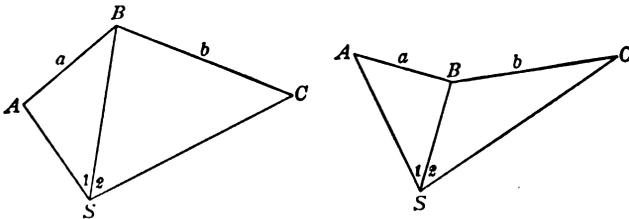
subtended at it by three stations  $A$ ,  $B$ , and  $C$  whose positions are known. It is well to measure the three angles at  $S$  and then by the station adjustment find the most probable values
