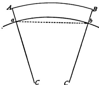
the surface of a spheroid coinciding with ocean level. Thus, if  $l_1$  represent the computed geodetic distance between two stations whose elevation above ocean level is  $h$ , it is plain from (31) that the true distance between those stations is
