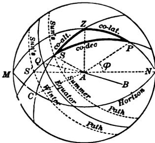
Thus, if  $A$  be any place, represented in the figure by a point at the center of the celestial sphere, the vertical line  $AZ$  determines the zenith  $Z$ . Let  $P$  be the celestial pole and  $N$  the north point of the horizon, then the angle  $PAN$  or the arc  $PN$  is the latitude of the place.
