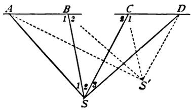
From these angles and the measured distances  $AB$  and  $CD$  the distance  $BC$  is computed in two ways, namely,
