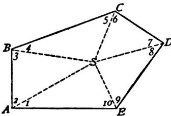
with the line to  $S$  be measured,  $S$  being an unoccupied station. By applying the rule of the last Article it is seen that there are two conditions in the figure adjustment, one angle equation and one side equation. If the
