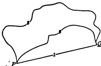
If the precision of the work per mile is the same, the value of  $r$ , being the same for the three lines, then the weights of the three results are to be taken as  $\frac{1}{5}$ ,  $\frac{1}{6}$ , and  $\frac{1}{10}$ . The adjusted elevation of  $P$  above  $Q$  is then found by the rule of Art. 4 to be 37.403 feet.
