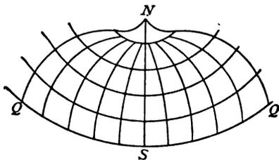
equatorial radius  $a$ , and the radius of any other parallel is  $a \pm d$ , where  $d$  is its distance from the middle parallel. This method gives trapezoids of equal area and an orthographic projection along the middle meridian and parallel, but the shape becomes rather awkward where a large area is represented.
