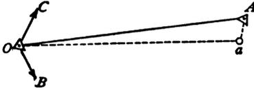
This is called the case of an eccentric signal, and a correction is to be applied to the observed angle to reduce it to
