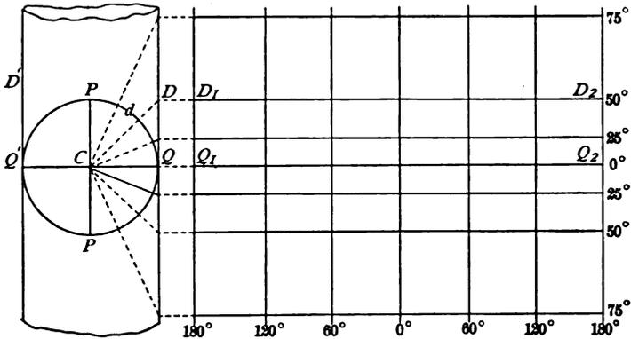
In the case of the spheroid the same principles apply for the construction of a Mercator projection, but the distance of any parallel from the equator will be
