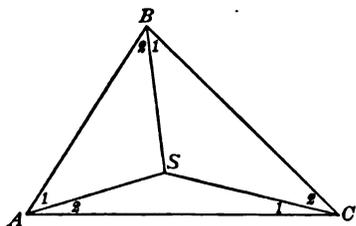
The station adjustment has already been discussed, and now the figure adjustment is to receive attention. This figure adjustment gives rise to conditions of two kinds, called angle conditions and side conditions.
