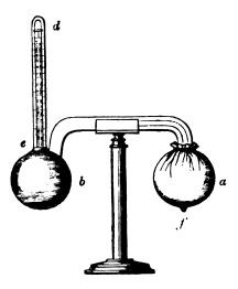
Secondly, I imagined that its sensibility might be increased by extending, at pleasure, the scale of the thermometer de. The divisions of the thermometer included in the glass instrument are necessarily small;
