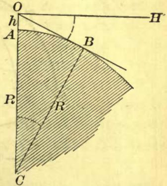
FIG. 3.—Dip of the Horizon.
