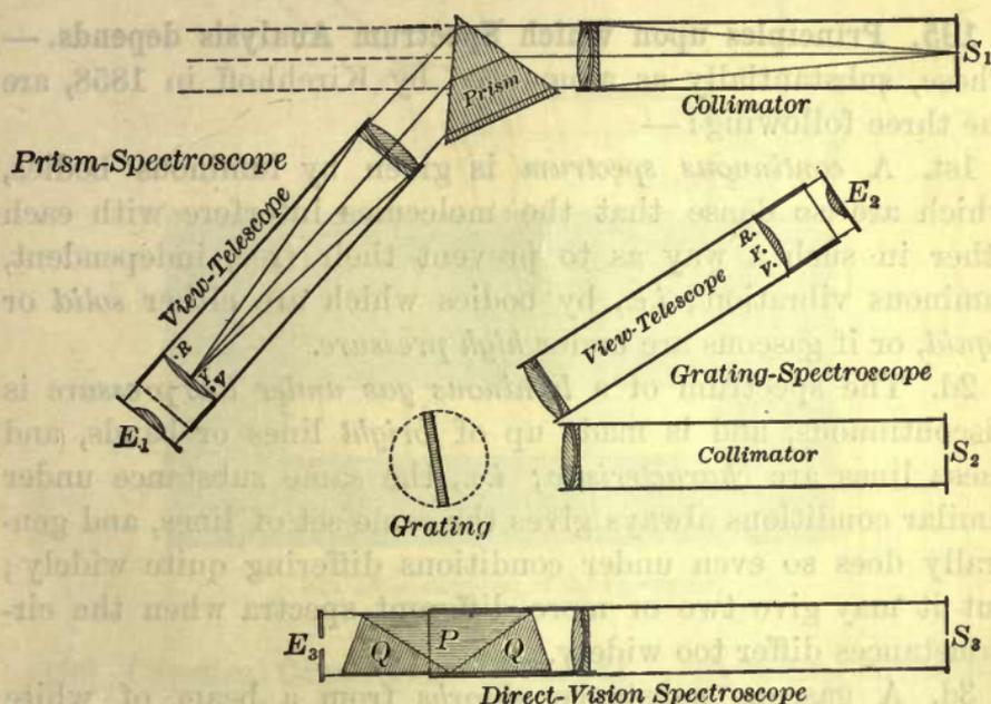
FIG. 52. — Different Forms of Spectroscope.
