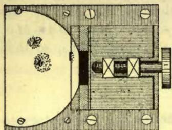
FIG. 129. — Spectroscope Slit adjusted for Observation of the Prominences.
