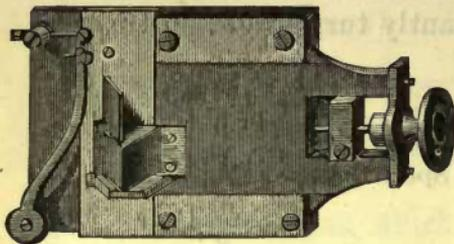
FIG. 54. — The Comparison Prism.
