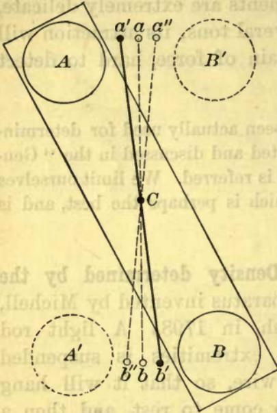
FIG. 20. — Plan of the Torsion Balance.
