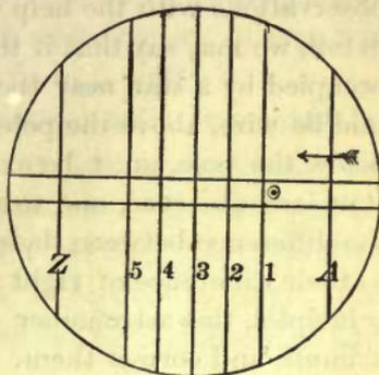
FIG. 151. — Reticle of the Transit Instrument.
