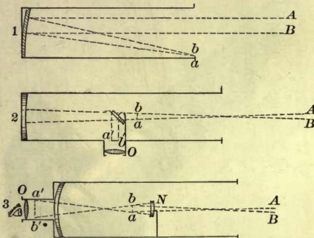
FIG. 145. — Different Forms of Reflecting Telescope.
