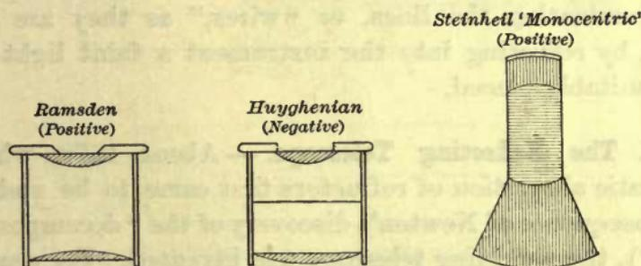
FIG. 144. — Various Forms of Telescope Eye-piece.
