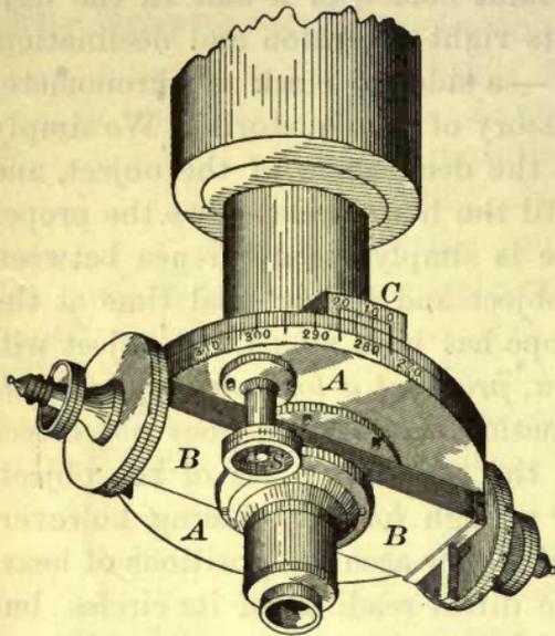
FIG. 148. — The Filar Position-Micrometer.
