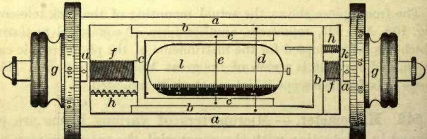
FIG. 149. — Construction of the Micrometer.
