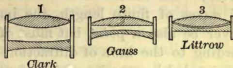
FIG. 143. — Different Forms of the Achromatic Object-glass.
