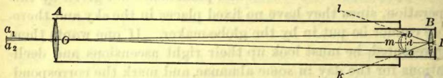
FIG. 142. — The Simple Refracting Telescope.
