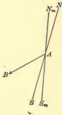
36. To convert magnetic courses into compass courses, or compass courses into magnetic courses, it is necessary to have a list of deviations corresponding to the different directions in which the ship heads. This is determined before the ship leaves port. Deviation acting on the compass needle to deflect it from a *magnetic* N. and S. line, tables of deviation give the amounts of deviation E. and W. of the magnetic north point.
