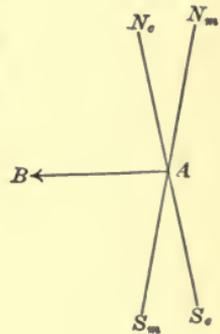
$$\begin{aligned} \text{com. course} &= N_c AB = 80^{\circ} \text{ left of N.} \\ \text{deviation} &= N_c A N_m = 23^{\circ} \text{ left of N.} \\ \hline \text{mag. course} &= N_m AB = 103^{\circ} \text{ left of N.} \\ &= 77^{\circ} \text{ right of S.} \\ \text{mag. course} &= \text{S. } 77^{\circ} \text{ W.} \end{aligned}$$
