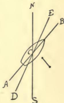
Although leeway is not an error of the compass, the effect of it is the same as if it were, and allowance must be made for it in order to determine the true course of a ship.
