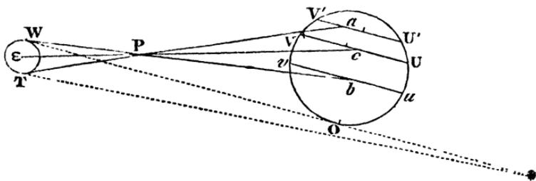
or the time of describing  $VU$ , then the time of describing  $vu$  nearer to the Sun's center than  $VU$ , would be  $T + t$ : of describing  $V'U'$  more remote than  $VU$  from the Sun's center,  $T - t'$ : and accordingly the difference of the durations of the transits seen from  $T$  and  $W$ , would be  $T + t - (T - t') = t + t'$ . This, as it is plain, is entirely the effect of parallax.
