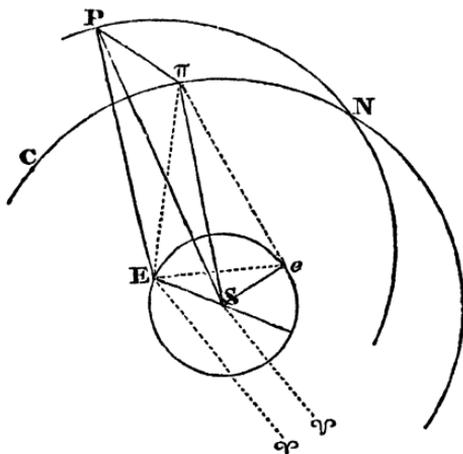
of the planet from the node ; this is technically called the *Argument of the Latitude* ; since it is the quantity, by means of which the latitude may, either be computed (see p. 254,) or, be taken out of the Tables.
