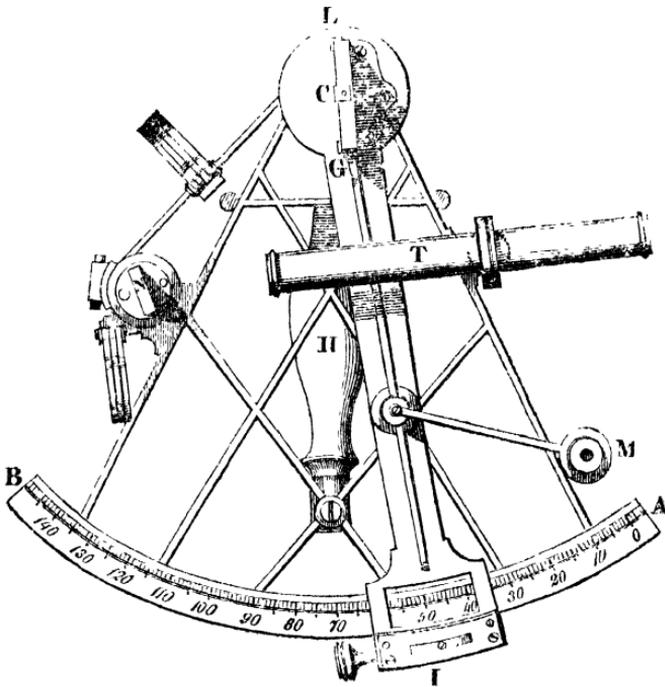
scope *M* moveable about a center, and capable of being adjusted so as to *read off* the divisions on the graduated limb *AB*. The less Figure is intended as a sketch of the larger and for the purpose of explaining its properties.
