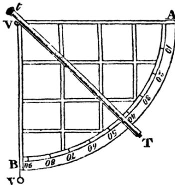
into 90 degrees: each degree into smaller equal divisions: the number of divisions plainly depending on the size of the instrument. *Ti* is a Telescope moveable about a center at *V*: *Vv* is
