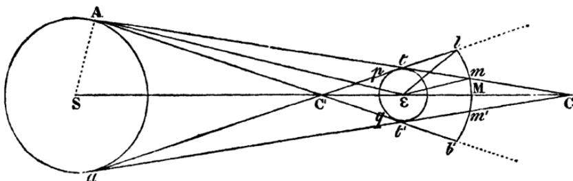
sections of the Sun and Earth, then the triangular space included within  $tC$ ,  $t'C$ , will represent the section of the conical shadow of the Earth. Let  $mMm'$  be part of the Moon's orbit, then the section of the Earth's shadow at the Moon is  $mMm'$ , and its apparent semi-diameter at the Earth, which we have to estimate, is the angle  $mEM^*$ .
