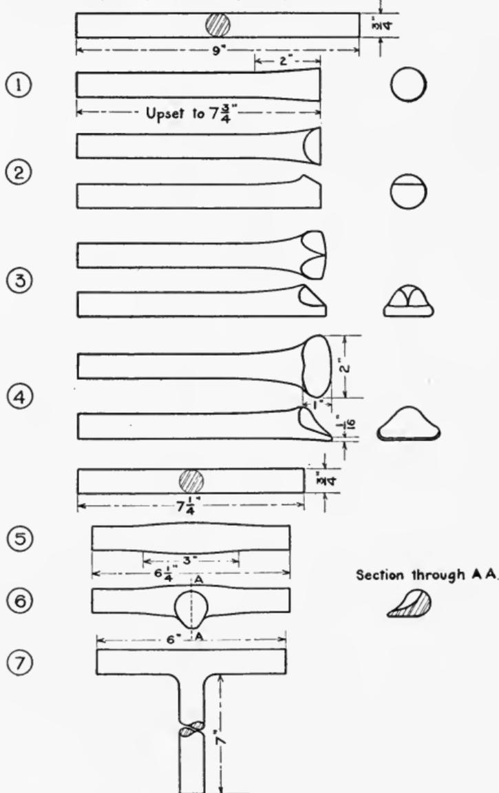
smoothed between top- and bottom-swages, and the scale removed with a file. The ends are then trimmed off, making the dimensions of the T as shown at 7.
