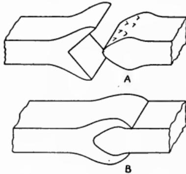
Fig. 42. SPLIT WELD FOR HEAVY STOCK.
