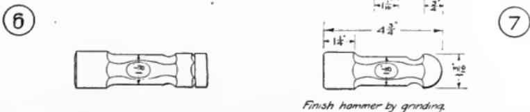
sides, in order to insure a square end. Draw-out the face, swage it, and trim it with a hot chisel. The peen should then be cut to length, and the corners cut off. It is rounded in a bottom-swage. The reason for finishing the face before the peen is that it is hard to hold the peen with a pair of tongs.
