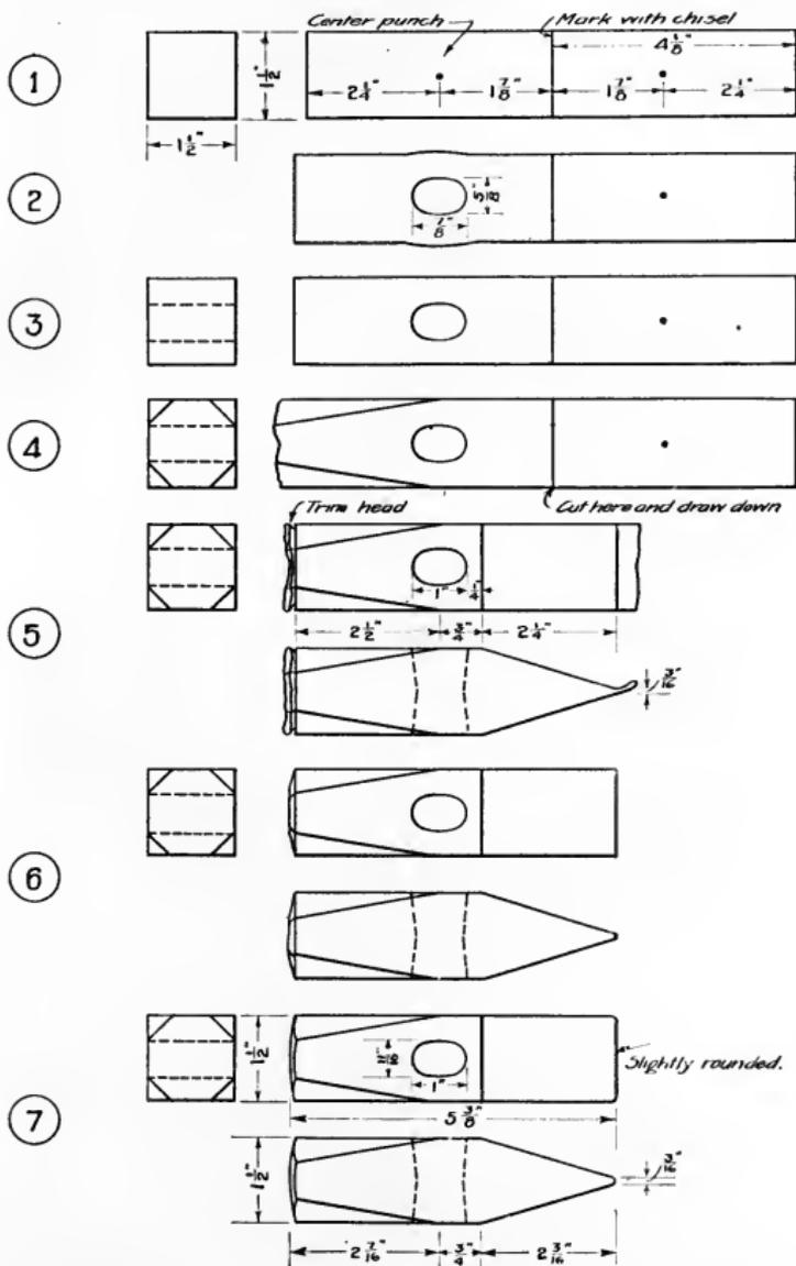
was done with the cold chisel. When it has cooled enough, the peen is hardened in the same manner, care being taken not to cool the stock around the eye. While cooling the peen, water should be allowed to drip on the center of the face. This prevents the colors from running down before the peen has been cooled enough, and insures a uniformly hardened face. If the face were cooled by merely dipping it in water, the outside edges would harden faster than the center and be more likely to crack.
