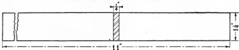
Width of end of scarf should be slightly less than width of stock.
