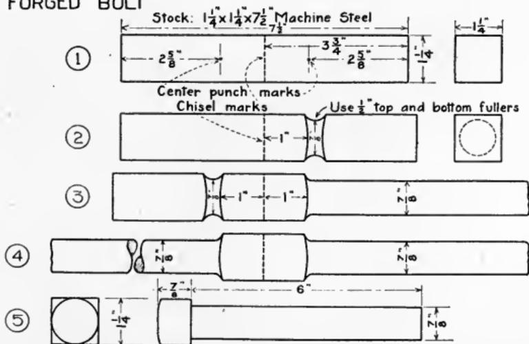
STEP SIX.—Heat the head slowly, to prevent the collar from burning, and weld it by hammering on all four sides. Finish it in a heading-tool in the same manner as an upset head.
