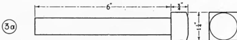
Stock for hexagonal head bolt:  $\frac{3}{4}$ " x 9" round machine steel
