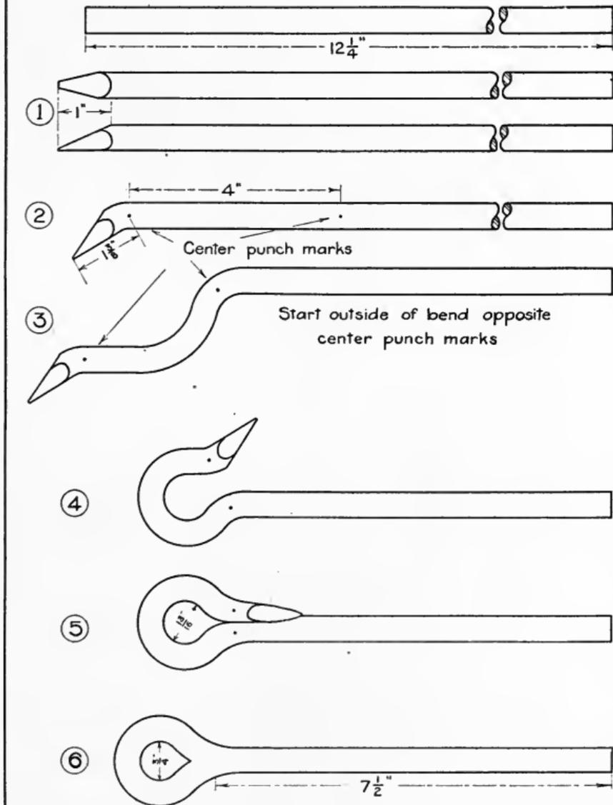
slightly larger than the finished hole, in the eye and bring the scarf and shank together, as at 5.
