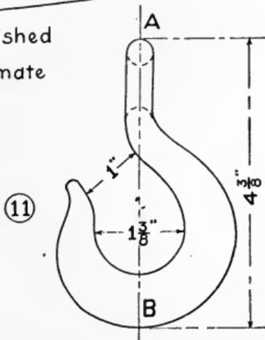
Line AB thru eye should also pass thru center of hook
