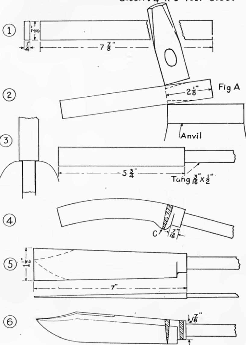
**HARDENING.**—The knife is heated slowly in a piece of pipe in the same manner as the tap. When it has reached the refining heat it is dipped in fish oil, the back or thick edge first, and cooled quickly.
