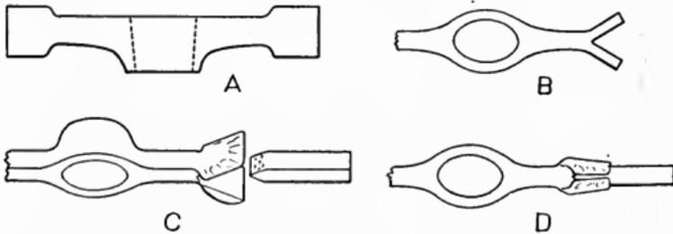
Fig. 43. WELDING TIP ON A PICK.
