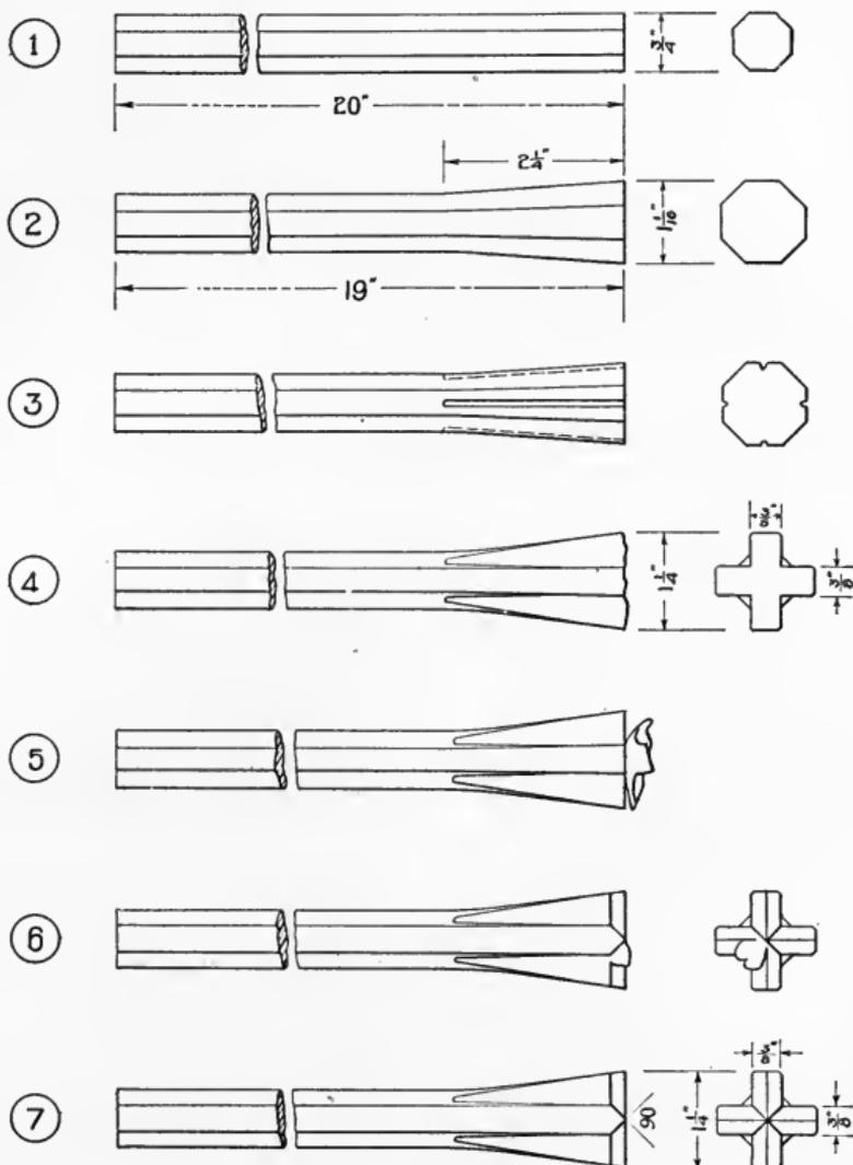
a square set-hammer. Trim off the end of the drill with a very thin hot chisel, making it square, as shown at 5.
