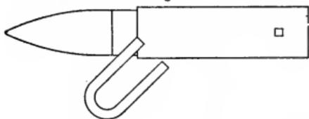
it points to the left, the scarf is left-hand and is harder to weld. The link should be shaped so that the end to be welded is narrower than the other. The stock is then less liable to be hammered small on either side of the weld, and the semi-circular end will be about the right size when the weld is finished.
