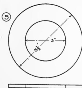
hand-hammer. Finish the edges on the horn, then smooth the sides with a flatter. The ring should be made circular on a cone, and the scale removed with a file.
