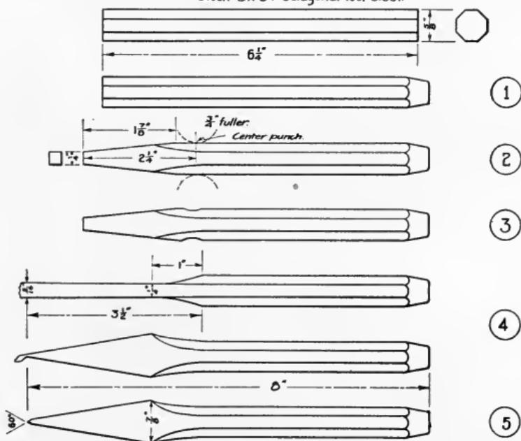
Test the chisel by chipping a piece of cast iron. If the cutting edge is too soft it should be rehardened at a higher temperature; while if it breaks, showing a coarse grain, it should be rehardened at a lower temperature.
