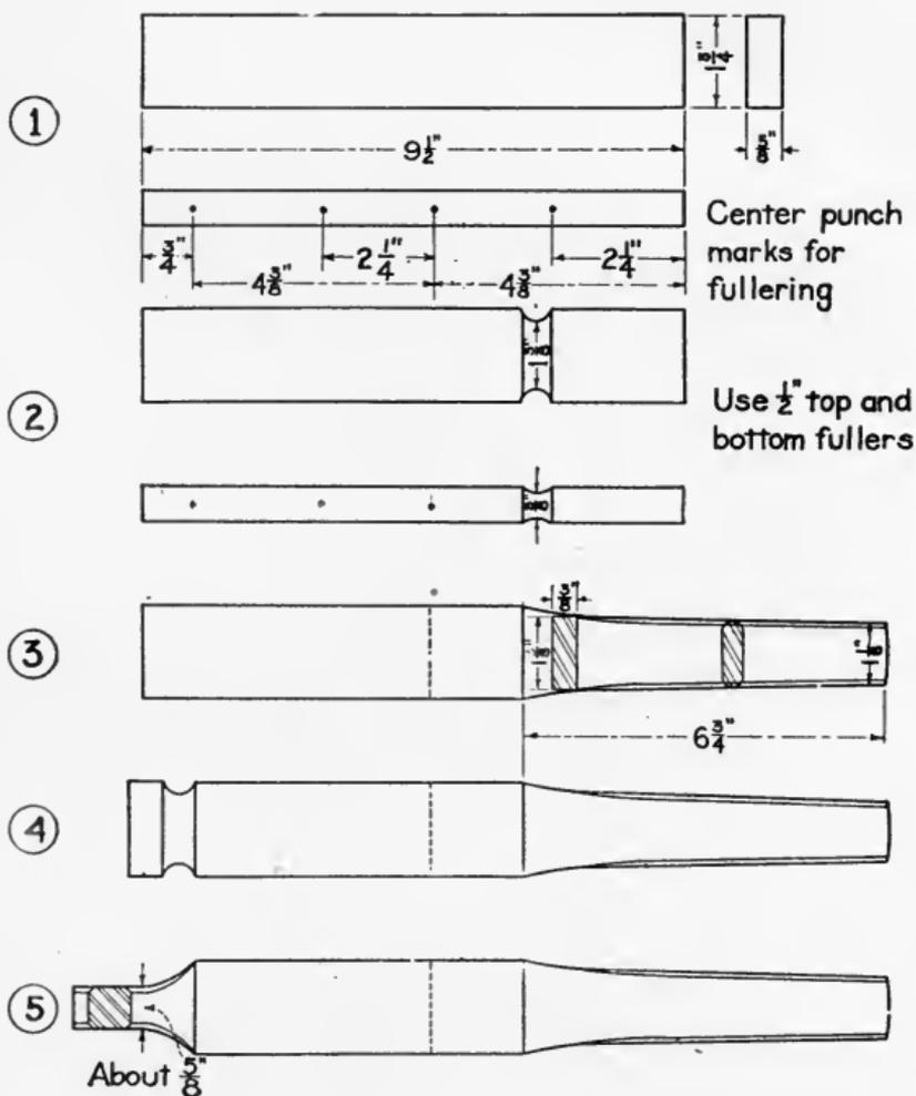
the jaws of the tongs from being caught between the dies. It is therefore best to use a piece of stock  $9\frac{1}{2}$  inches long. This will give enough material for two wrenches, with an allowance for a short tong hold. Remember to use hollow-bit tongs. Flat-jawed tongs are unsafe.
