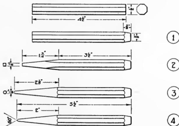
tool occurs at or near the tip. Trim off the end with a hot chisel, and bend it up slightly, as shown.
