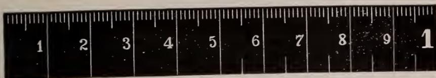
10-centimeter rule. The upper edge is in millimeters, the lower in centimeters and half centimeters.
