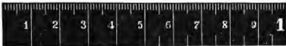
10-centimeter rule. The upper edge is in millimeters, the lower in centimeters and half-centimeters.
