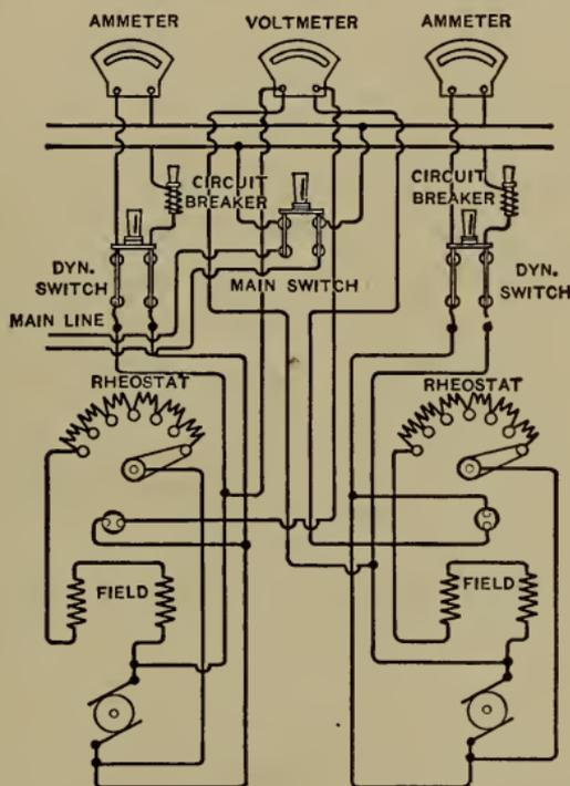
FIG. 61.—Diagrammatic Connections of Two Shunt Dynamos in Multiple.
