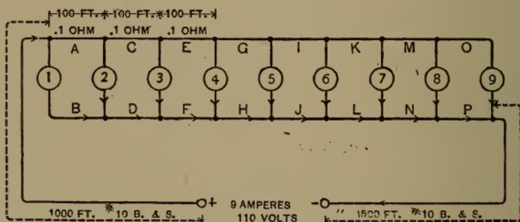
FIG. 6.—Wiedemann System of Wiring.
