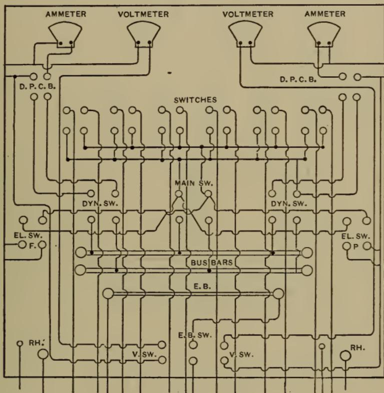
FIG. 70.—Back View of Switchboard, Showing Connections to Equalizer Bar, Switches and Meters.
