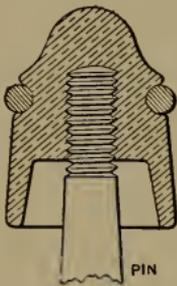
FIG. 85.—Single Petticoat Insulator.
