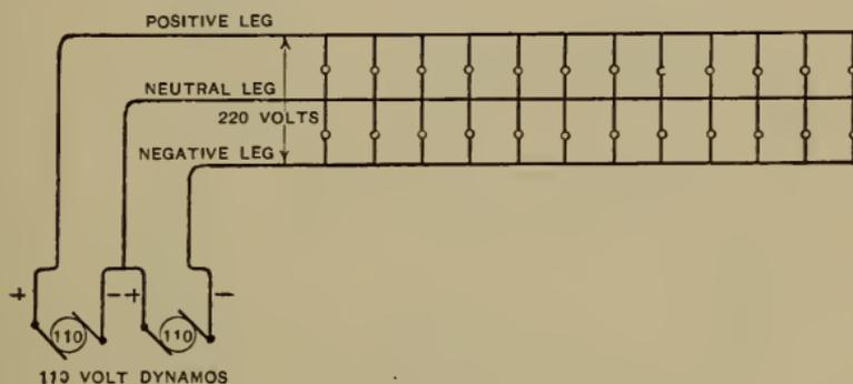
FIG. 32.—The Three-wire System Balanced.
