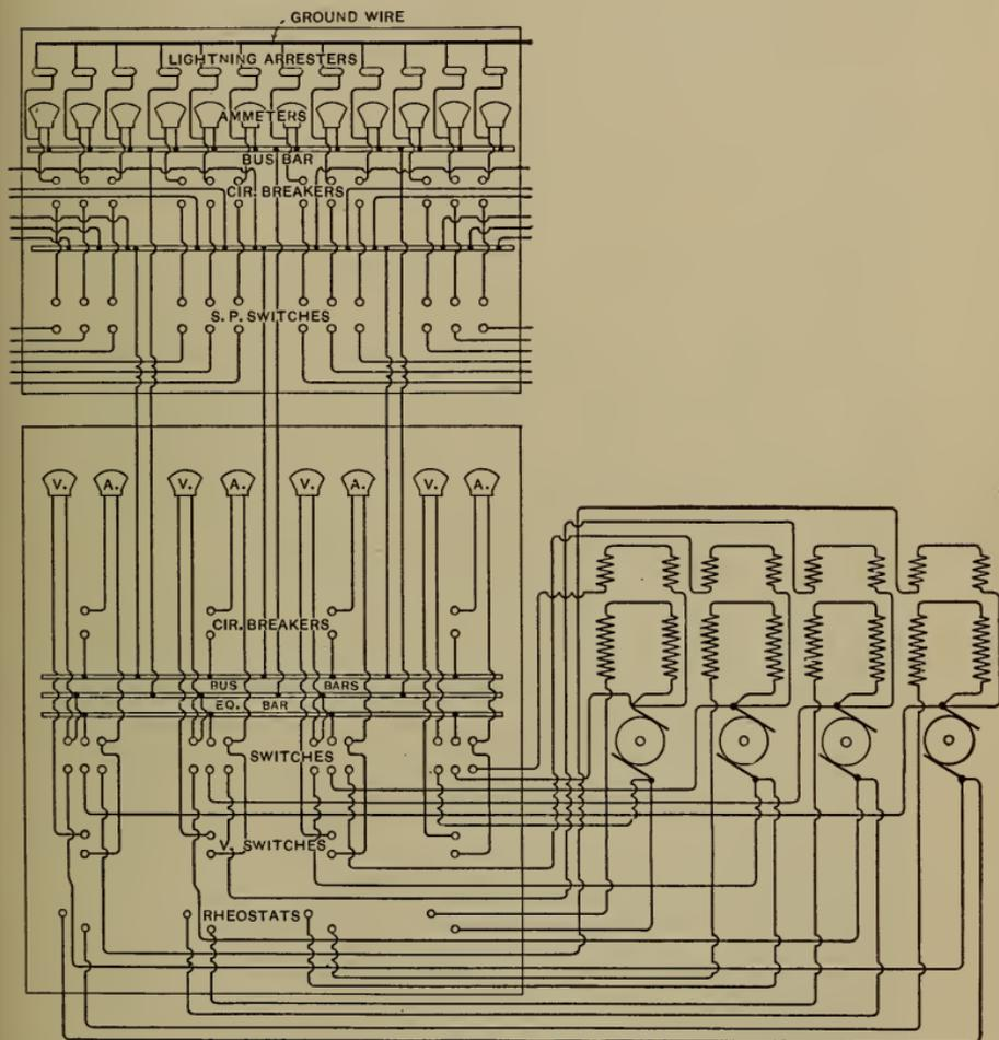
FIG. 81.—Back View of Generator and Feeder Switchboard, Showing Dynamos in Multiple.
