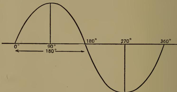
FIG. 94.—The  $360^\circ$  Representing a Complete Cycle.
