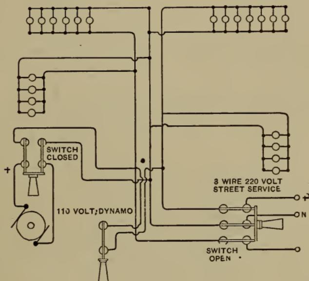
FIG. 34.—Combination of Two and Three-wire System for Protection Against Break-down of Private 110-Volt Two-wire System.
