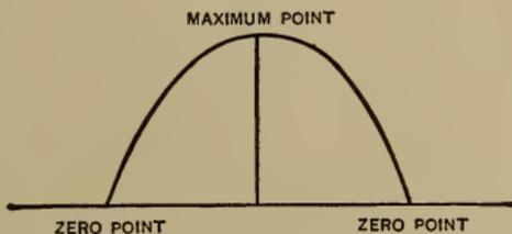
FIG. 90.—Curve Showing the Rise from and Fall to Zero in a Single Wave of E M F.
