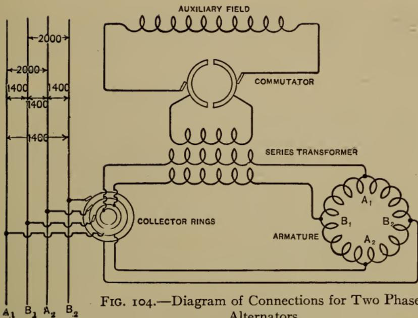
FIG. 104.—Diagram of Connections for Two Phase Alternators.
