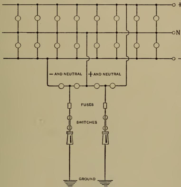
FIG. 84.—Ground Detector for Three-wire System.
