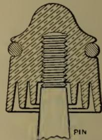
FIG. 87.—Triple Petticoat Insulator.
