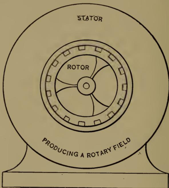
FIG. 97.—Elements of an Induction Motor.
