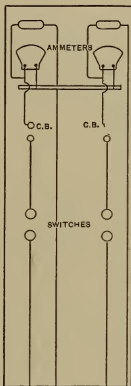
FIG. 76.—Feeder Panel
