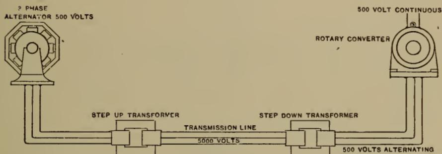
FIG. 100.—Elements of a Power Transmission Plant.
