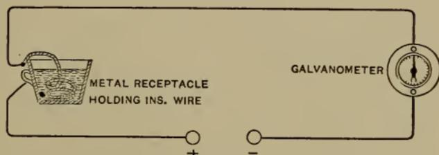
FIG. 27.—Connections for Second Reading.
