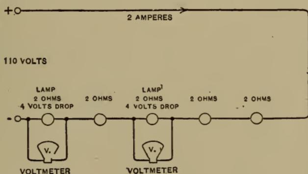
FIG. 2.—Lamps in Series, 4 Volts per Lamp.
