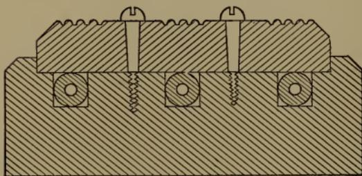
FIG. 46.—Moulding Carrying Wires.
