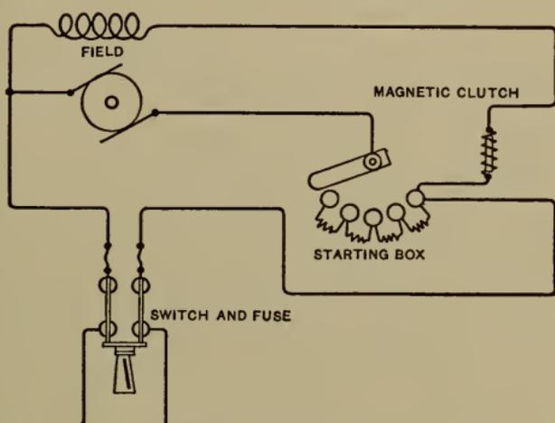
FIG. 40.—Practical Connections of a Shunt Motor.
