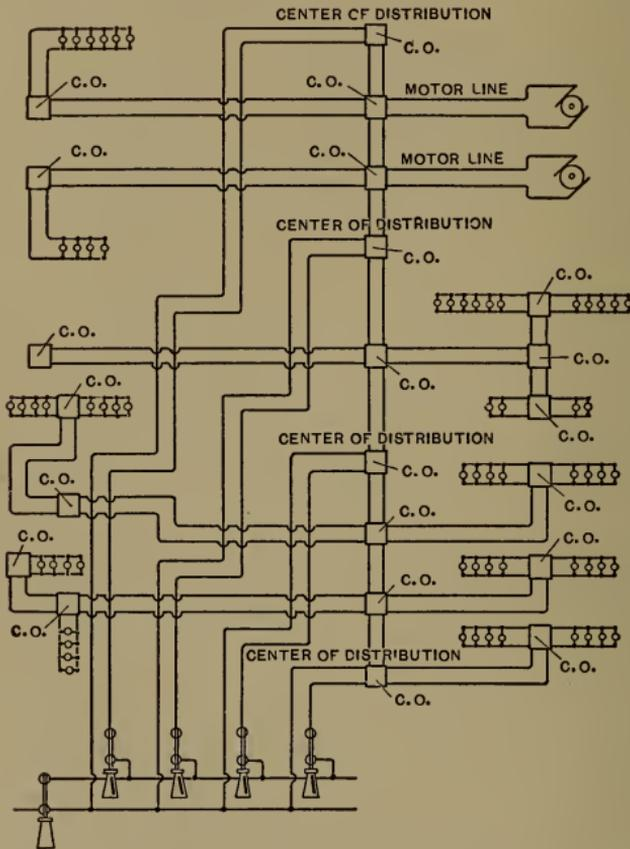
FIG. 17.—Four Main Centers of Distribution and Sub-centers.
