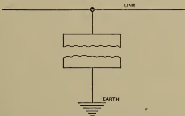
FIG. 82.—Principle of the Lightning Arrester.
