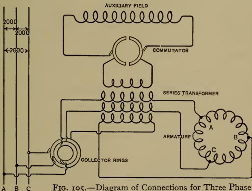
FIG. 105.—Diagram of Connections for Three Phase Alternators.
