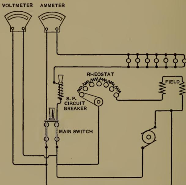
FIG. 59.—Connections and Accessories of a Shunt Wound Dynamo.
