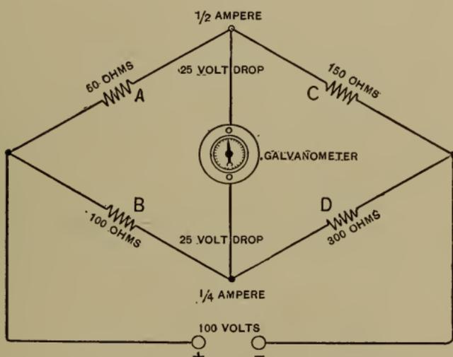
FIG. 22.—Calculating the Drop in a Bridge.
