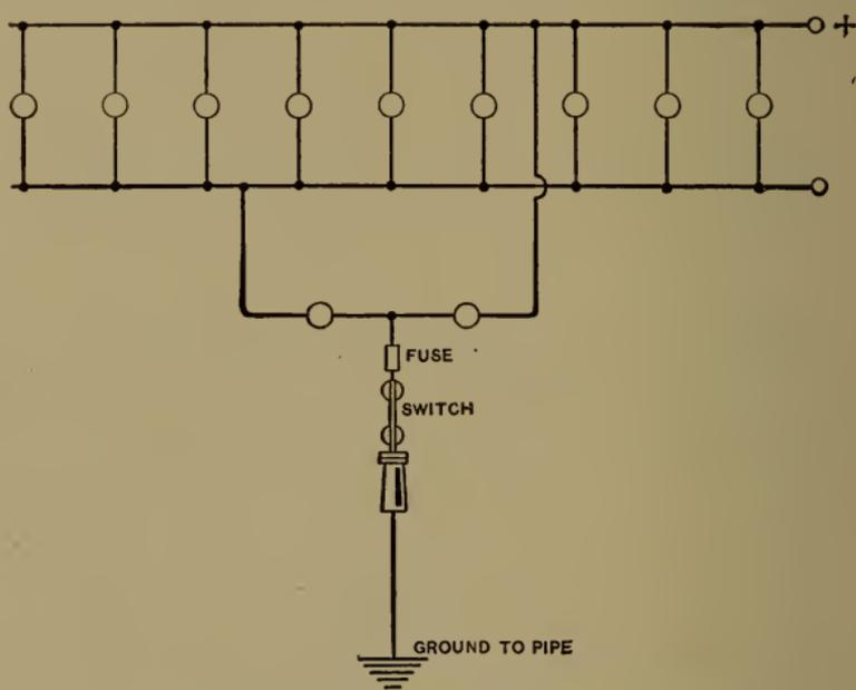
FIG. 83.—Ground Detector for Two-wire System.
