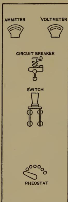
FIG. 78.—Generator Panel (One Circuit).
