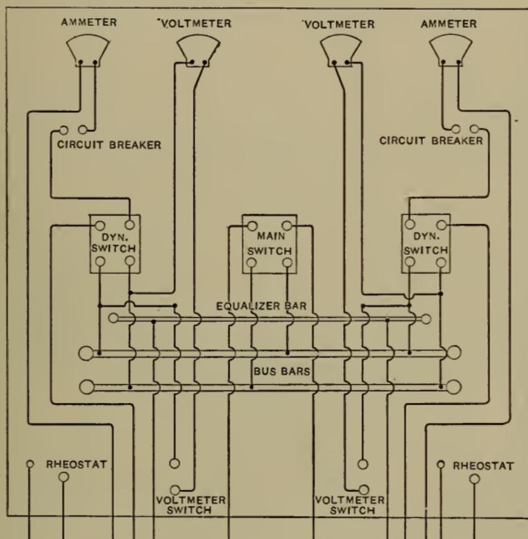
FIG. 68.—Back View, Showing Wiring Connections of Two Compound Wound Dynamos.
