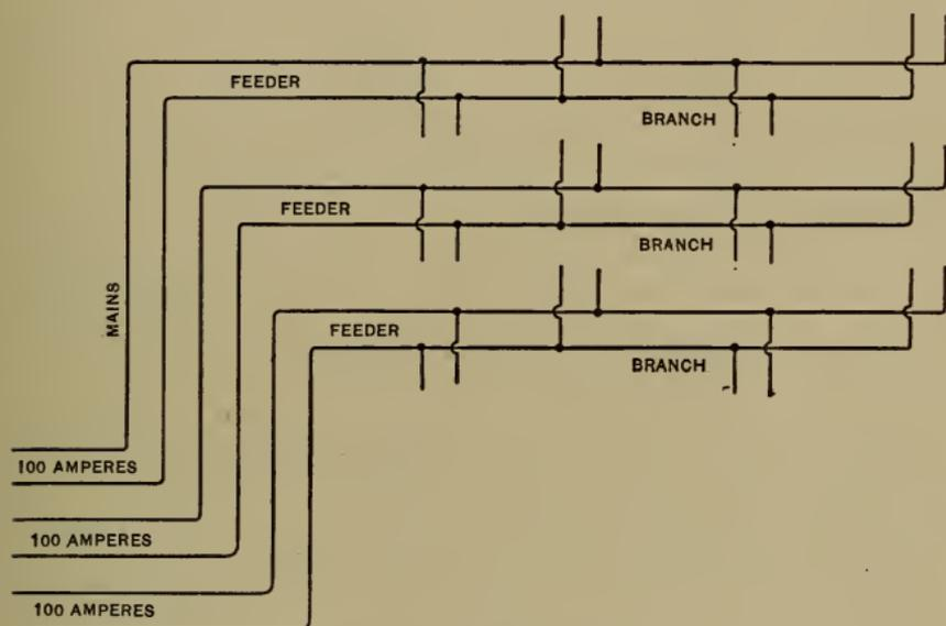
FIG. 11.—System with Individual Mains.
