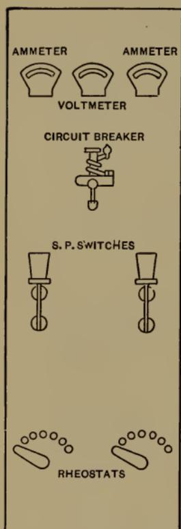
FIG. 77.—Generator Panel (Two Circuit).
