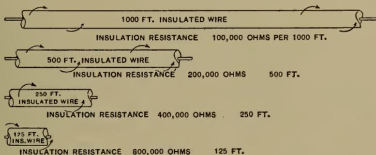
FIG. 24.—Insulation Resistance of Various Lengths of Wire.
