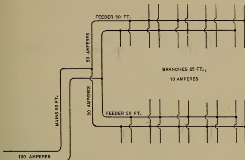
FIG. 12.—Wiring System for Two Floors.
