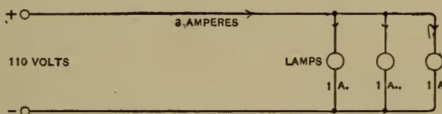
FIG. 4.—Incandescent Light System, Multiple Wiring.
