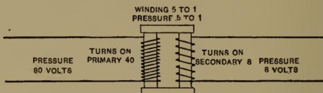
FIG. 101.—Principle of Transformer Winding.
