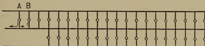
FIG. 29.—The Three-wire System Unbalanced, Showing the Use of Neutral Wire with Respect to Three Lamps.
