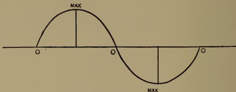
FIG. 92.—Curve Showing a Complete Cycle of EMF.
