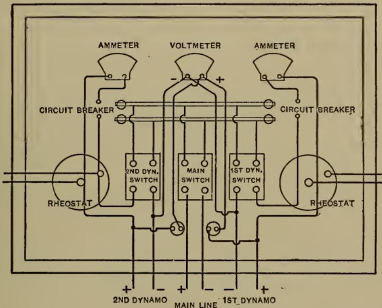
FIG. 63.—Back View of Wiring Connections of Two Shunt Dynamos in Multiple.
