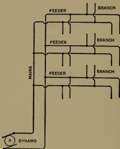
FIG. 10.—Elements of a Wiring System.
