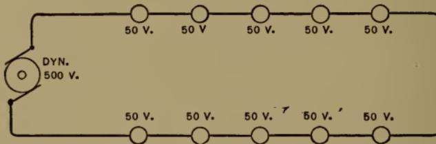
FIG. 3.—High Tension Arc Light System, Series Wiring.
