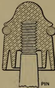
FIG. 86.—Double Petticoat Insulator.
