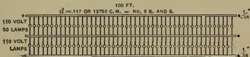
FIG. 31.—Three-wire System. Size of Copper Wire. Transmitting the Same Power, 2 Per Cent. Drop.
