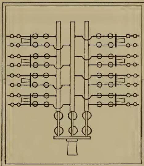
FIG. 58.—Panel Board for Three-wire System.
