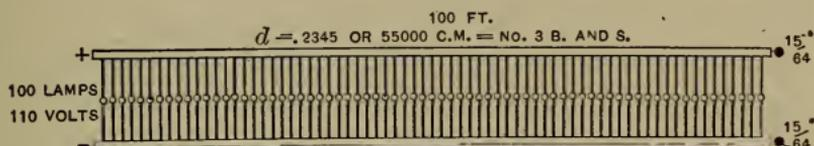
FIG. 30.—Two-wire System. Size of Copper Wire. Lighting 100 16 Candle Power Lamps, 2 Per Cent. Drop.
