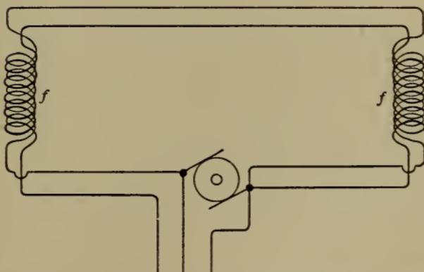
FIG. 37.—Connections of a Differentially Wound Motor.
