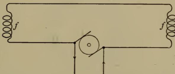
FIG. 36.—Connections of a Shunt Wound Motor.
