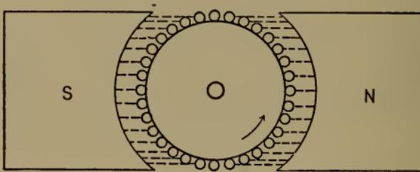
FIG. 38.—Conductor Cutting Lines of Force.
