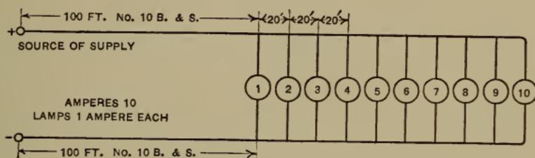
FIG. 5.—Analysis of a 10 Lamp Circuit.
