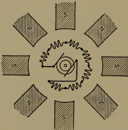
FIG. 42.—Elements of an Alternator.
