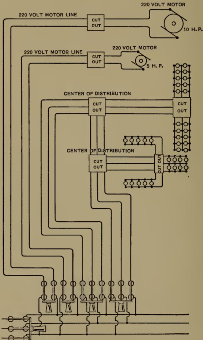
FIG. 33.—Three-wire System with Two Centers of Distribution
