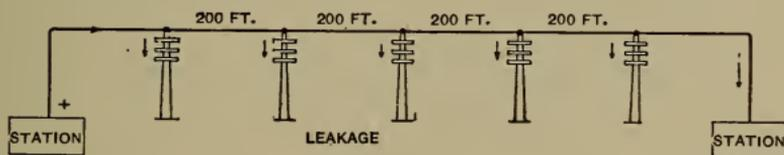
FIG. 25.—Conditions Existing in a Long Distance Line.
