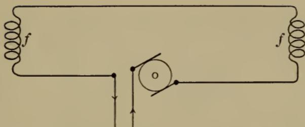
FIG. 35.—Connections of a Series Wound Motor.
