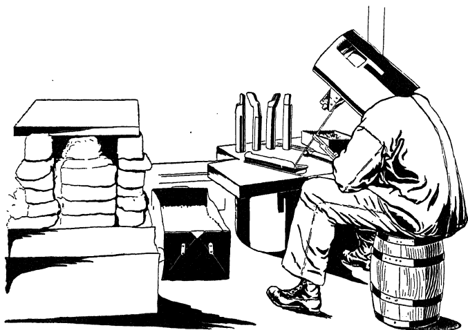
FIG. 147.—Welding High-Speed Tips Onto Mild Steel Shanks.
