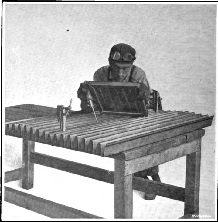
Fig. 4. Arc Welding of Corrugated Sheet Steel for Small Transformer Tanks, using Carbon Electrode
