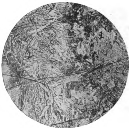
Fig. 21. Another Photomicrograph showing Joint between Welding Metal and Plate
