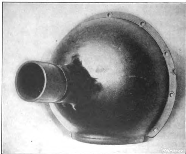
Fig. 8. Tubing welded to a Stamping; Weldings of this Character can easily be handled on Butt-welding Machines especially designed for this Work
