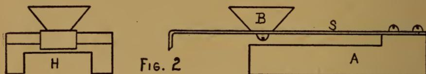
shown enlarged in Fig. 2. The body of the key is made from a block of wood  $2\frac{1}{2}$  inches long,  $1\frac{3}{4}$  inches wide, and  $\frac{3}{4}$  inch thick. It is hollowed out on the under side as shown at H, so that it will fit snugly over the yard stick, and slide easily along the latter. On account of the different width and thickness of various yardsticks, it is impossible to give dimensions for the slot shown at H, but the amateur can easily arrange this.
