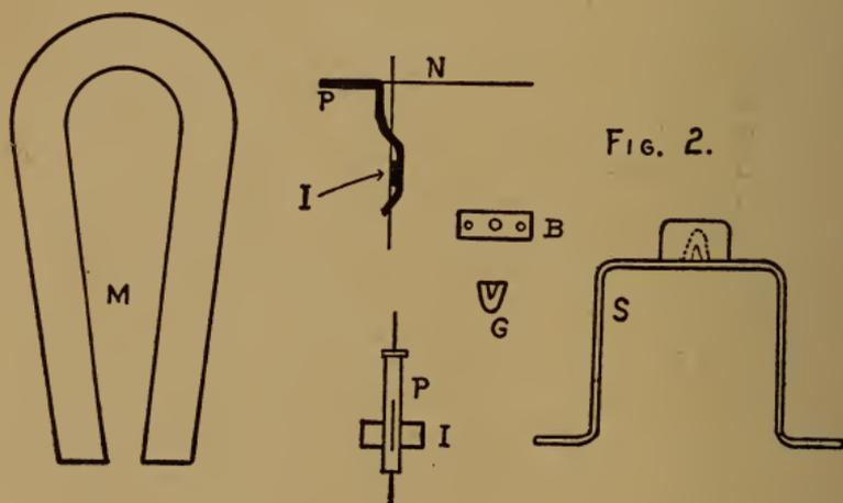
is bent over at right angles at a distance of 5-16 inch from the upper end of the needle. The object of this bend is two-fold. First, it is to be used to support the pointer N by being bent around the latter, and for this reason the strip at this point should be cut rather wide, say  $\frac{1}{8}$  inch. Second, the weight of the projecting part of the strip is designed to counteract the weight of the pointer so as to form a moving system which will be nicely balanced.
