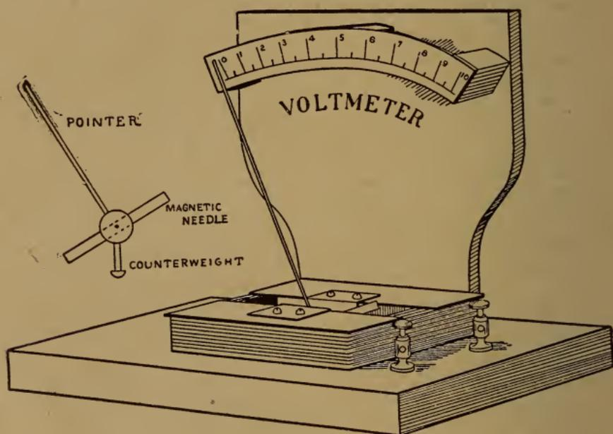
To the magnetic needle thus mounted a pointer 3 inches long is to be attached at right angles to the needle. The best material of which to make this pointer is a firm, hard straw taken from an ordinary broom. Straighten it by rubbing between the fingers, bore a very small hole in one of the wooden clamps which hold the piece of watch spring to the piece of needle, insert the pointer in this hole, and fasten with a bit of glue. The pointer should be straight, and should be at
