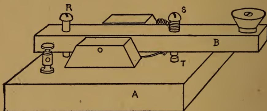
ator, who works a “key” so-called, which is simply an instrument for opening and closing, with accuracy, an electric circuit. All that we shall have to do to make our set complete is to make this key.
