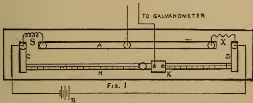
22 German silver or iron wire about a yard long, an ordinary wooden yardstick, a strip of brass or copper 4 feet long,  $\frac{1}{2}$  inch wide, and at least  $\frac{1}{32}$  of an inch in thickness, and five ordinary binding posts.
