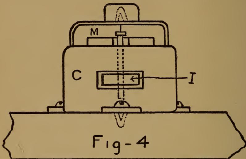
voltmeter. In order to measure the deflection of the pointer a circular scale cut from a piece of stiff Bristol board is mounted at S, by being glued firmly to the top of the magnet, the pointer being so adjusted that it is about 1-16 inch above the scale. In our next chapter an explanation of the method of calibration will be given.
