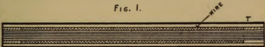
but securely insulated from both. In our coil, the principal difficulty will be to properly insulate the secondary coil, against the high voltage generated within itself.
