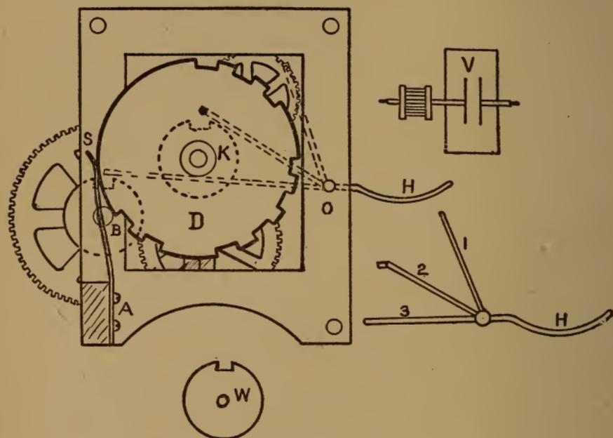
Clockwork Mechanism of Fire Alarm
