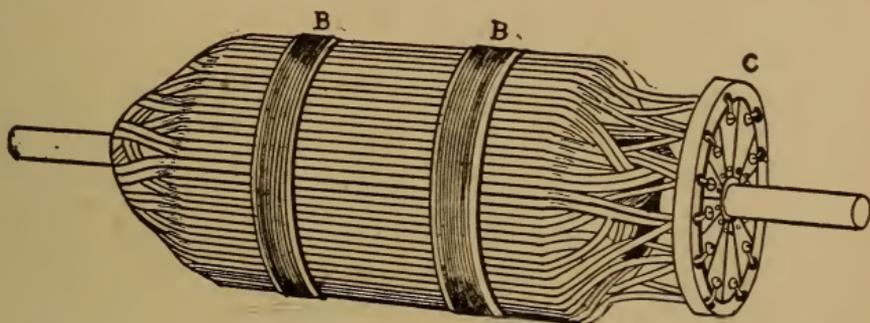
ARMATURE AND COMMUTATOR
