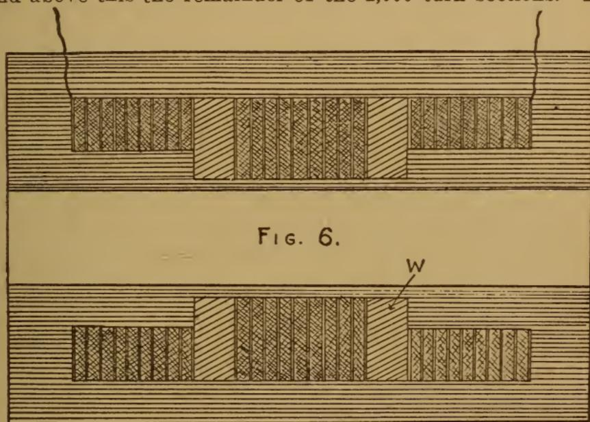
wooden rings used should be thoroughly dried in an oven and then well soaked in boiling hot paraffin wax before being used.
