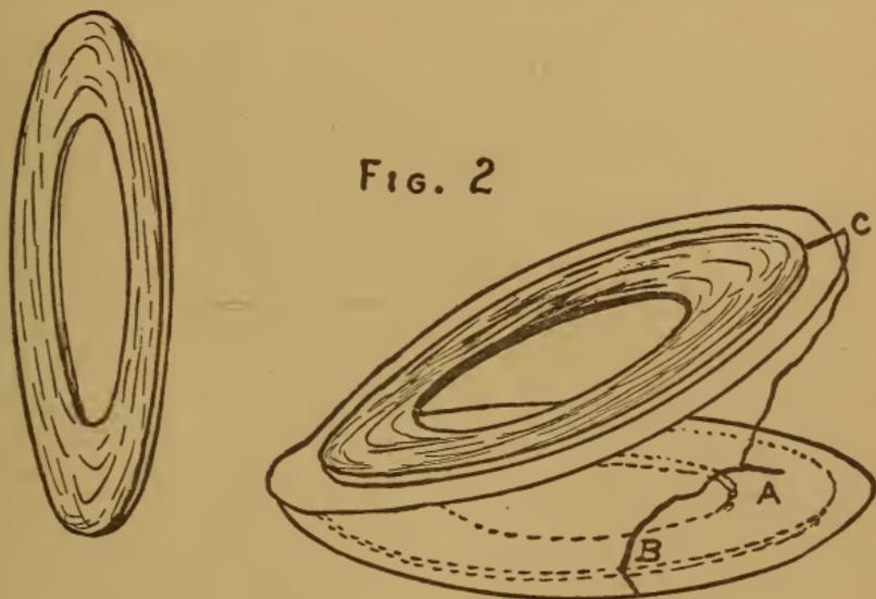
of a very great number of turns of fine wire. Each turn of the secondary has generated within it an electromotive force, and as the latter must be very high, this necessitates a large number of turns.
