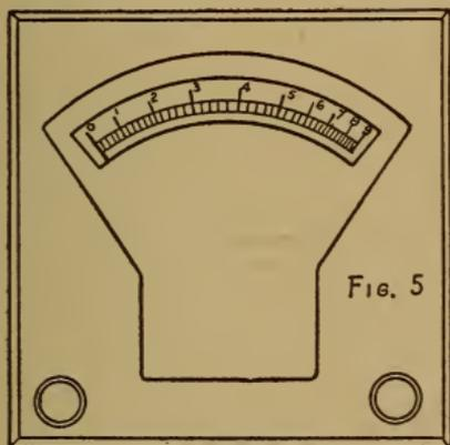
The instrument as described may be used as a voltmeter or as an ammeter according to the method of connection. In either case, for the purpose of calibration, a standard instrument is almost necessary—that is to say, some instrument whose readings are known to be approxi-
