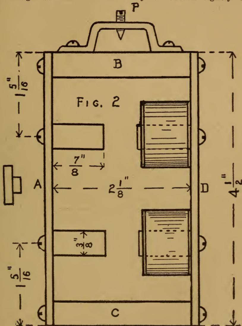
the circular iron cores, to form heads to contain the wire to be wound upon the cores.
