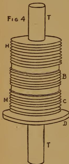
Take a piece of board about  $\frac{7}{8}$  inch thick, and cut a circular piece  $4\frac{1}{4}$  inches in diameter. Through the center bore a hole, which shall be large enough to admit the pasteboard tube containing the primary, and make a tight fit. This piece of wood is seen at D in Fig. 4, with the tube projecting at T for a distance of three inches.
