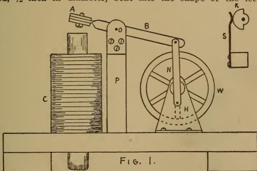
U, each of the arms being  $3\frac{1}{2}$  inches long, measured from the extreme bottom. On each arm wind a coil of insulated wire, so as to form a bobbin 2 inches long and  $1\frac{1}{4}$  inches in diameter. These had better be made of number 24 double cotton covered magnet wire of which about 4 ounces will be required. Carefully insulate the iron core by a layer of paper,
