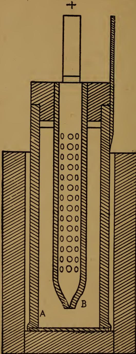
the latter will be held firmly in the block. Now immerse the wooden block after the smaller tube is in place, in smoking hot paraffine wax, leaving it there until the wood has become thoroughly saturated with the hot wax. This is to protect the wood from the action of the acid. Do not get any wax on the lower part of the lead tube.
