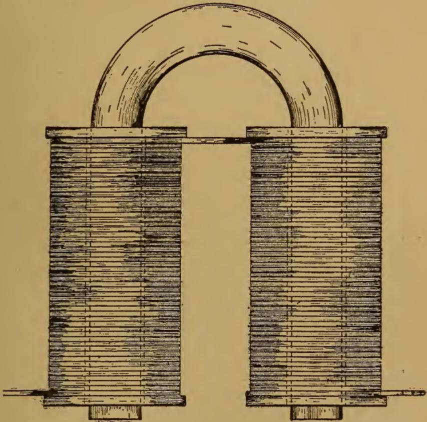
On each spool wind nine layers of No. 18 double cotton covered magnet wire. Be sure and wind each layer evenly and tightly, as this adds much to the appearance of the finished coil. When wound, slip the two spools of wire upon the iron core, and wedge them tightly in place. Connect one end of the first coil
