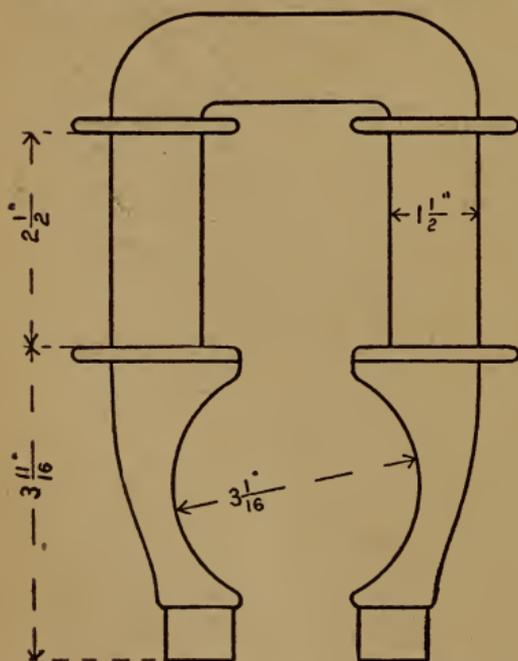
armature space should be 3-16 inches. Next, how large should the core of the field magnet be? This will depend upon the strength of magnetic field that we are to force through it. There is a definite relation between the strength of magnetic field, the speed, the electro-motive force and the conductors on the armature. In every dynamo, the product of the number of conductors on
