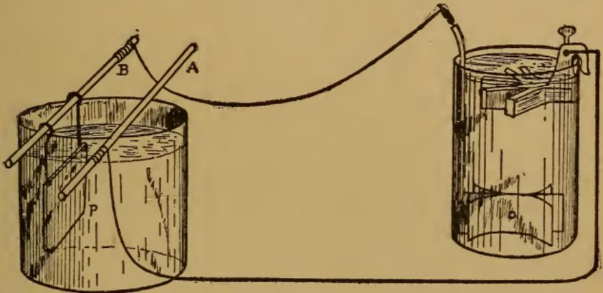
to the other, the solution will be broken up by the action of the current, and a portion of the metal formerly held in solution will be deposited upon the plate where the current leaves the liquid. Thus if a copper and lead plate dip into a solution of copper sulphate, and an electric current be sent through the solution from the copper to the lead plate, copper will be taken through the solution, and deposited upon the lead plate.
