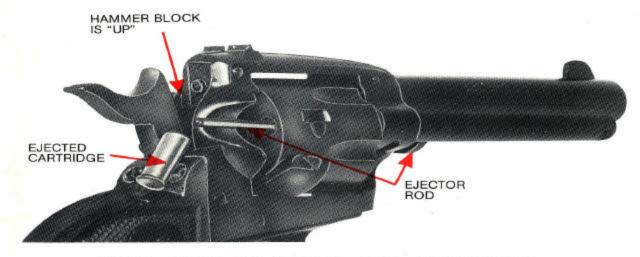
Line up chamber with ejector rod, push ejector rod back through chamber to push out cartridge.
