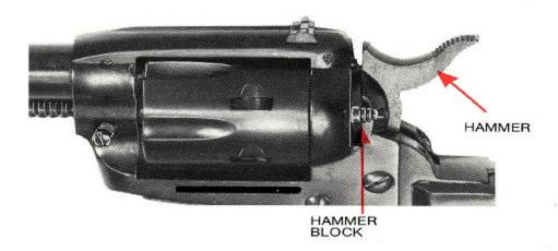
Do not disengage Hammer Block until aiming at target, ready to shoot.
