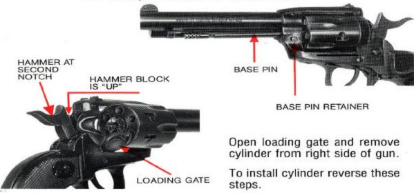
Before loading, test base pin by pulling it forward without pressing base pin retainer. If installed correctly you should not be able to pull it out.
