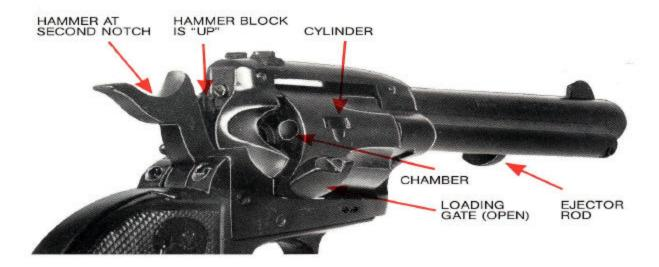
DO NOT EVER carry a live round (loaded cartridge) in the chamber lined up with the hammer-firing pin-barrel, even if the Hammer Block is engaged. Keeping an empty chamber in line with the firing pin is good insurance against any kind of accidental firing.
