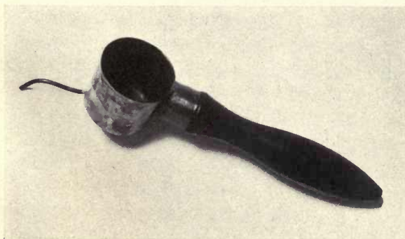
FIG. 24—AMERICAN MODIFICATION OF JAVANESE TJANTING
