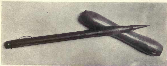
FIG. 22—"WAX PENCIL" MODEL OF TJANTING
