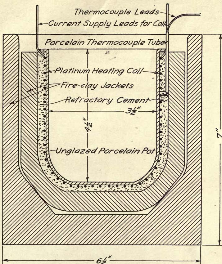
FIG. 3. DETAIL OF POT, RESISTOR, AND INSULATION
