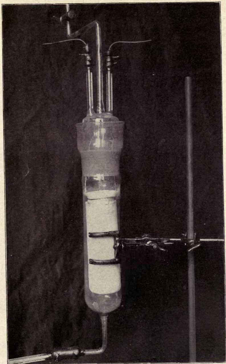
FIG. 6. APPARATUS FOR MEASURING AND ANALYSING THE DISSOLVED GASES
