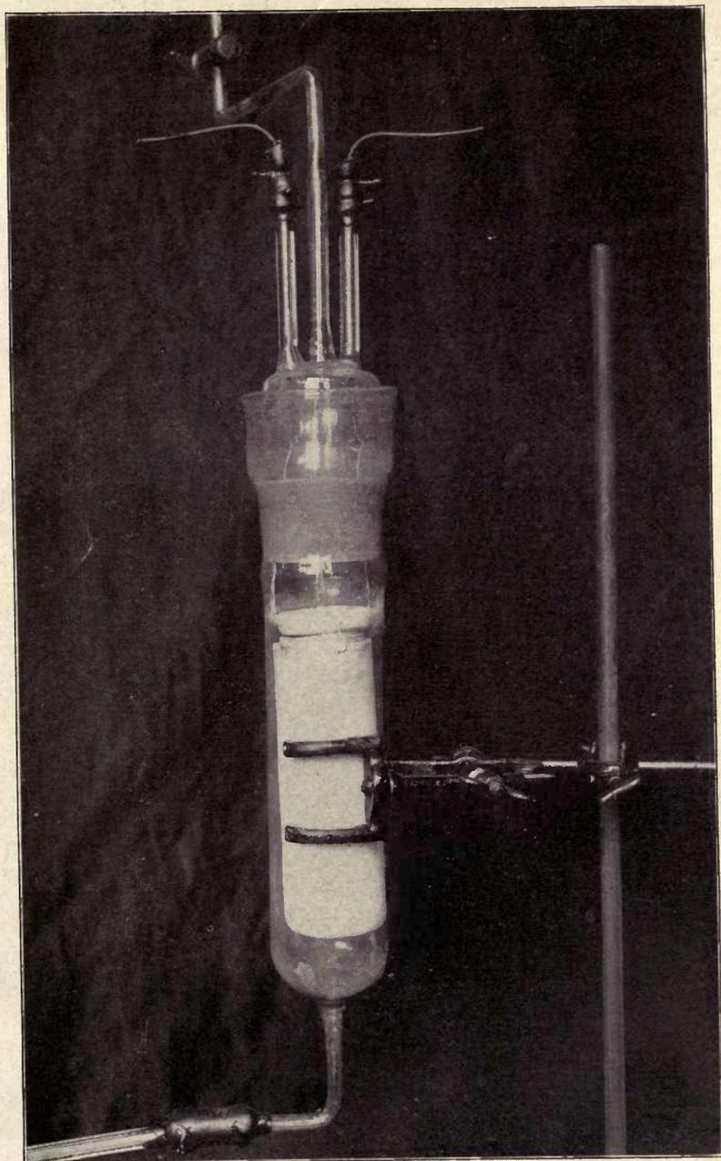
FIG. 6. APPARATUS FOR MEASURING AND ANALYSING THE DISSOLVED GASES
