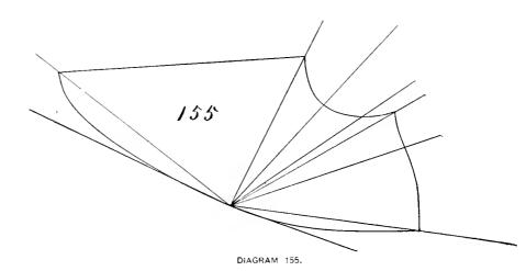
paper large enough, and then mark around the half vamp as got from the working standard. Call it diagram 154, after which select the point easiest to work from as centre of radiating lines. Draw lines sufficient to break all curves. Too many lines do no injury, but only serve to make unnecessary work.
