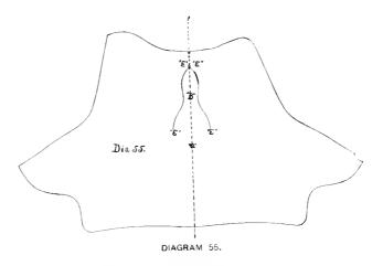
the same lining patterns as well as trimming patterns. This boot, known as the "Climax," is generally cut from heavy stock, such as grain leather. The vamp is used plain.—not beaded. This gives the quarter by drawing a straight line as indicated by dotted line "A." Fold the paper and cut out the quarters, as illustrated in diagram 55. with folded line dotted at "A." While the paper is folded, cut at "B," shown as gore, in diagram 56.
