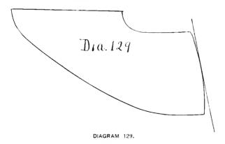
companies now have a wide throat plate—used in closing on with a knife—so as to leave a wide extension of cloth outside of the stitch to prevent it fraying out.
