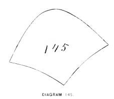
The next will be an ordinary patent tip (diagram 145) cut as usual, while diagram 146 is the same tip cut to save stock and gives the same appearance in the shoe as 145.
