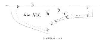
There seems to be no set rule whereby any one can get a perfect blocker the first time, as it largely depends on the stock to be crimped, the manner in which it is to be crimped, whether by machine or by hand, or on a brake. It also depends a good deal on the man who crimps it. It is well to use the rule laid down as far as practical, being governed in many instances by the case in hand. Sometimes repeated trials may be needed.
