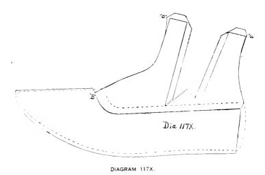
When the front quarter is crimped with the form sharper than the cutting-in form, it is expected that the cutter will see that the crimp curve is made to match that of the cutting in pattern by twisting or straightening the leather.
