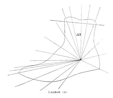
cut off each piece to the outside line and then mark around it on the metal or board with a fine awl. Then cut down to the next size or half size and mark around that, and so on down to the smallest. Of course this destroys your graded paper, but you have the set ready to get out. If you want a duplicate it is easy to mark around your set of metal or board patterns.
