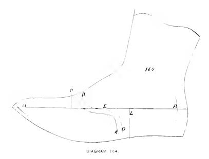
line  $\tau$  on the radii on the long leg. Then I had the one grade on the short end. So I merely run out on line  $\tau$  up to size 7, taking measure of line 2 on the radii and run out from size 4 up to 7. Then I took measure on line 3 and proceeded as before. And so on around the work.
