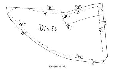
the quarter as got from the standard, "D" is where the front lacing is cut in to throw back the lining without any hand shearing or table work. There should be no cement or glue used on the lining anywhere. There is no use for any.
