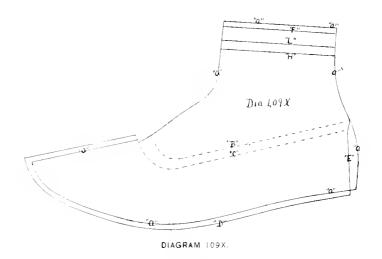
extra roll is caused by closing the quarters on a little lower on the whole lining. It is usual to stitch an inside back stay on the lining down to the vamp lining, leaving lining and stay entirely loose from vamp line to the bottom. This allows the shoe to draw to the last. Nothing will then interfere with the counter, beside it does away with the lump caused by seaming. This shoe is generally vamped through the lining with good results.
