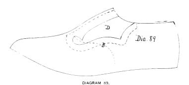
lacing facing cuts very cheaply, and by putting a piece of leather or cloth in the vacancy, "D," (diagram 89) it makes a very nice style. The piece of insertion should be cut as diagram 91 and as dotted line "A" shows the edge of the
