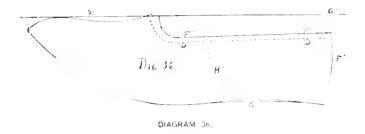
a vamp is generally the best of the skin, too valuable to be used in either tongues or flies. This vamp, if cut whole, is generally put on the shoe by a cylinder machine, and when stretched by bead and presser foot, would be too long. Cut it off at the rear from one-eighth to three-sixteenths inch, as seen at "E." The dotted line "D" "D" rep-
