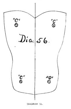
shown on diagram 12. The stab holes, C C C C, diagram 56, are to be pierced so that in fitting they are placed to points E E E E, diagram 55, as the correct spring is so given to gore diagram 56. After getting the outside fitted, close the lining on, and complete as any button boot.
