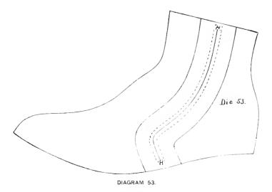
when the linings are ready for the top facings. To get the top facing mark around standard diagram 48 from H to H,
