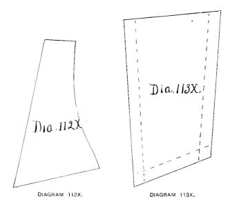
Next lay out the vamp, diagram 111N, and lap on the quarters and gore. Measure each side of the centre of the leg top, for the gore, making it as wide as desired. Then lay off the lap of gore under the quarters, after which cut out all laps and use this standard to get the pieces. Get out the vamp, following with the back quarter and gore, as seen in diagram 112N and 113N.
