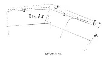
Referring again to diagram 61, see at L and H, where the lines are drawn. This gives the height of or top edge of the lining and the bottom of the facing, obtained by marking round the standard and diagram 61. Recollect that the top of the outside rolls down so the top facing will be cut three-eighths of an incli narrower than it shows drawn round the top of standard diagram 61, one-fourth of an inch for allowance and one-eighth of an inch for allowance to where it is seamed on quarter.
