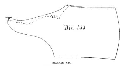
Diagram 133 shows the quarter lining cut from sheep, and at "A" the dotted line shows the line of the opening of the vamp.
