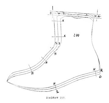
little more than the 5-16, and on EE the increase would be well to be 3-8, although in regular width grading generally holds to 5-16 increase for each width.
