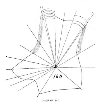
ard. Then get out the largest standard from the largest last, varying in leg as deemed best, after which get the pieces of the largest size and smallest size and grade between with the proportional dividers, as this is the only method of obtaining a proper result. After a set of infants' has been graded do not allow a file put on them for trueing up, for fear of losing the small curves necessary to bring out a small shoe.
