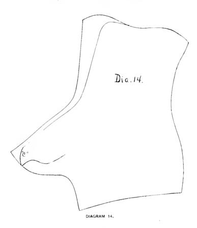
as well as to accomplish a purpose in closing the toe of the lining. When cutting a pattern for a very cheap shoe, it will be well to round the front end of the small quarter clear down to the place where it meets the lower end of the button fly. See diagram 14, "C." This would save stock and take the thickness out from under the lower end of the button fly and yamp, as shown at "C," diagram 14.
