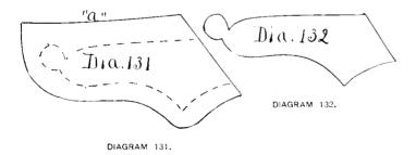
gore, instead of simply drawing hard across the ankle, would draw from instep to heel, an easier fitting shoe could be obtained, beside the leg would be gently forced back, and the heel would not get so far forward. The wrinkles which show so badly just above the vamp at the back would not be there. Diagram 132 shows a pattern used to mark the gore so as to fit correctly.
