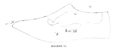
of the last to allow the gore to draw sufficiently on the foot, the laster may draw it down some in the shank, but not too much. Some foremen think it best in making any gored shoe to stitch in one or two pieces of drill or webbing from one side of the gore to the other so as to prevent the strain in lasting coming wholly on the gore. When the shoe comes off the last trim out the pieces with hand shears.
