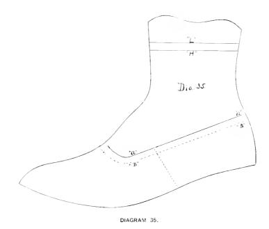
Decide the back of vamp at "A," diagram 35, and draw vamp line "A," "A," allowing the usual distance for lap of quarter. Then draw dotted line "B," "B." Cut through on both lines and take out the piece representing the lap.
