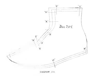
grading is illustrated so plainly in diagram 203 as to preclude the necessity of further explanation.
