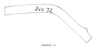
in the full pattern, and then the surplus stock instead of being on the floor, where the table girl has cut it off, is in the skin to be cut into something else. Diagram 72 shows the facing cut so as to be plain edge. If fold is wanted simply add it, and then fold the edge before putting the facing on the quarter.
