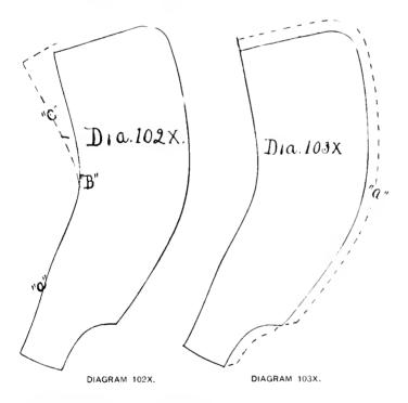
fly as laid off by the eye, generally from about half the width of the leg at the top.
