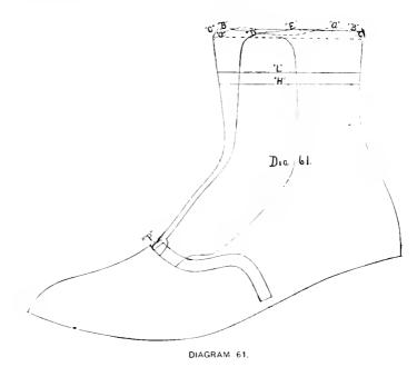
Roll the top from nothing at the corner of the small quarter at D, diagram 61, until it gradually turns about three-sixteens of an inch at E, (diagrams 61 and 62), and then make an even roll until reaching the button fly at "A," diagram 61, gradually running to an even bead at B, as shown in diagram 62.
