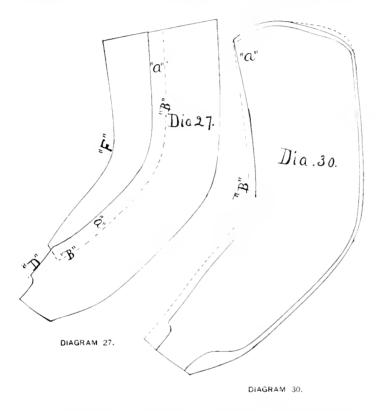
sheep. This cloth "snipe" is closed on to the leather at seam "A," dotted line "B" showing the lap, and, being
