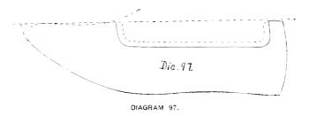
car, where the eyelet holes are, will not admit of roll. Their shape precludes such a result. The standard, diagram 96, is got as usual from the last, after which lay out vamp line and lap; then the tongue and quarter. The back of the tongue must not be too far to the rear, or the shoe will be difficult to get on the foot. The outline of the vamp is shown on diagram 97.
