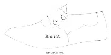
Diagram 102 is a "Southern button." It is about the same fitting as the "Southern tie," except the shoe requiring two quarters, as one must be long enough to fold so as to make the button fly, and the other is short, only taking the buttons. It being a circular vamp makes it cut cheaper.
