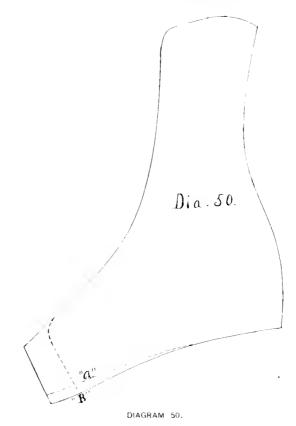
One piece of pattern will do for both sides of the linings for the shoe, as one is cut without the hole, and the
