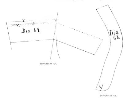
shows bottom of top facing. The dotted line B shows the curve top of standard button boot. This lace we will make roll top and also straight top. For the lining, see diagram
