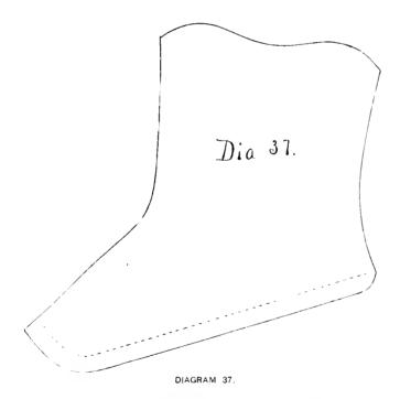
resents the vamp as it will be after the folding at line "F" "F" is taken off. The dotted line "H" shows where the vamp is divided into front vamp and foxing. The foxing in this case is generally closed on, and afterwards stayed with a double needle machine, the same as the front and back of the quarters. If desired, the vamp can be cut so as to lap on the foxings, in which case the shoes can be vamped on a flat bed machine, the same as a circular vamp.
