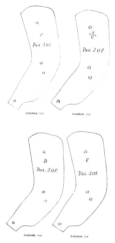
board, and then lay the 4 C, 205, with holes pricked at HH, and KK and having the front, top and bottom directly under the 205, mark through the prick holes. Now your 4 C original is all ready to get the corresponding curve of back on each width.
