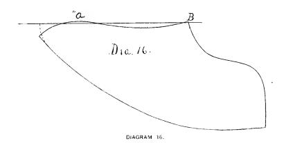
Fold the paper at line "A"-"B," and cut out the half vamp. This half vamp, if exactly duplicated in another half, will make a whole vamp, as shown in diagram 17.
