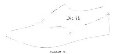
Next lay off the vamp line. Then, allowing lap, lay off the front of the quarter. If a foxed shoe is desired lay off the top of the foxing, then, allowing lap, lay off the bottom of the quarter. It seems advisable to end a foxing, if possible, at the top of the back of the shoe as shown in diagram 75, "C," to prevent a lump, which is always caused by ending it, as seen at "B," in diagram 76.
