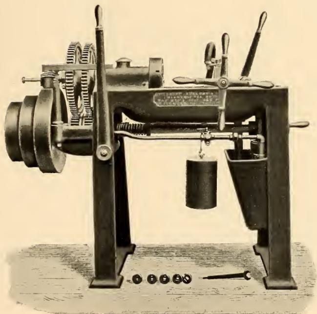
$\frac{3}{4}$ " BOLT AND NUT-SCREWING MACHINE.
