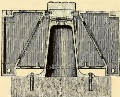
wheels that bear on the circular track and take the tip of the table when the load is not balanced. The pivot centre itself consists first of a conical post with a broad base, for bolting securely to a large capstone upon a suitable foundation.
