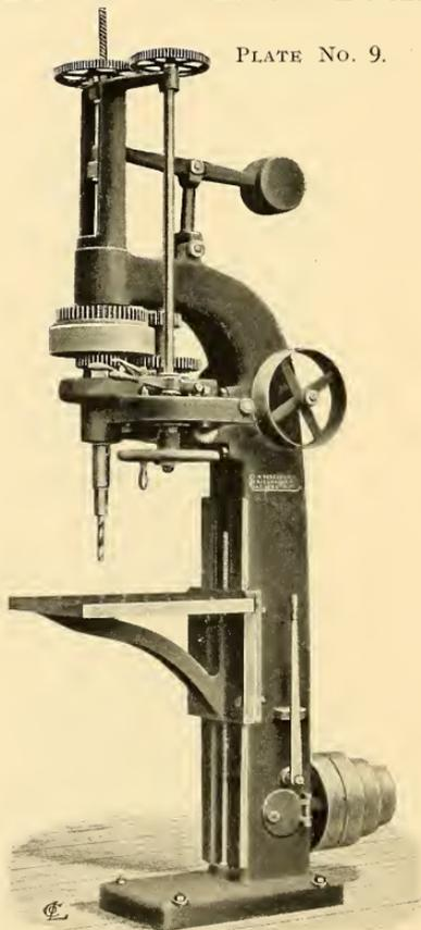
36" VERTICAL DRILLING MACHINE—WITH RECTANGULAR TABLE.
