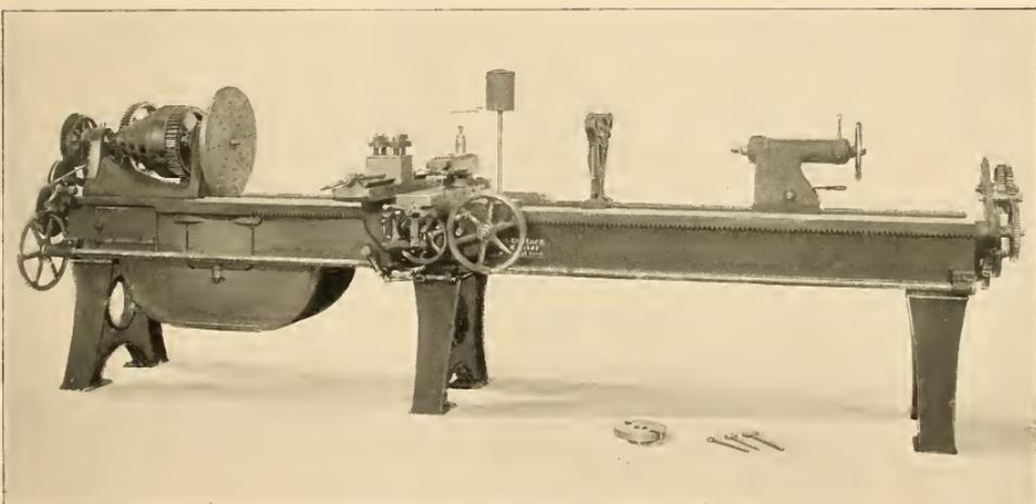
20' GAP LATHE.—GAP CLOSED.
