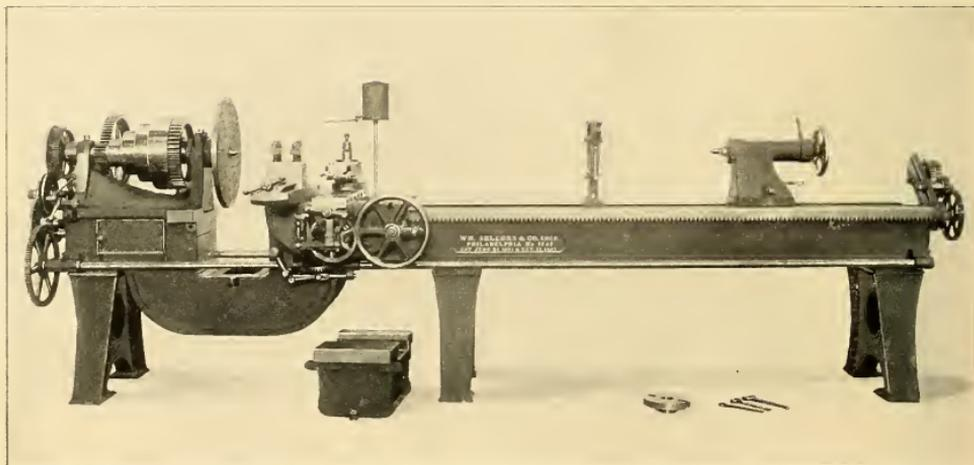
20" GAP LATHE.—GAP OPEN.
