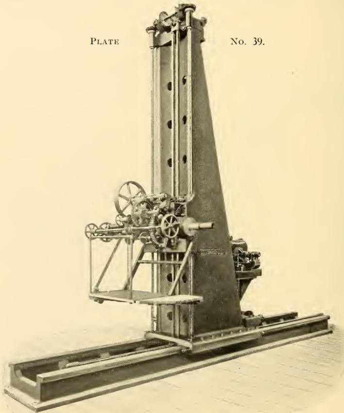
FLOOR-BORING MACHINE ON INDEPENDENT BED.
