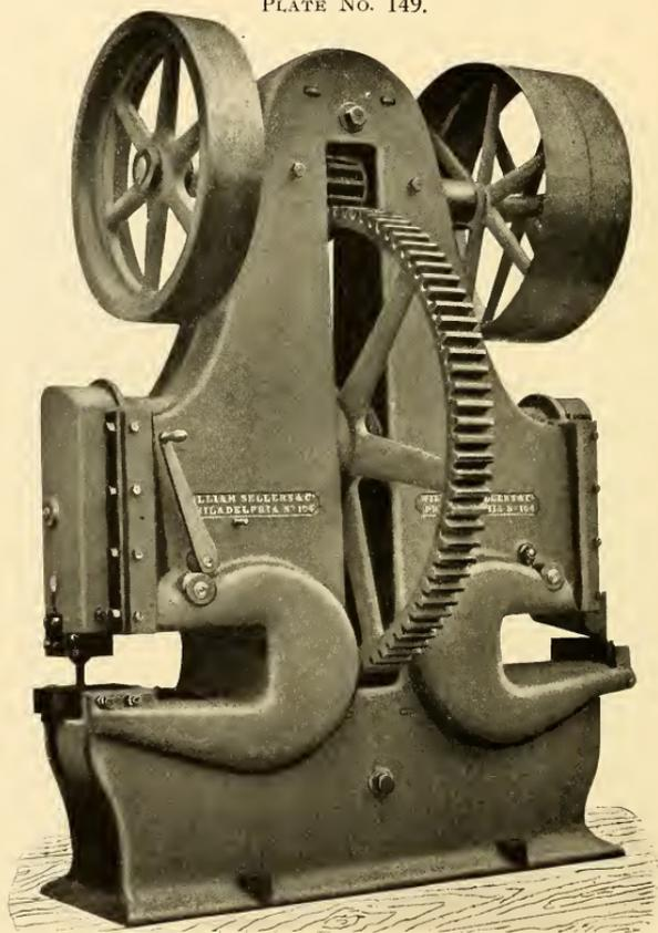
PUNCHING AND SHEARING MACHINE COMBINED.
