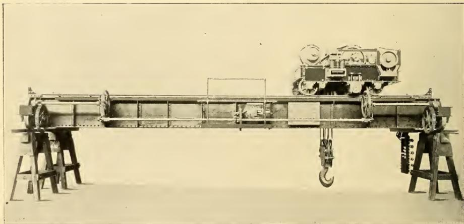
20-TON TRAVELLING CRANE.—FOR RIVETER TOWER.
