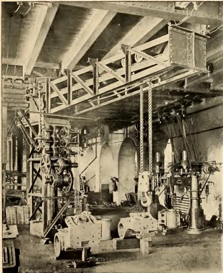
6-TON ELECTRIC COLUMN JIB-CRANE.
