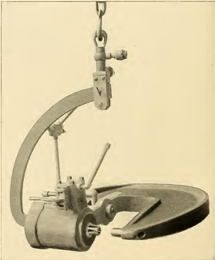
DIRECT-ACTING PORTABLE HYDRAULIC RIVETER.
