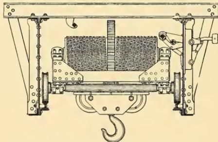
SECTION THROUGH BRIDGE WITH TROLLEY
