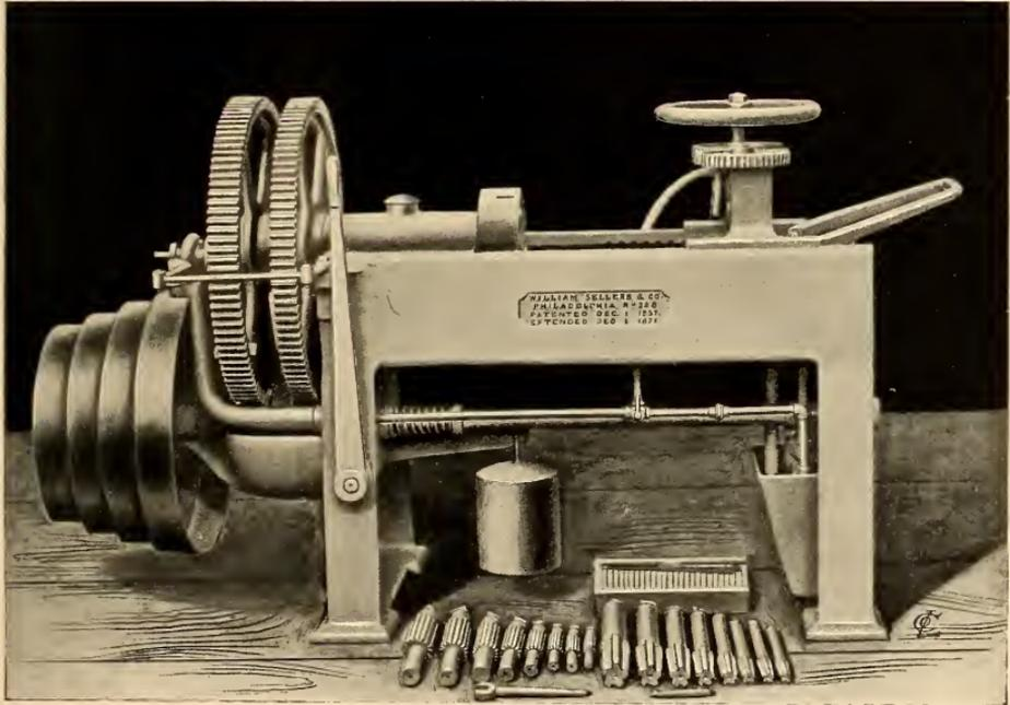
$2\frac{1}{2}$ " BOLT AND NUT-SCREWING MACHINE.
