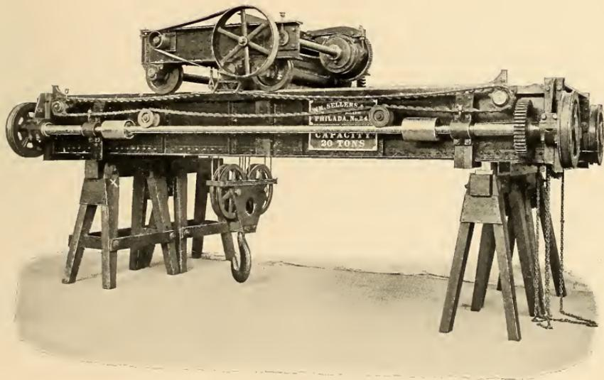
20-TON TRAVELLING CRANE.—FOR USE OVER A RIVETING MACHINE.
