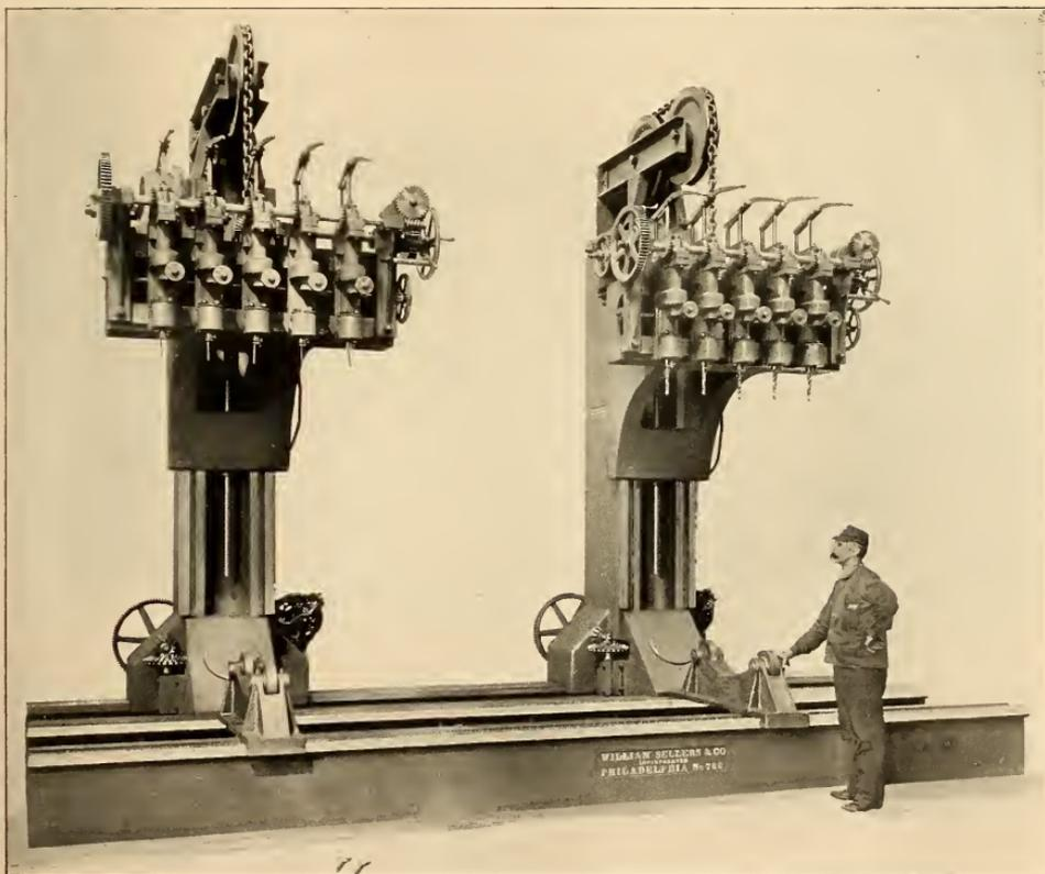
**TEN-SPINDLE BOILER-SHELL DRILLING MACHINE.**
