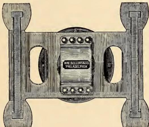
simply because those particular tables were greatly overloaded. Indeed, it is a remarkable fact, and one which speaks well for the materials used, that they have stood at all under the loads given them. Cast-iron tables can be made to carry any required weight, but they must be made deeper and heavier as the load is increased.
