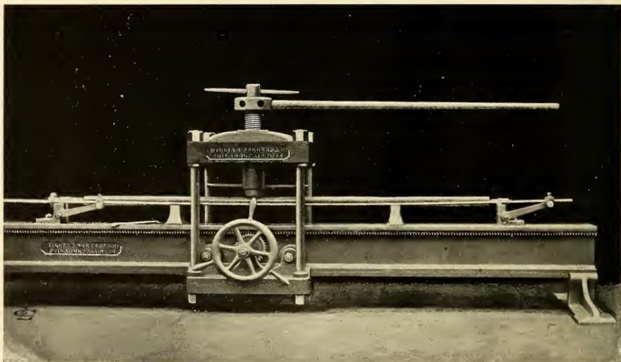
HAND STRAIGHTENING MACHINE.—FOR SHAFTS.
