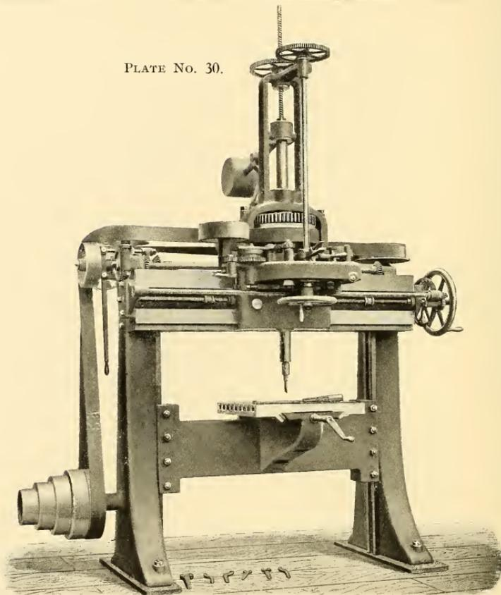
TRAVERSE-DRILL WITH COTTER DRILLING ATTACHMENT.
