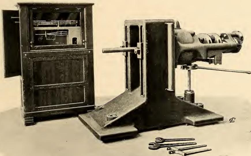
30,000-LB. DYNAMOMETER AND SCALE-CASE.
