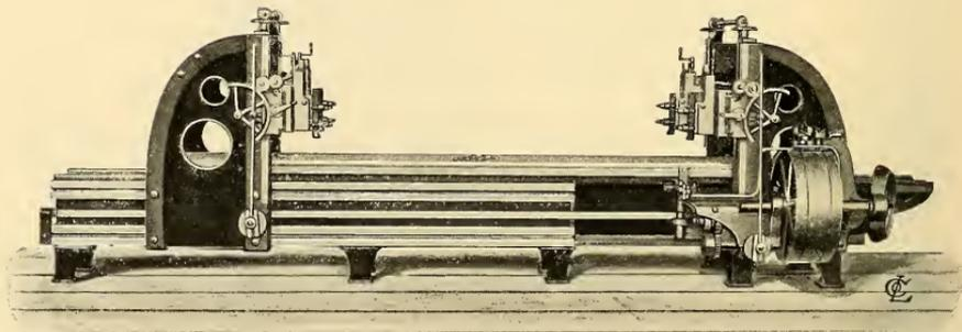
36" ROD PLANER—TO PLANE RODS FROM 3 FEET TO 12 FEET LONG.
