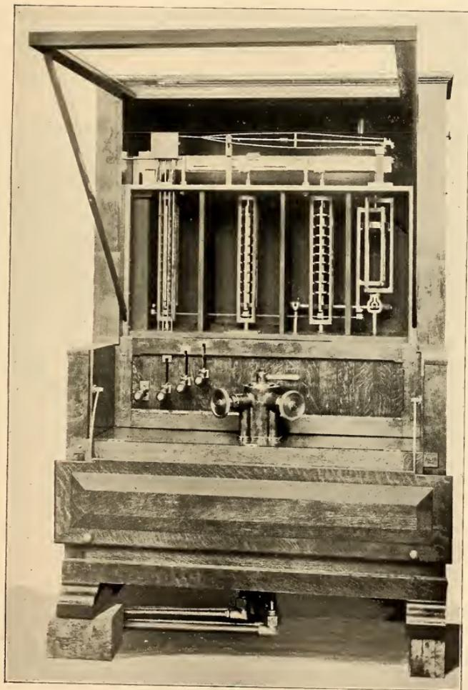
HYDRAULIC SCALE FOR EMERY TESTING MACHINES.
