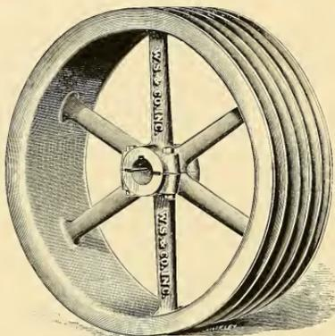
the best of their kind. The transmission wheels should be of *iron*, and have turned grooves of sizes and shapes that have been proved by long experience to be best for the purpose. They should be properly balanced, the various grooves should be so accurately turned to the same pitch diameter, that all of the ropes, or the various wraps of the same rope, may travel at the same velocity, and they should be so fitted and attached to the shaft that the grooves will "run true" and without vibration.
