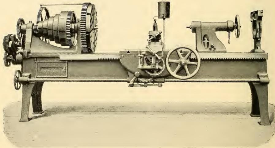
26" LATHE.—TRIPLE-GEARED, TURNING AND SCREW-CUTTING FEEDS.
