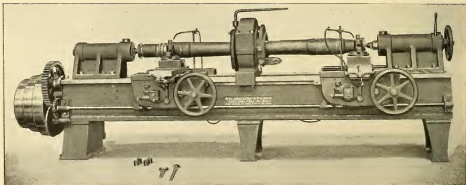
20" DOUBLE AXLE LATHE—WITH CENTRAL DRIVING HEAD.
