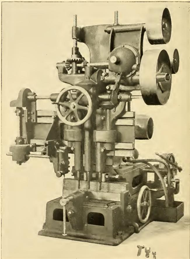
THREE-SPINDLE DRILLING MACHINE.
