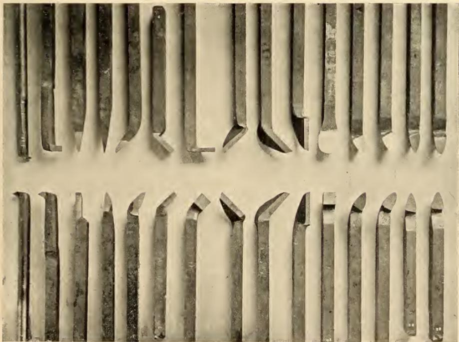
EXAMPLES OF LATHE TOOLS FINISHED TO SHAPE BY THE
