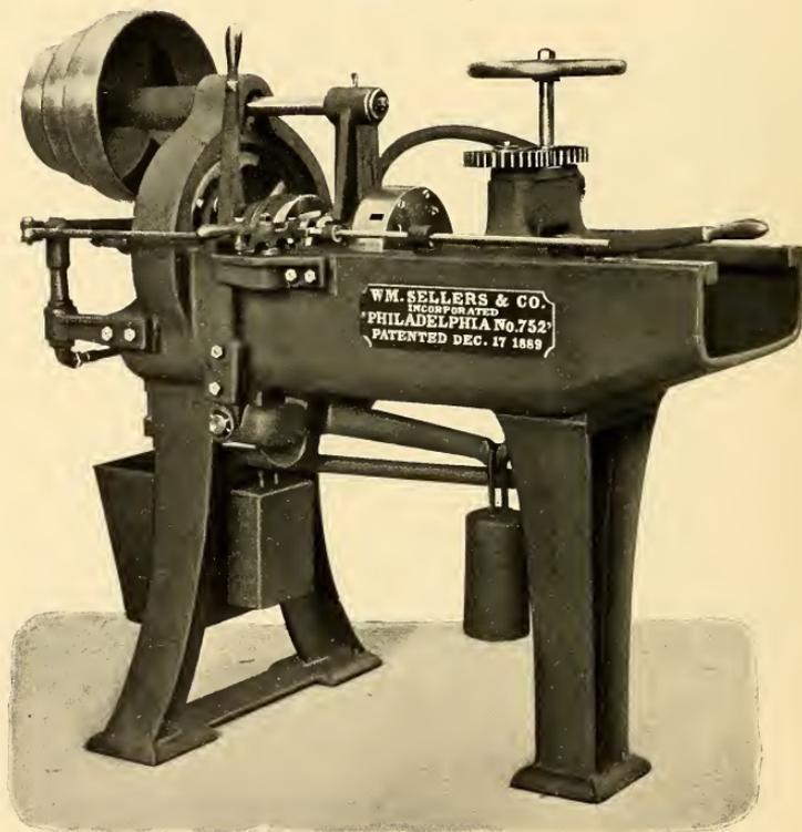
1½" PATENT BOLT AND NUT-SCREWING MACHINE.
