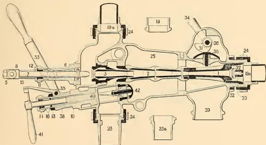
When it is especially desired to use supply water at a high temperature, a new form of this injector (Class K.) can be supplied, for which the limiting temperature is 145 degrees at 120 pounds of steam, and 140 degrees at 180 pounds pressure. The capacity of these injectors is given in the following table, which is based upon recent improvements that have largely increased the delivery at 180 and 200 pounds steam pressure.
