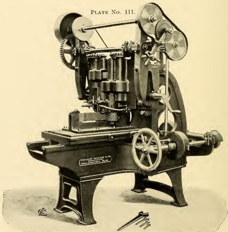
TWO-SPINDLE VERTICAL MILLING MACHINE—FOR TEST SPECIMENS.
