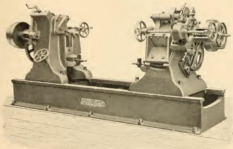
WHEEL-QUARTERING MACHINE FOR LOCOMOTIVE DRIVING-
