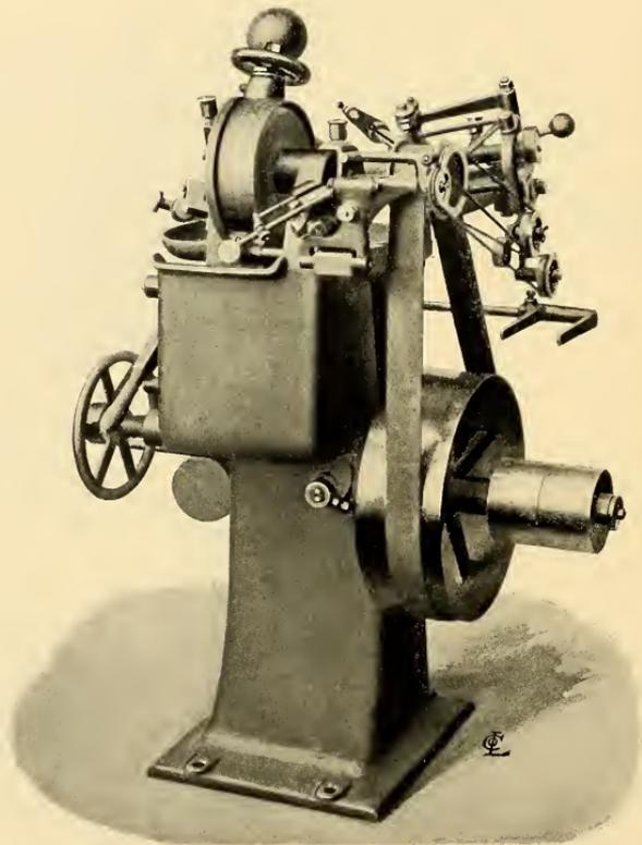
REAR VIEW OF PATENT DRILL-GRINDING MACHINE.
