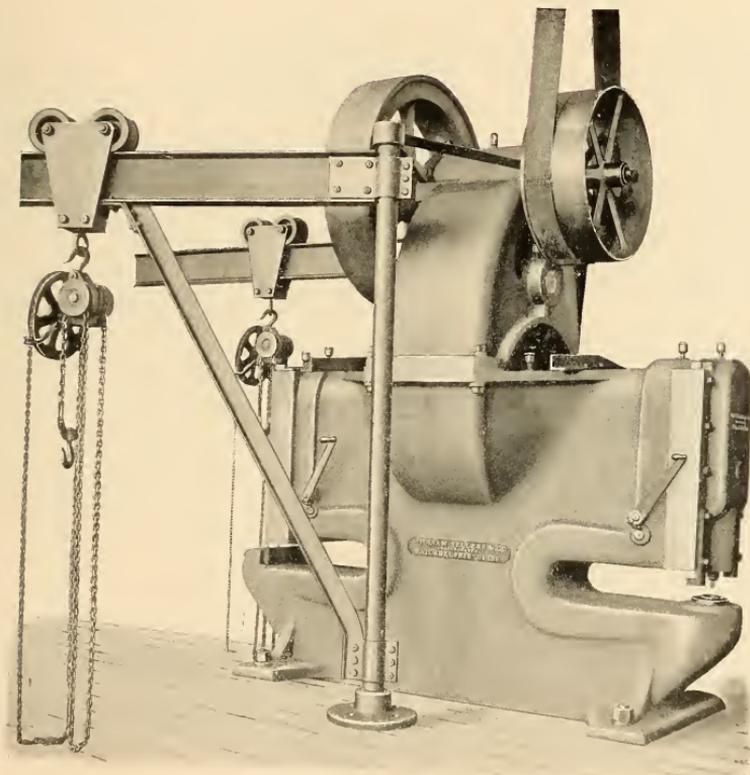
PUNCHING AND SHEARING MACHINE COMBINED—30" OVERREACH.
