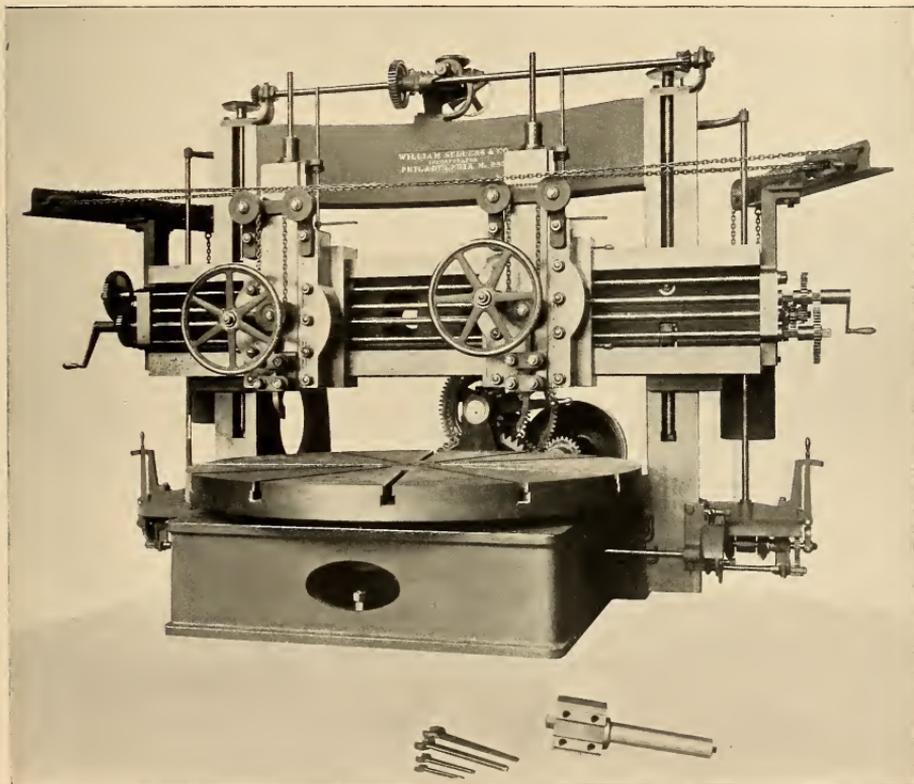
7-FOOT BORING AND TURNING MILL,—WITH TWO SADDLES.
