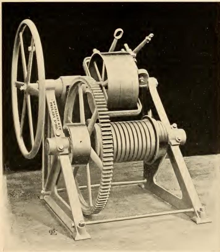
SPUR-GEARED HOISTING CRAB.—WITH WESTON RETAINING CLUTCH.
