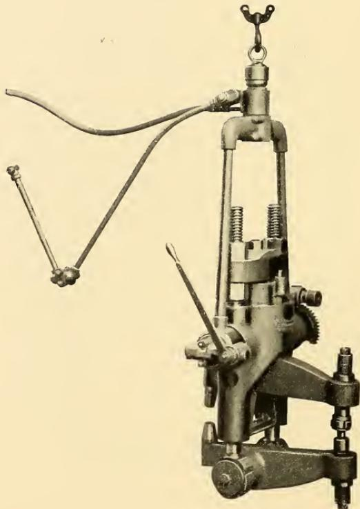
DIRECT ACTING PORTABLE HYDRAULIC RIVETER.
