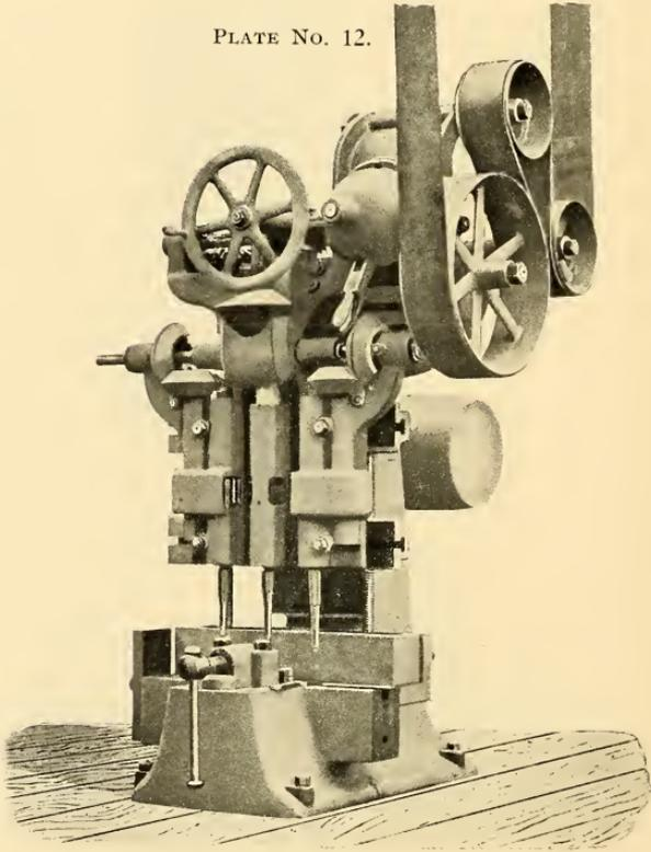
THREE-SPINDLE RAIL DRILLING MACHINE.
