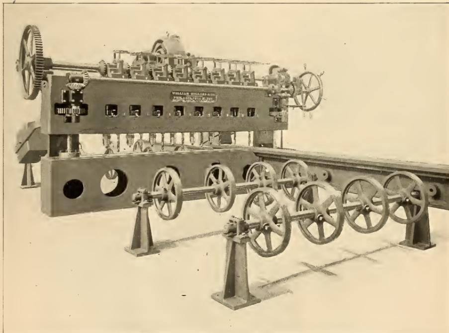
FOURTEEN-SPINDLE DRILLING AND BORING MACHINE.
