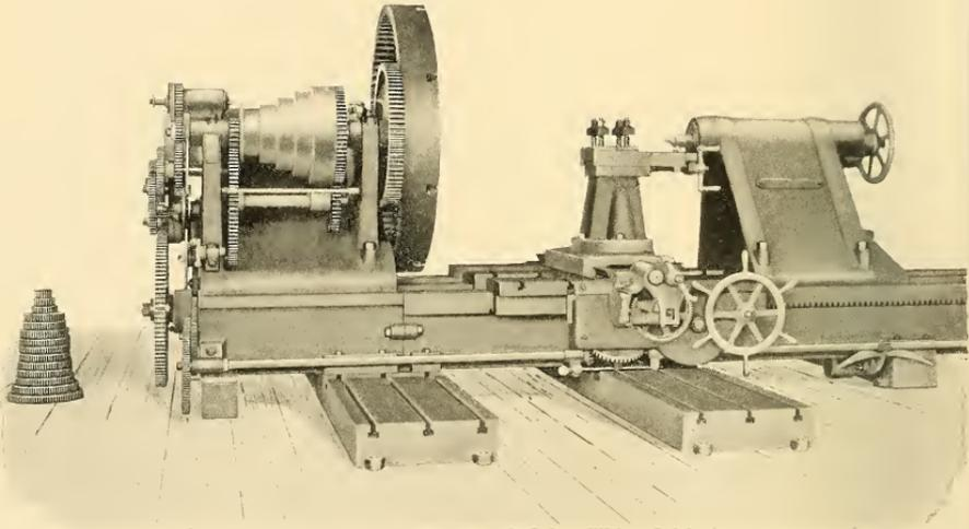
72" SELF-ACTING GAP LATHE.—FOR SCREW-CUTTING AND TURNING.
