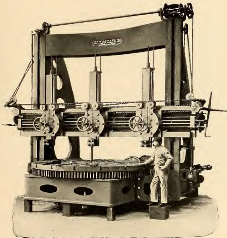
12-FOOT BORING AND TURNING MILL—WITH THREE SADDLES.
