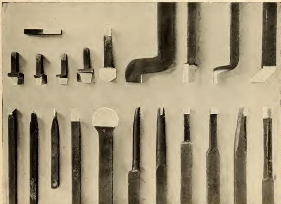
EXAMPLES OF MISCELLANEOUS THREAD, BORING, SLOTTING, AND OTHER
