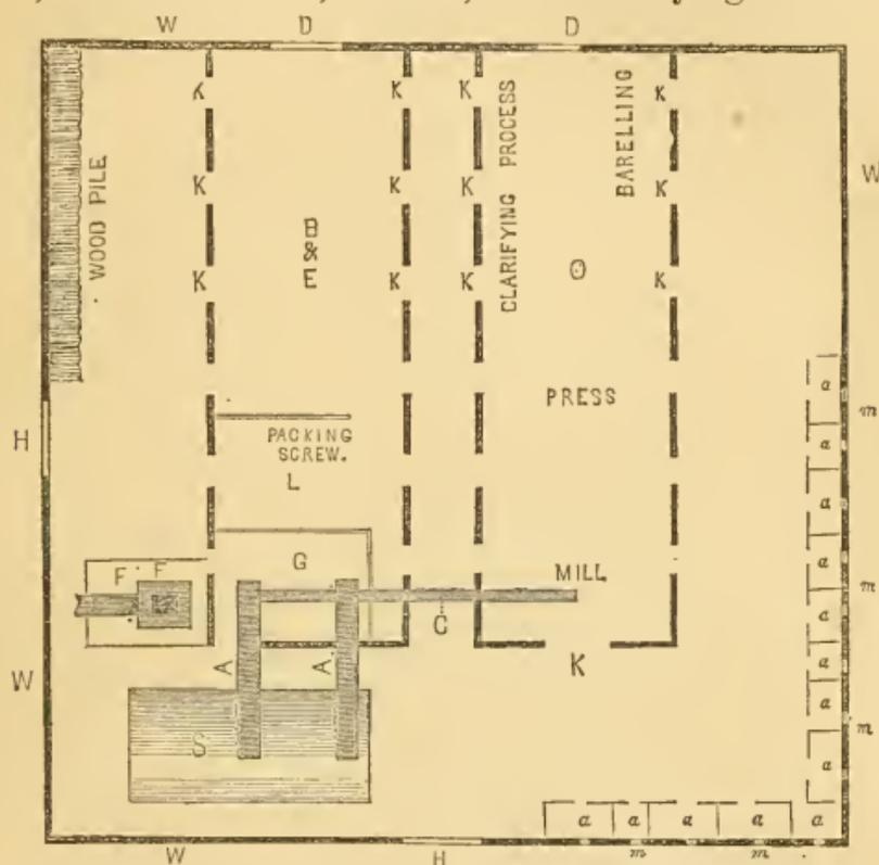
Fig. 20.—PLAN OF COTTON FACTORY AND INCLOSURE.
