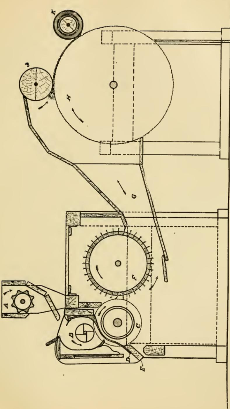
FIG. 74. Section Through Cotton Seed Linter.
