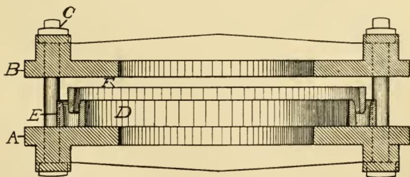
FIG. 102. Mold for Making Hydraulic Packing.
