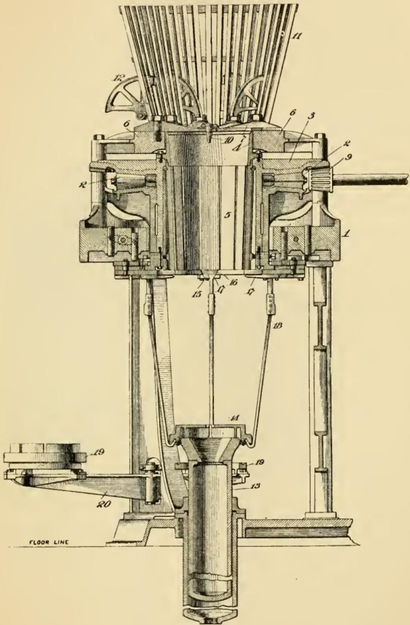
FIG. 35. Ginnery Compress, End Packed Cylindrical Bale.
