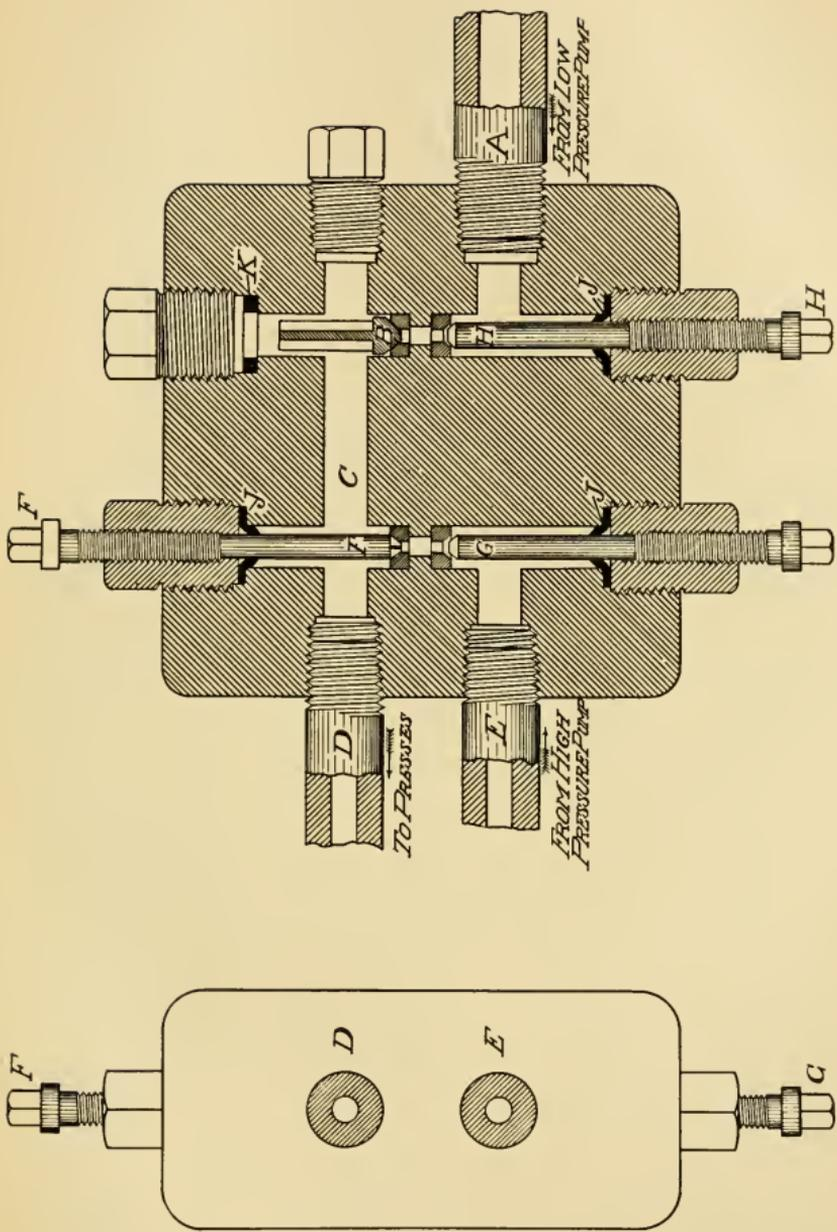
FIG. 107. New Style Automatic Change Valve.
