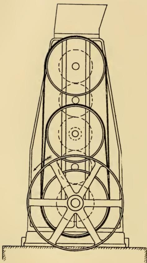
FIG. 86. Diagram Tandem Drive for Five-High Rolls.
