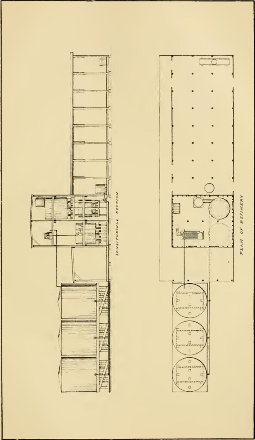
FIG. 113. Plan and Section Cotton Oil Refinery.
