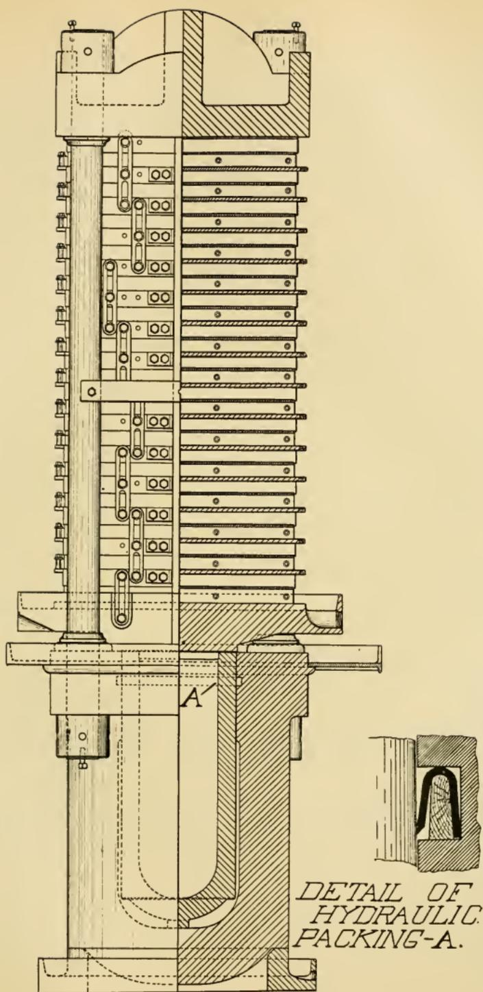
FIG. 101. Oil Press, Showing Hydraulic Packing.
