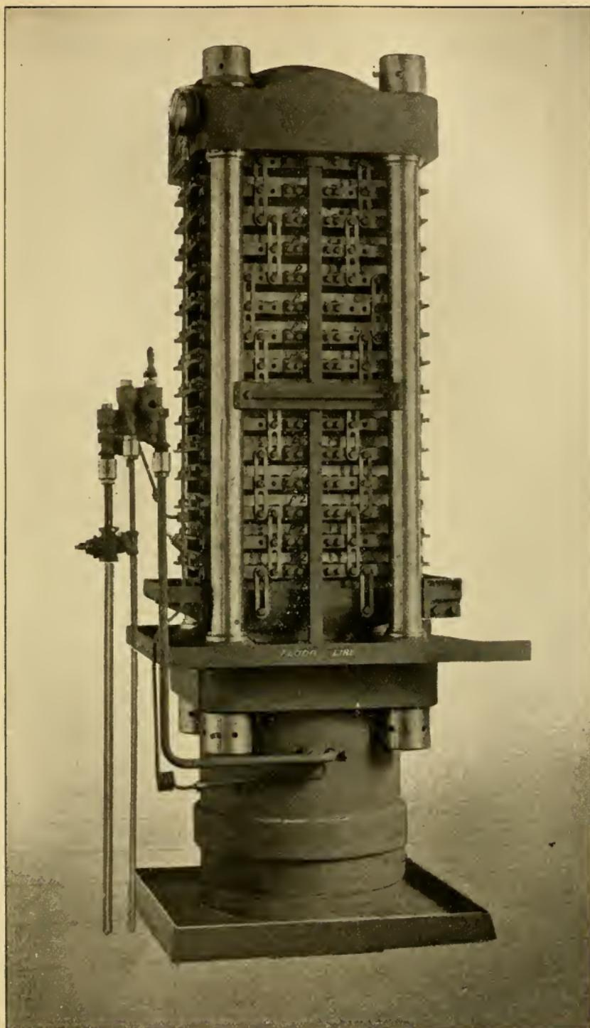
FIG. 99. Oil Press, Showing Valves.
