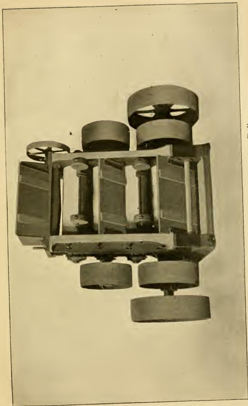
FIG. 87. Four-High Tandem Rolls.
