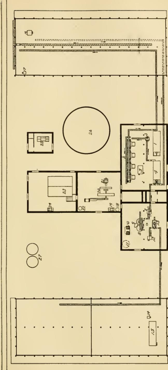
FIG. 67. Arrangement of Machinery, 40-Ton Oil Mill, 1901.
