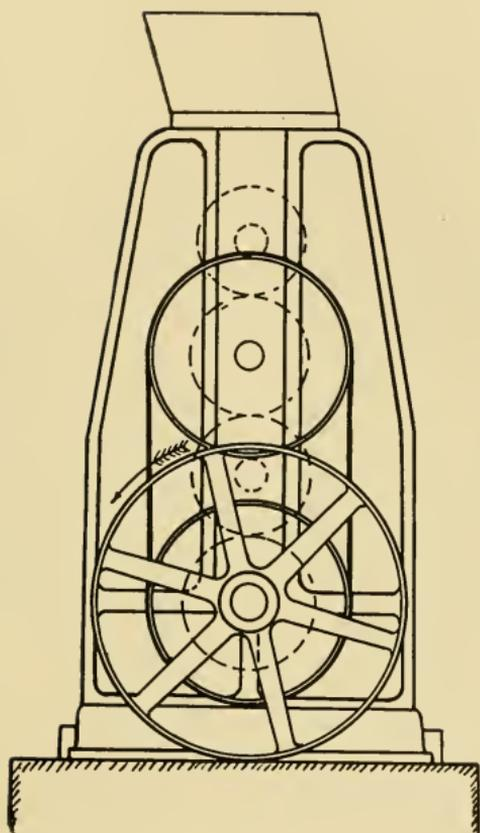
FIG. 85. Diagram Tandem Drive for Four-High Rolls.
