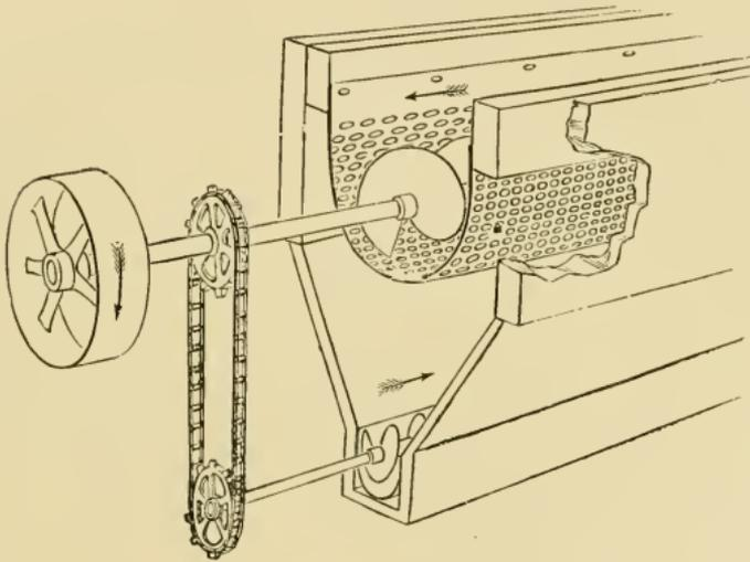
FIG. 82. Separating Conveyor.
