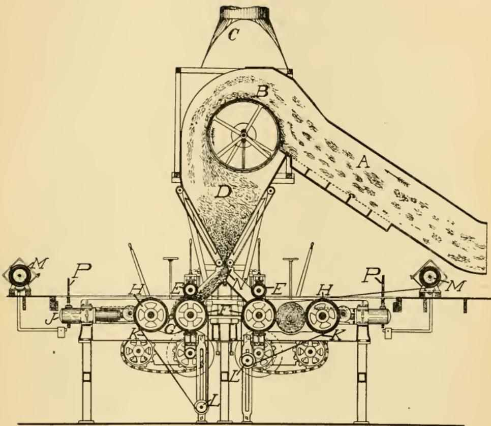
FIG. 34. Ginnery Compress, Cylindrical Lap Bale.
