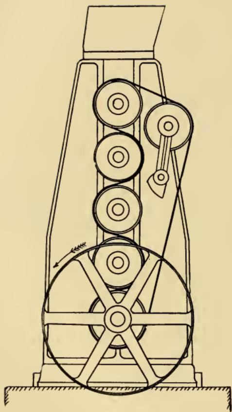
FIG. 83. Diagram Serpentine Drive for Rolls.
