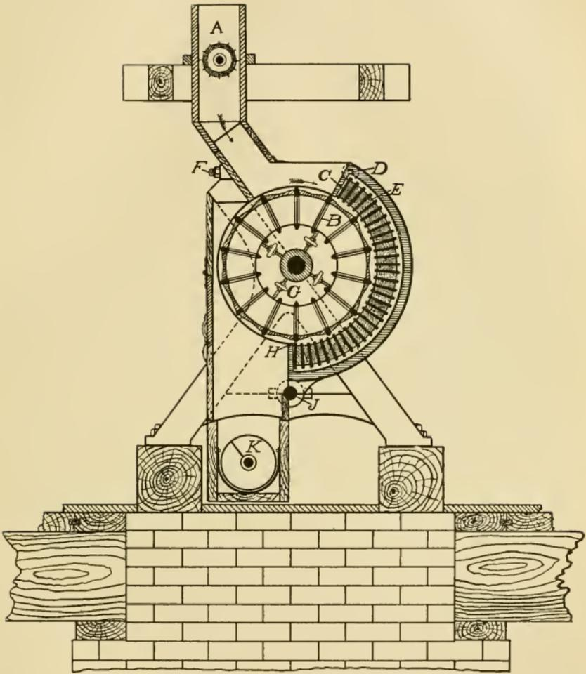
FIG. 80. Section Through Huller.
