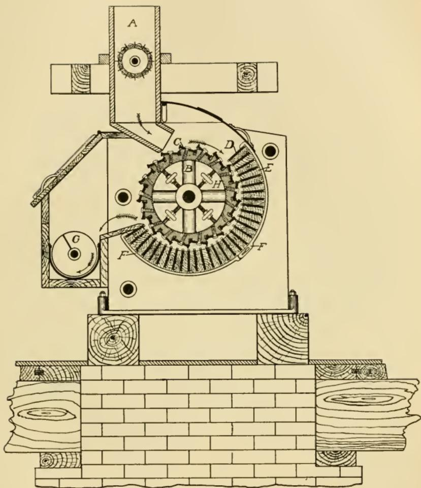
FIG. 78. Section Through Huller.
