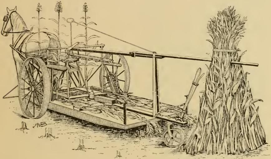
FIG. 9.—Rear view of two-row corn harvester.
