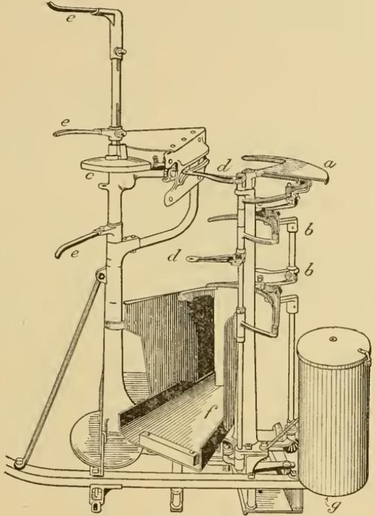
FIG. 14.—Binder attachment: *a*, needle; *bb*, packers; *c*, knotter cam; *dd*, compressor hook; *eee*, discharge arms; *f*, Butt table or butt shoe; *g*, twine cam.
