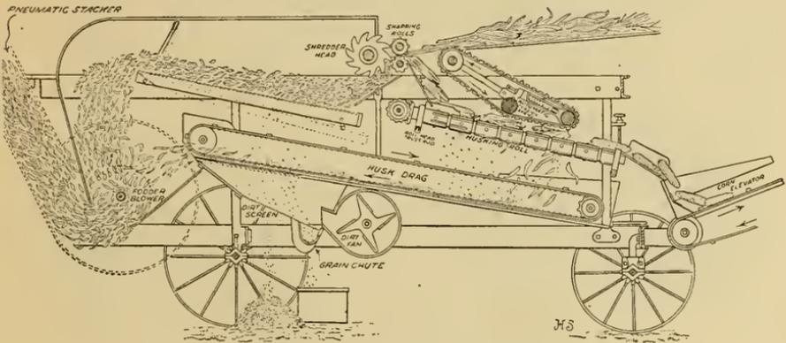
FIG. 22.—Skeleton of husker and shredder.
