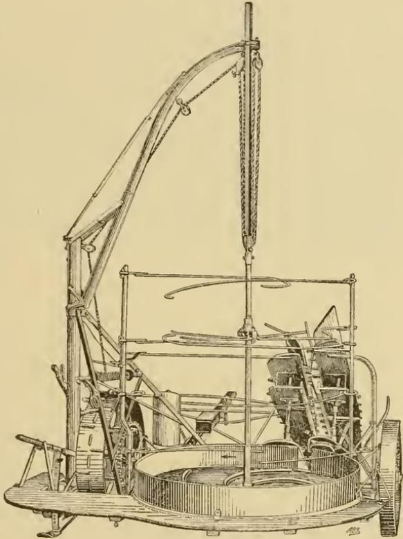
FIG. 17.—Corn harvester and shocker.
