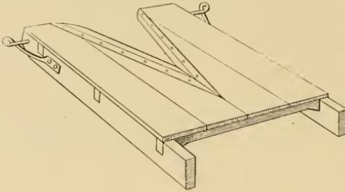
FIG. 4.—One-row sled harvester.
