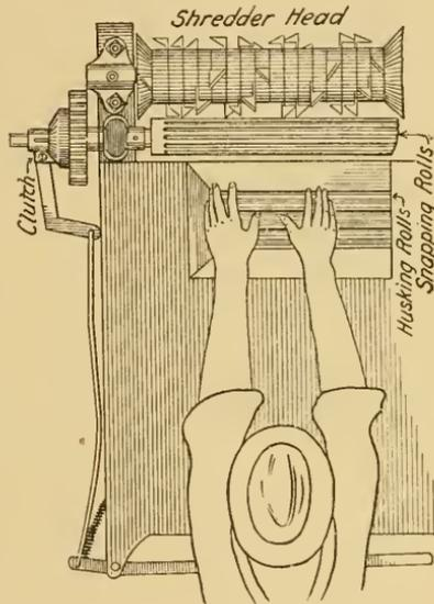
FIG. 24.— Safety device for shredder.
