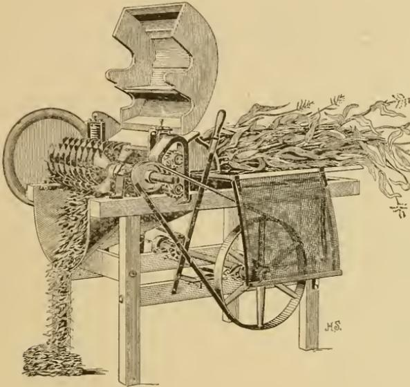
FIG. 21.—Corn shredder.
