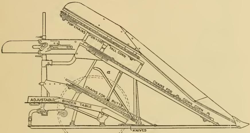
FIG. 12.—Skeleton frame of corn binder, showing chains.
