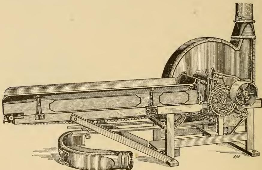
FIG. 20.—Self-feeding ensilage cutter with blower.
