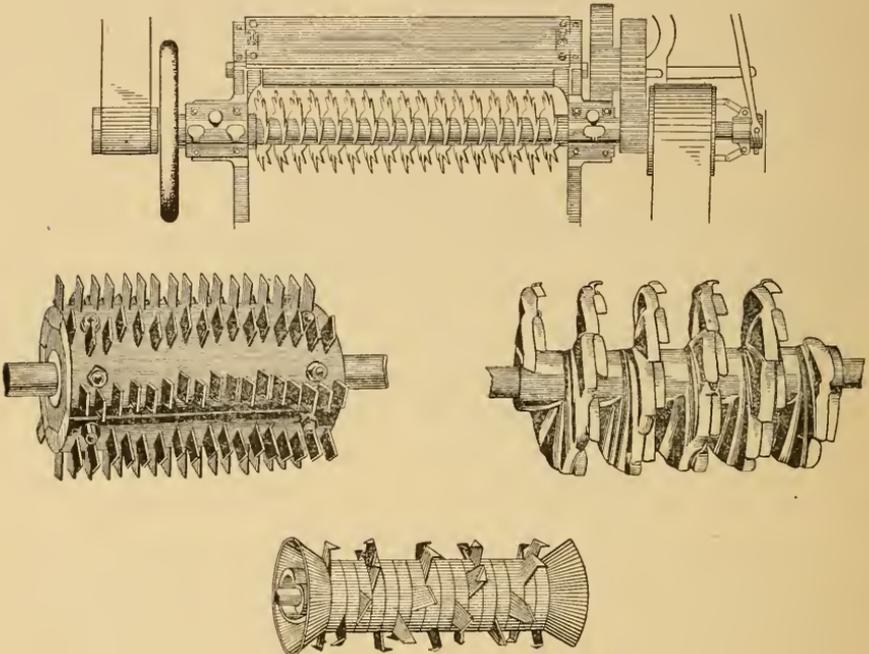
FIG. 23.--Forms of shredder heads.
