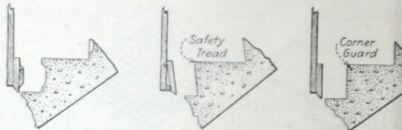
Fig. 39—Detail of different step treads and forms for them.
