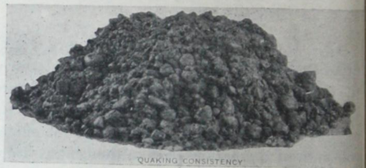
Fig. 7—Three typical consistencies of concrete mixture when poured. A guide for mixing concrete for different kinds of work.
