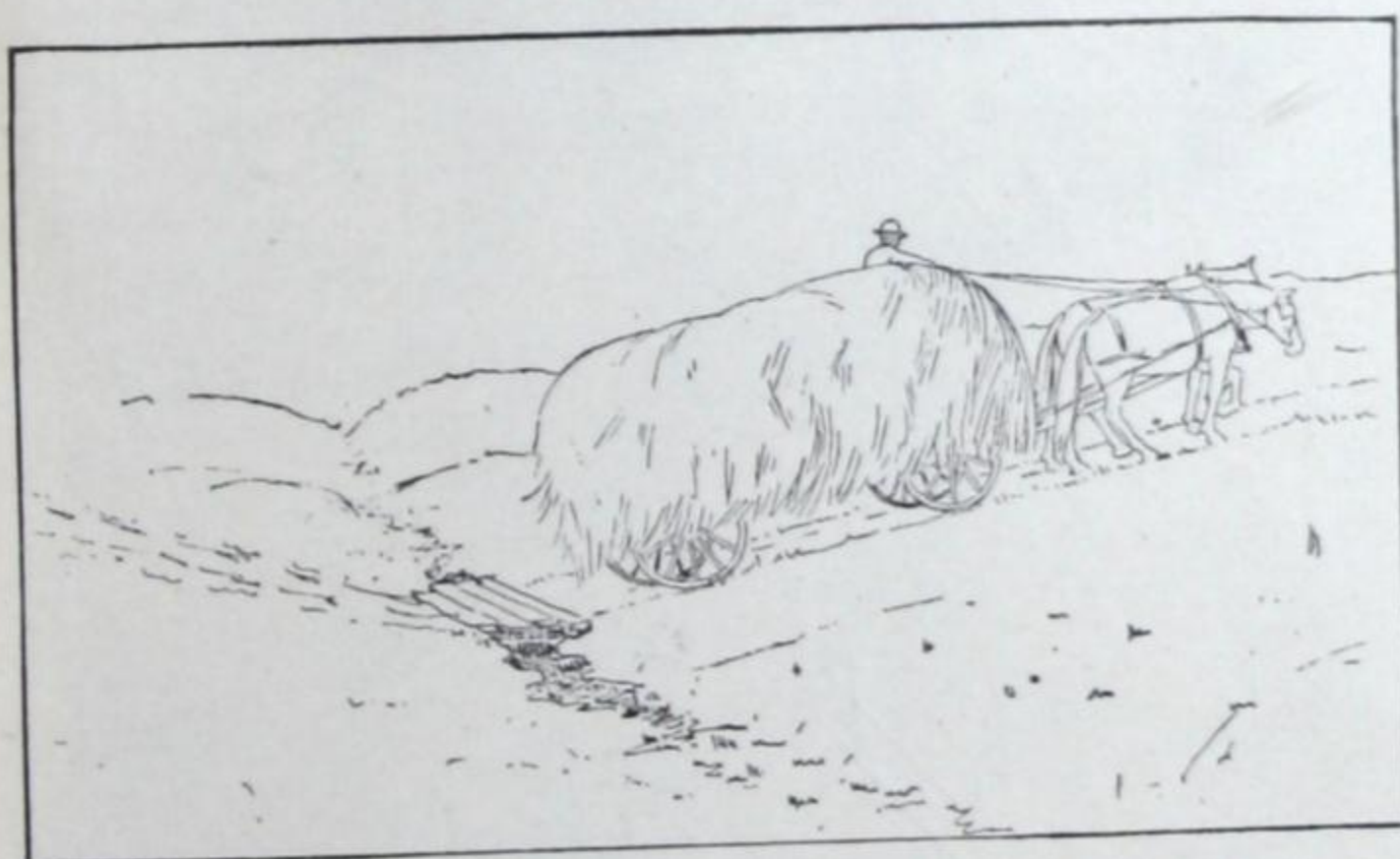
Fig. 195—Heavy grades raise hauling costs. Put in a concrete culvert and fill up road.
