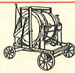
ELLIS Mixing Unit (Powerless-On Truck) Capacity, 3 to 5 Cu. Ft. (Dry)
