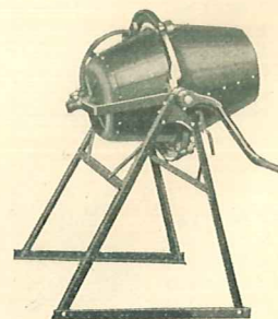
Illustration shows side view of the WIZARD Junior Concrete Mixer in loading and mixing position. Note the long handle for tilting drum—makes turning easy.
