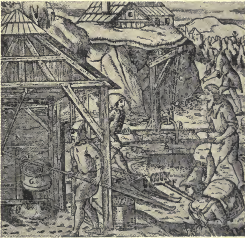
FIG. 10. EARLY SCREENING APPARATUS
